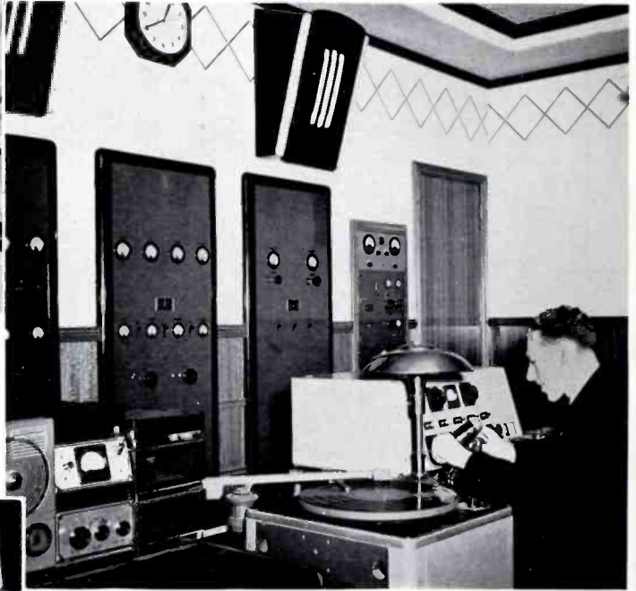
▲ A portion of KFAR's transmitter control. Chief Engr. Stan Bennett at the console. Door to the right gives quick accessibility to RCA 1-G transmitter.
