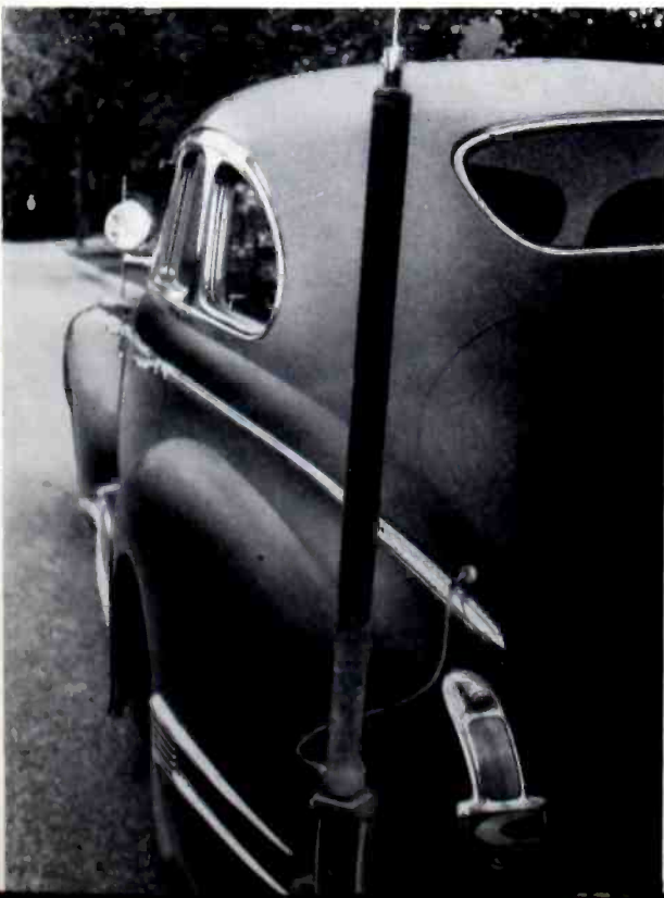
FIG. 3. Closeup of the special car antenna developed for the Wyoming Patrol. The four-foot loading section is shown here. A seven-foot whip (removable) fits in the top of this section.
