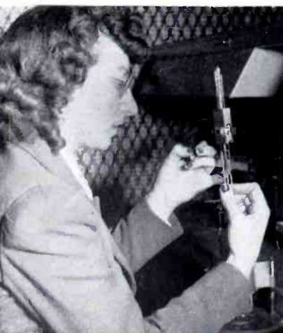
6 The completed rebuilt filament stem with new filament installed.
