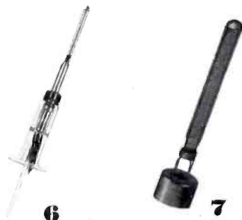
7 The grid assembly is sand-blasted, the grid cap polished, and the grid vacuum fired.
