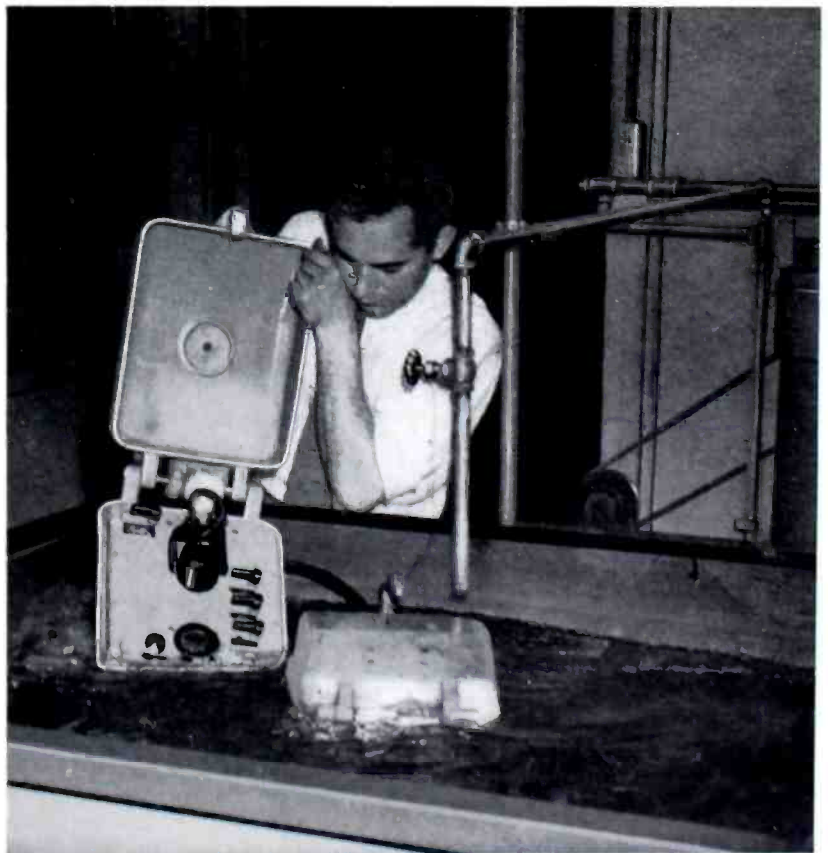
RCA battle announcing equipment being subjected to the submersion test. Equipment of this type must be waterproof and rugged; must operate without failure under the most difficult conditions.
