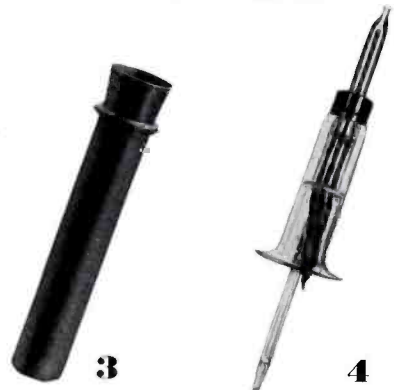
3 Rebuilt anode with new, thick copper cone ready for machining to obtain new feather-edge for glass-to-metal seal.
