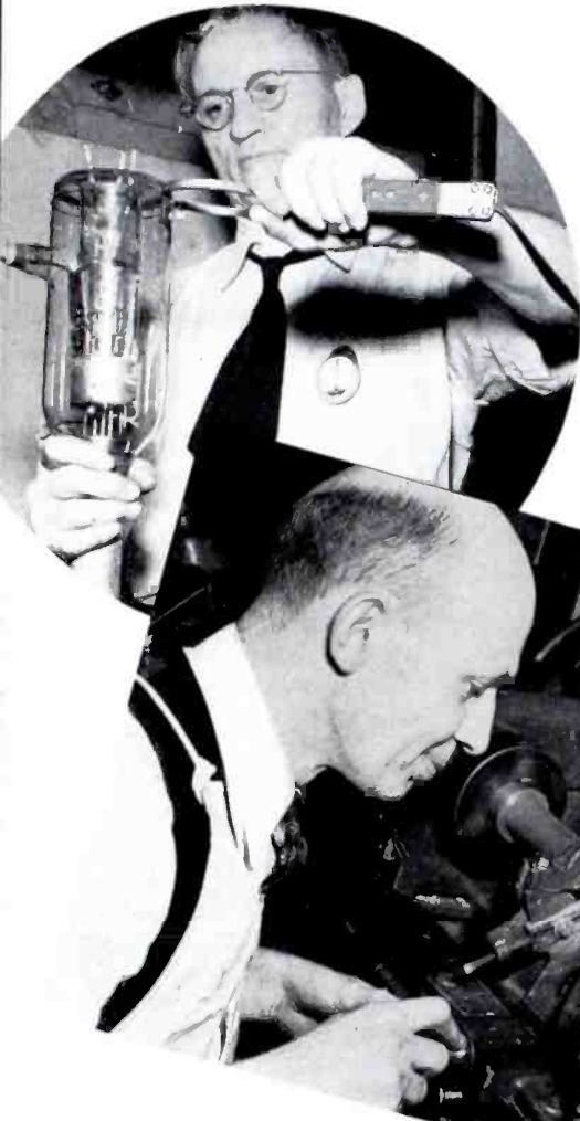
1 The glass envelope is carefully cut open by means of an electrically heated wire and application of a damp cloth.
