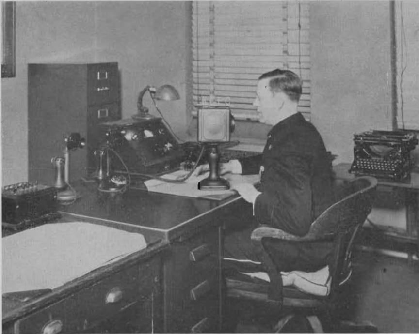
CLOSEUP OF RADIO DISPATCHER'S DESK WITH CONDENSER MICROPHONE AND RADIO TRANSMITTER CONTROL BOX
