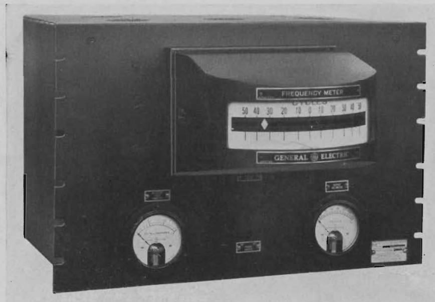
FIGURE 4 METER-POWER SUPPLY UNIT. NOTE LARGE EASY-READING FREQUENCY METER
