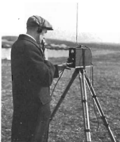
FIGURE 3—COMPLETE "TRANSCIEVER" EQUIPMENT MOUNTED ON TRIPOD FOR FIELD SERVICE.
