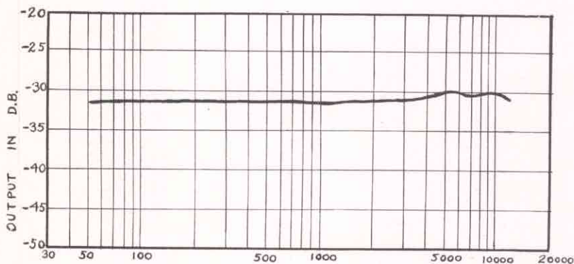
FIG. 7—FREQUENCY IN CYCLES PER SECOND. CURVE SHOWING OUTPUT AT THE 250 OHM LINE OF THE AMPLIFIER FOR CONSTANT SOUND PRESSURE IN FREE SPACE.
