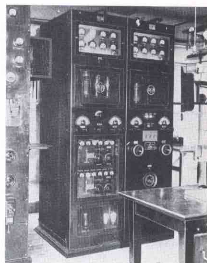
THE NEW RCA 1-C TRANSMITTER AT WBEN.
