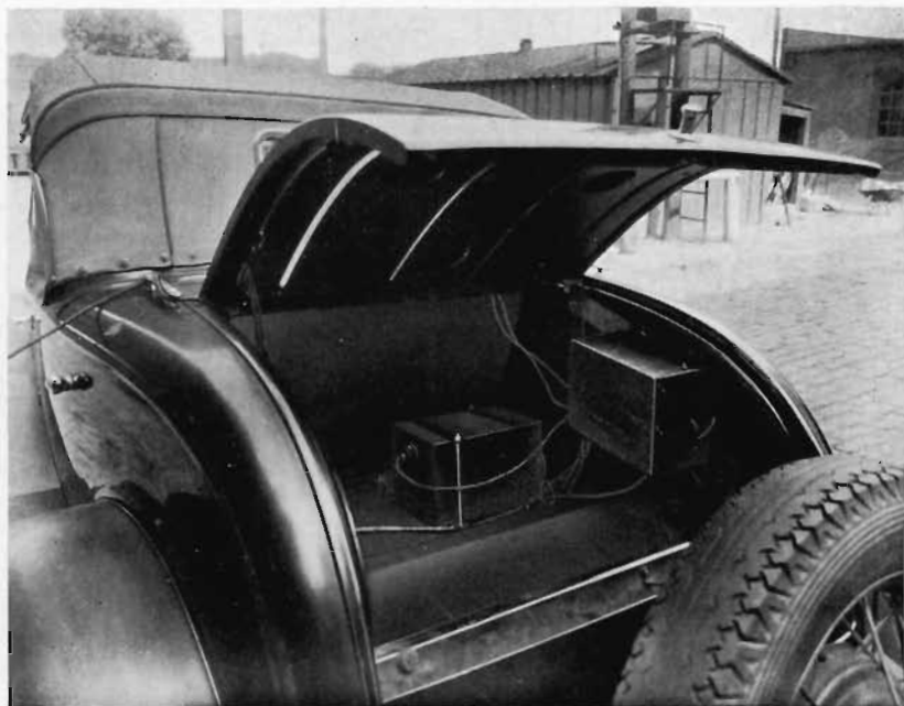
FIGURE 3—TYPICAL INSTALLATION IN POLICE CRUISING CAR, BALTIMORE, MARYLAND
