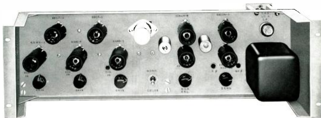
FIG. 1. The automatic light control amplifier is housed on a standard bathtub chassis for mounting in a 3V pedestal, TP-15 Multiplexer pedestal or a cabinet rack.
