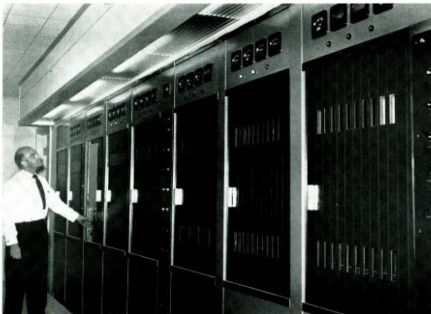
FIG. 17. Transmitter Supervisor, M. A. Robertis, adjusting control on aural position of TT-25AH Transmitter.
