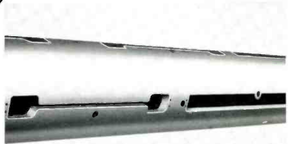
CLOSE-UP OF ANTENNA SHOWING UNIQUE SLOT RADIATOR DESIGN
