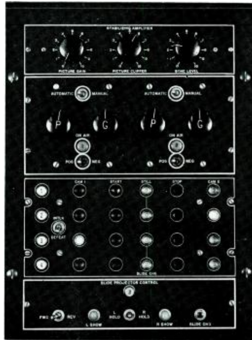
FIG. 5. ALC remote control units (second panel from top) may be mounted in a standard console along with other remote control panels. An adaptor faceplate accommodates two of these units at this position. Manual pedestal and gain controls are also located at this panel for convenience of operation.
