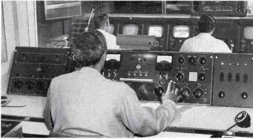
FIG. 9. Audio booth for Studio 2. Note main video switching and control position immediately in front of audio booth. Note BC.6 audio console.
