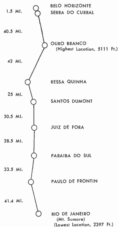
FIG. 2. Simplified diagram showing number of hops and distances covered by the Radio Tupi microwave installation.
