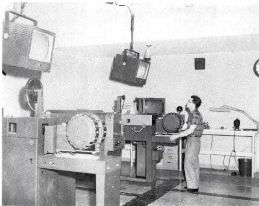
FIG. 12. Film projection room. The operator is standing by the monochrome vidicon equipment. This consists of two TP-6A Film Projectors, a TP-7 Slide Projector, and TP-11 Multiplexer. To the left is RCA 3-V Color Film equipment (also used for monochrome). This consists of TP-6CC Film Projector, a TP-7 Slide Projector, and TP-15 Multiplexer. Ample space has been provided for expansion.
