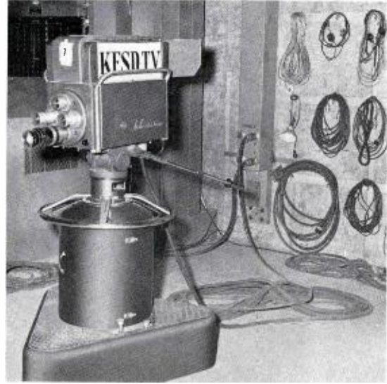
FIG. 5. Camera, intercom, and microphone outlets in Studio 1. To the right are storage hooks for intercom and cable equipment.
