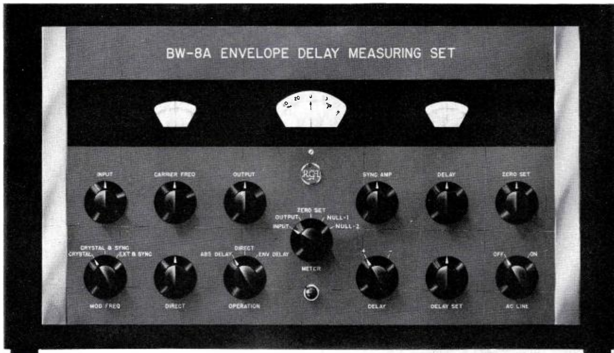
FIG. 1. This is the Envelope Delay Measuring Set, Type BW-8A. All operating controls have been placed on the front panel of this direct reading equipment.
