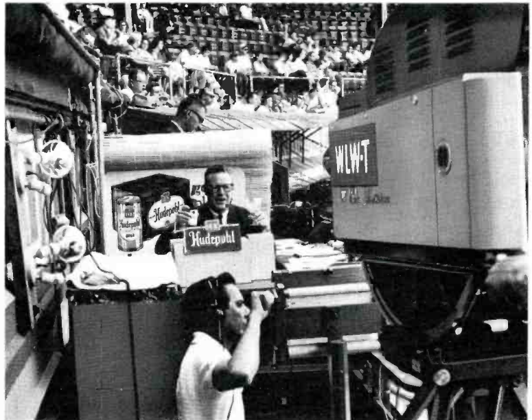
FIG. 4. A miniature set for live commercials is located in the tv booth behind home plate. The color camera is positioned so that it may be easily swung around to pick up the commercials. A portable hand-prompter and two fill-in flood lights complete the equipment complement.
