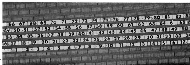
FIG. 1. Close-up of headwheel panel of the RCA TV Tape Recorder showing how video heads apply transverse tracks on tape. Tracks shown here are an artists conception of video information applied to tape. Extreme close-up below shows detail of tracks—note that each scanning track is made up of 18.4 horizontal TV lines.
