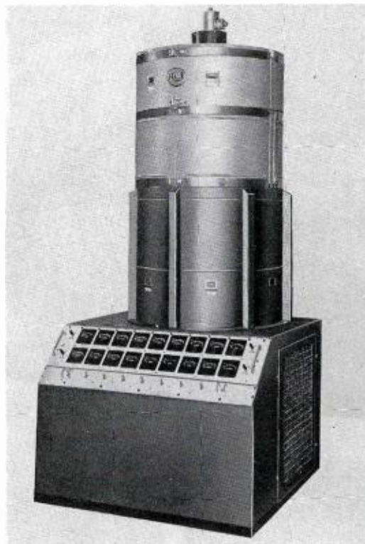
FIG. 8. External view of the TT-25CH amplifier. Note the extensive metering facilities, which indicate all important circuit conditions.
