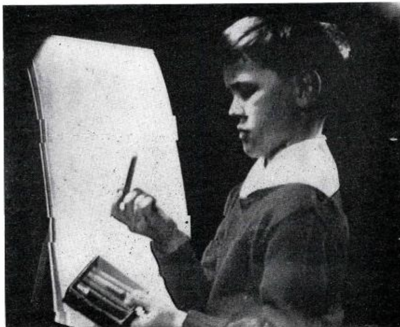
FIG. 2. The displacement of individual heads by an finite amount from exact quadrature appears in the tv picture as a horizontal displacement of "headbands." This is the effect that results—note displacement of vertical lines.
