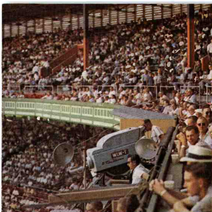
FIG. 1. Located in the tv booth behind home plate, an RCA color camera does double duty—picking up infield action as well as live commercial inserts and between-inning commentary by station sportscasters.
