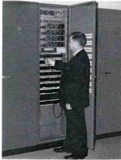
FIG. 2. Dan F. Hynes, chief engineer of video facilities is shown at the video distribution patch panel, which he designed and built for WWL-TV.
