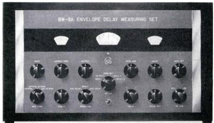
FIG. 4. This is the Type BW-8A Envelope Delay Measuring Set. All control functions are on the front panel for ease of operation.
