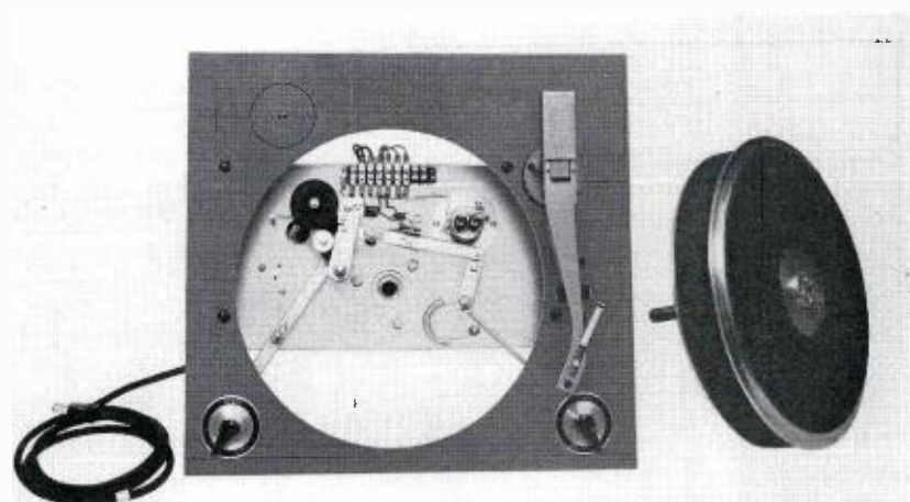
FIG. 3. The platter assembly is easily removed exposing the idler wheels and wiring terminals. Lubrication is thus simplified.
