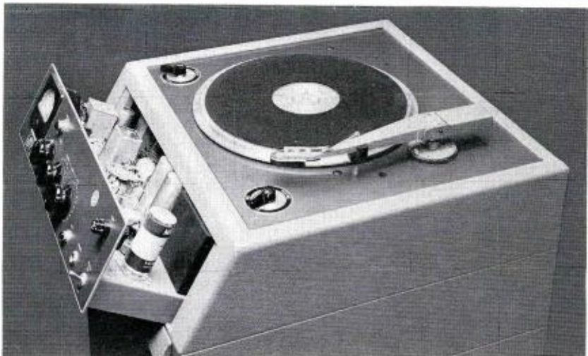
FIG. 4. This shows how the BA-51A Magnetic Record/Reproduce Amplifier is installed in the turntable cabinet and it is easily removed for servicing.
