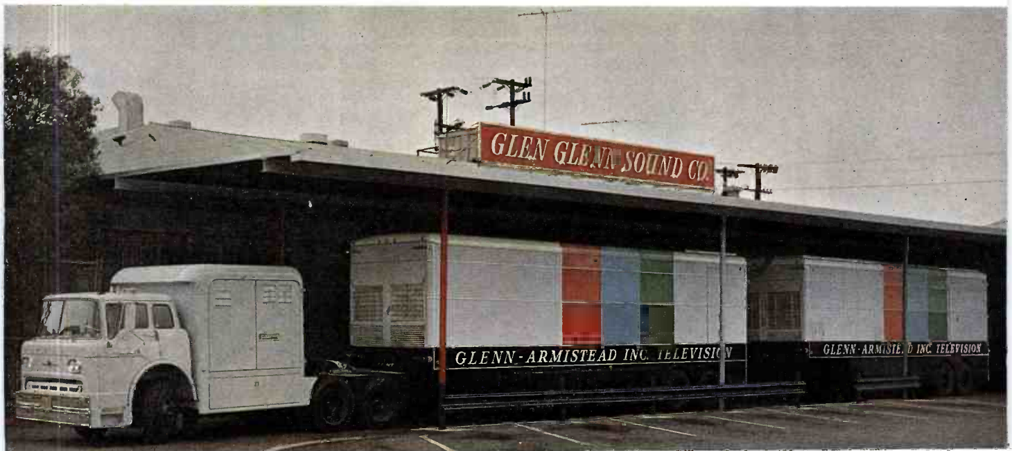
FIG. 8. Tractor and two trailers that comprise the complete Glenn-Armistead color TV production system. Normally, these units are parked at Glen Glenn Studios, where they function as fixed studios to produce color or monochrome TV tapes for clients. One unit contains the control, switching, and effects equipment. The other unit contains a film system and two color TV tape recorders.
