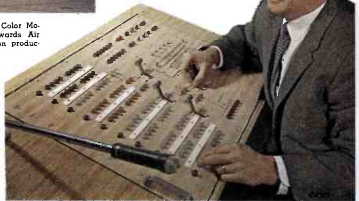
FIG. 7. Mr. Joseph Bluth, Vice-President in Charge of Technical Operations, seated at chief control position. Both tape recorders and film projectors can be controlled from this position. Live cameras are switched; sequences from tape, film, and slides inserted. Special effects can be executed as production rolls on. This is live editing.
