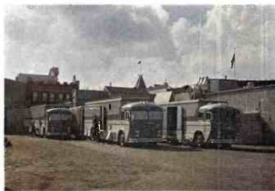
FIG. 3. Skelton Studios three mobile color tv units on location at Disneyland. One unit houses control and switching equipment, including special effects—this is the production center. Second unit houses tv tape recorders and film system. Third unit houses power generating equipment—to operate the system on location—space for storage, and a machine shop.
