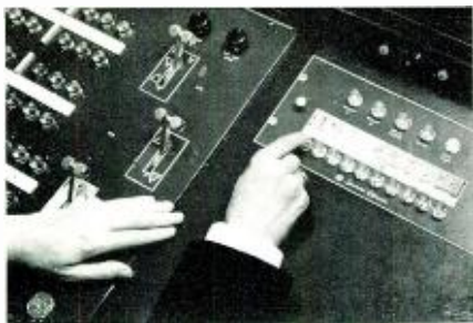
FIG. 5. Transistor switching and special effects equipment handle color and monochrome signals with equal ease, maximum quality.
