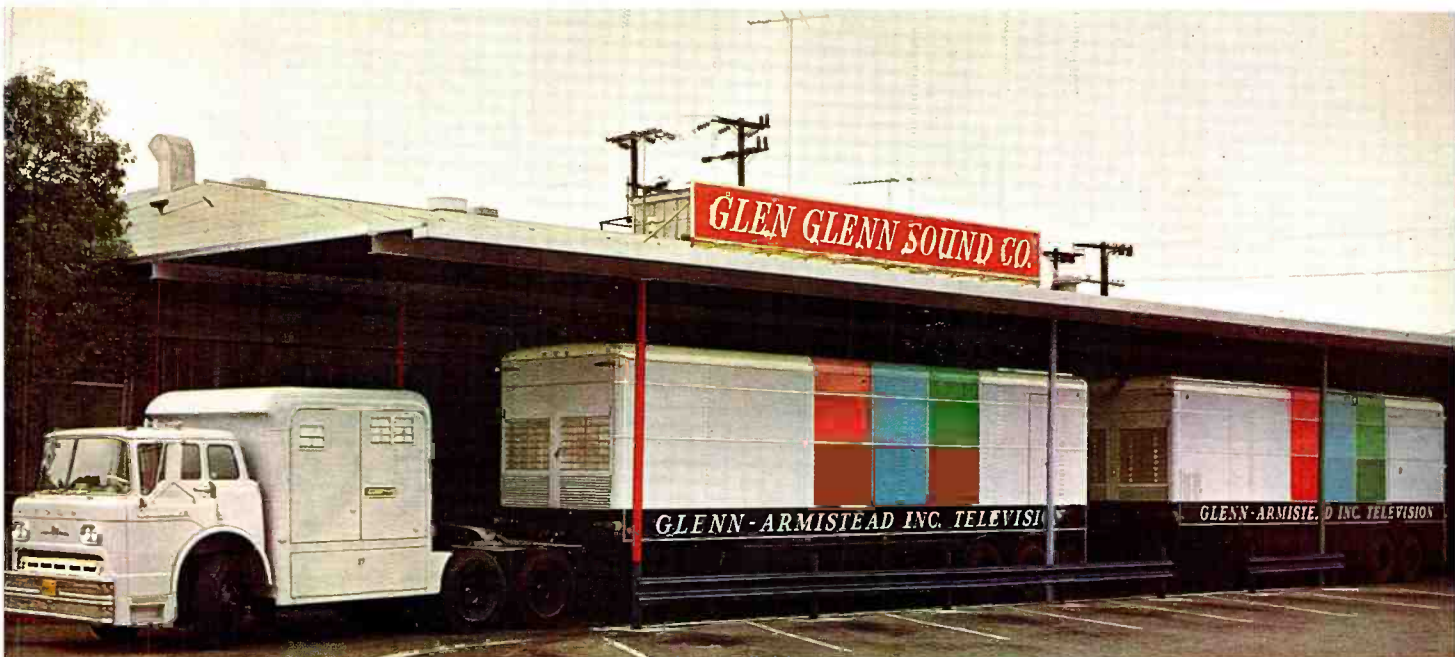
FIG. 8. Tractor and two trailers that comprise the complete Glenn-Armistead color TV production system. Normally, these units are parked at Glen Glenn Studios, where they function as fixed studios to produce color or monochrome TV tapes for clients. One unit contains the control, switching, and effects equipment. The other unit contains a film system and two color TV tape recorders.
