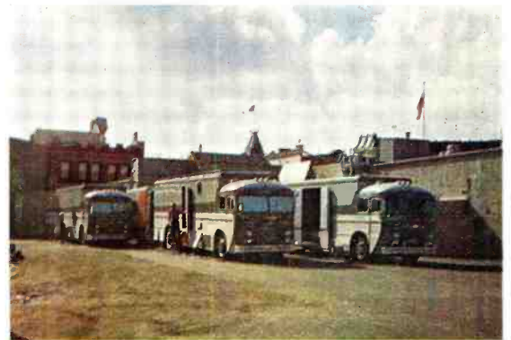
FIG. 3. Skelton Studios three mobile color tv units on location at Disneyland. One unit houses control and switching equipment, including special effects—this is the production center. Second unit houses tv tape recorders and film system. Third unit houses power generating equipment—to operate the system on location—space for storage, and a machine shop.
