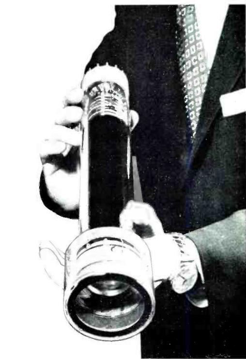
FIG. 2. Directly interchangeable with RCA 6474 and RCA 7513 color camera tubes, the RCA 4401 requires no greater lighting for color than for black-and-white telecasting.
