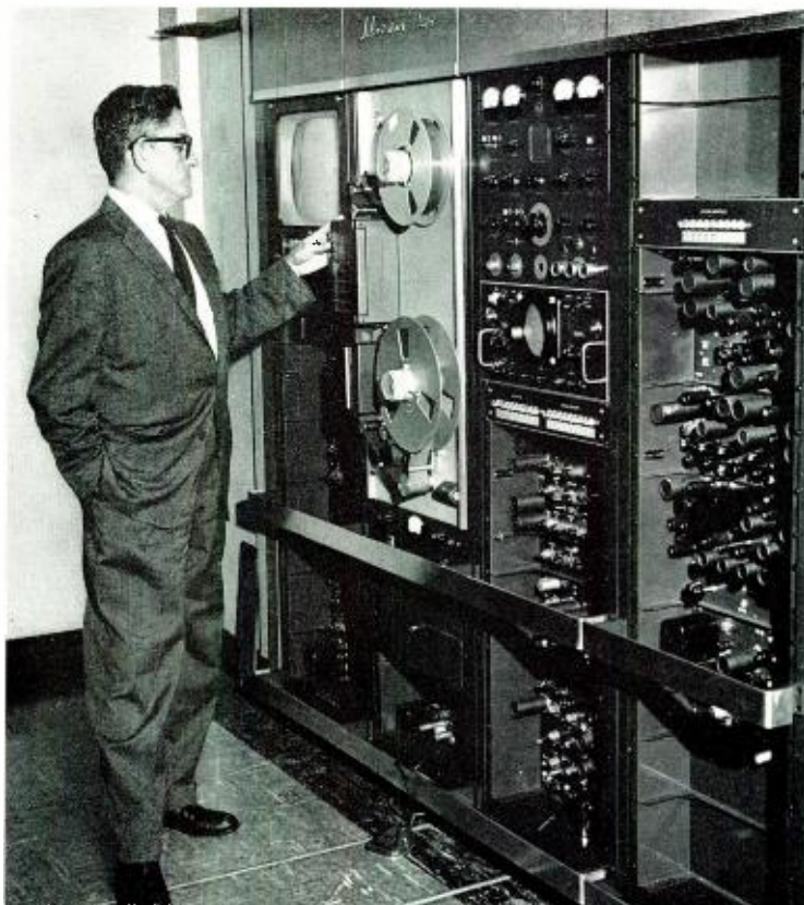
FIG. 2. Number one of two tv tape recorders at WBAP-TV. Both are color equipped.
