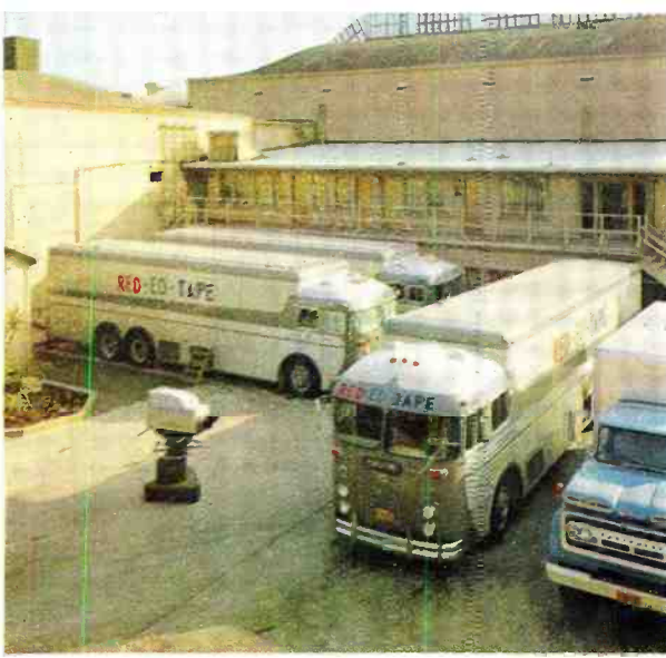
FIG. 1. Three Skelton RED-EO-TAPE Mobile Units. Control room bus is at left foreground, and the recording unit directly behind. The power and equipment storage bus is at right.
