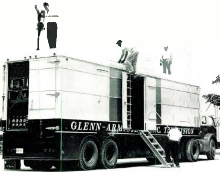
FIG. 1. Mobile TV on location—getting ready to operate—note ladder on door. Camera hoist on roof, which is reinforced to support cameras and operators—ready for color or monochrome operation.
