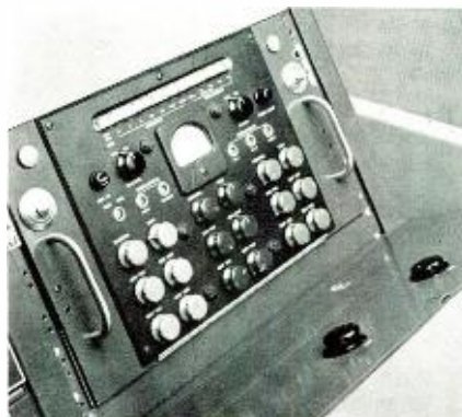
FIG. 4. Processing amplifier has compacted signal processing circuits resulting in minimum rack space and 50 per cent power reduction.
