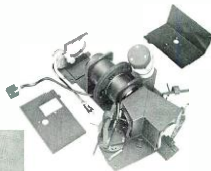
FIG. 3. New optics for the TK-41C incorporate prisms for color separation.
