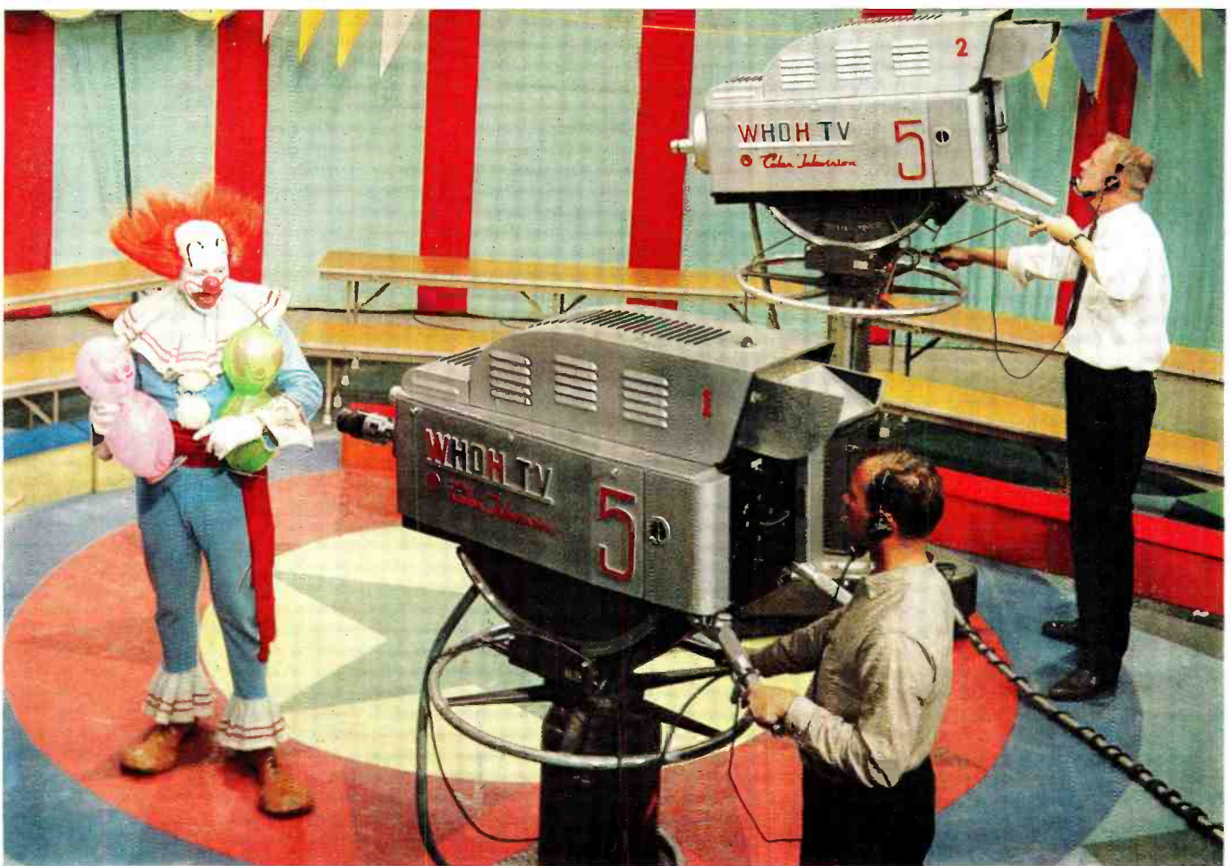
FIG. 1. All of WHDH-TV's local live colorcasts originate from two similarly equipped tv studios. Here "Bozo the Clown" performs for two TK-41 studio color cameras.
