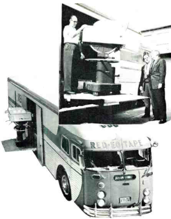
FIG. 5. Hydraulic lift gate enables one man to handle a TK-41 Color TV Camera by himself. Watching the demonstration are: Gibson Scott, director of transportation, Robert Cobler, chief engineer, and Edward Hilley, studio manager of Skelton Studios.
