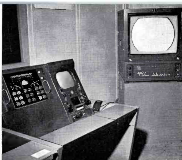
FIG. 28. Camera control console and 24-inch color monitor in control room of color TV instruction studio.
