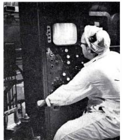
Pictures from underwater cameras guide technician in remote control of fuel loading at nuclear plant.
