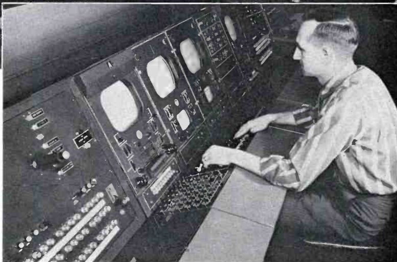
FIG. 10. Tv control showing a close up of the second TS-21 switching panel which is adjacent to the BC-6 audio console.
