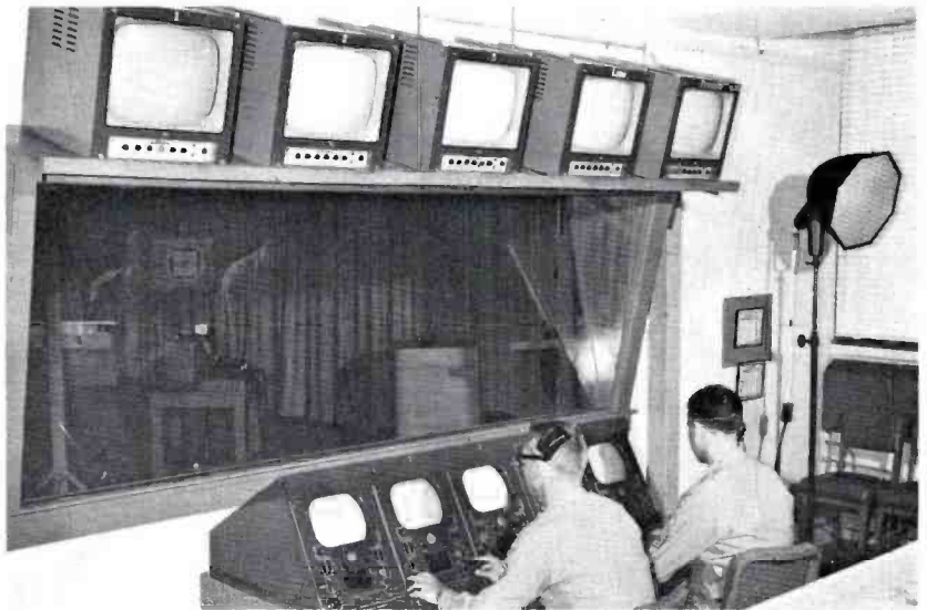
FIG. 19. At the video console, Video Engineer, Malcolm Carr corrects camera shading while Technical Director, Owen Stofel observes the outgoing picture. Overhead monitors are for three TV cameras, Line and Preview.
