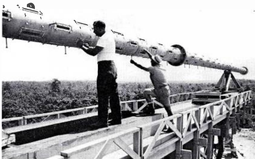
CRADLED IN A HUGE TURNTABLE at RCA's test site near Camden, N. J., this 114-foot UHF antenna, first of its type, is capable of radiating the maximum 5 megawatts of ERP. The new antenna weighs 13 1/2
