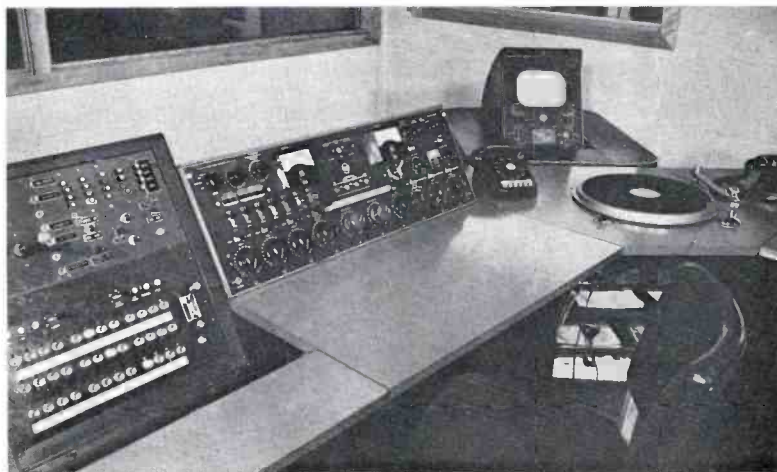
FIG. 10. Tv control showing a close up of the second TS-21 switching panel which is adjacent to the BC-6 audio console.
