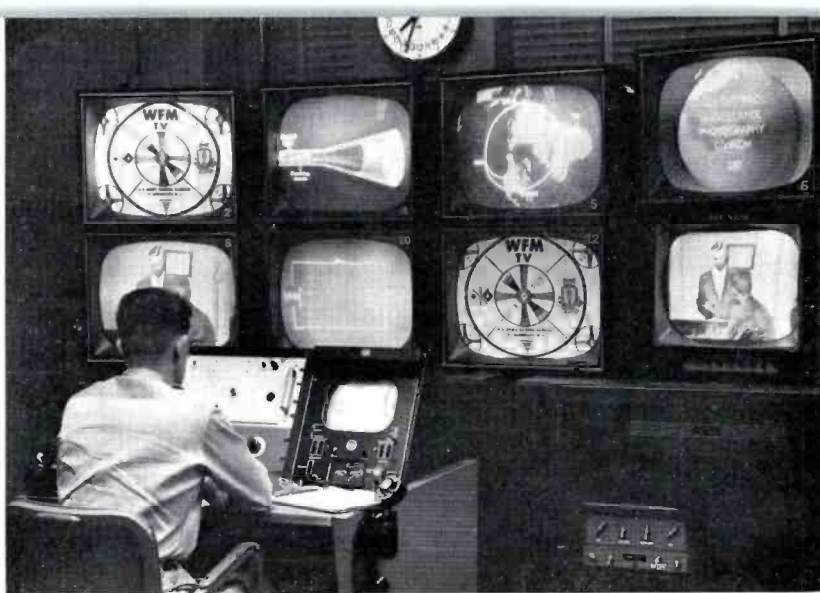
FIG. 25. Master control console, where pictures are selected for transmission on each of WFM-TV's seven channels.
