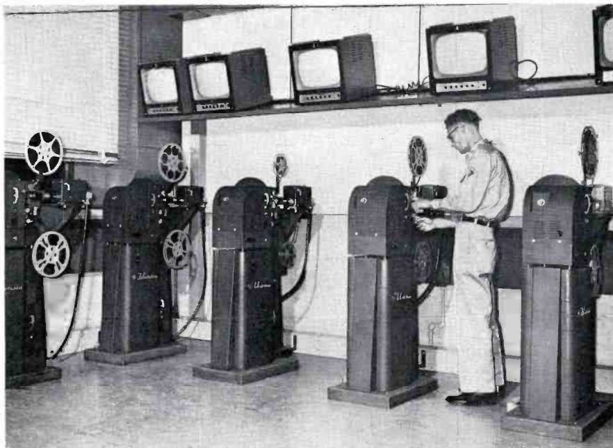
FIG. 6. Six TV film chains are used to distribute training films to classrooms.
