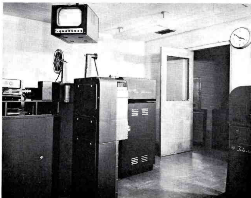
FIG. 11. WKZO-TV projection room showing TK-26 color film chain, TK-21 monochrome film chain, TP-15 multiplexer and TP-6 projectors. The station produces many of its own color film specials.
