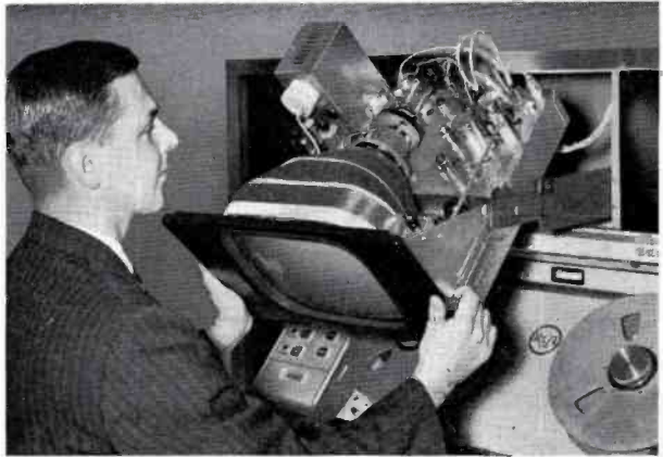
FIG. 19. Picture monitor also incorporates convenient slide-out and tip-down accessibility.
