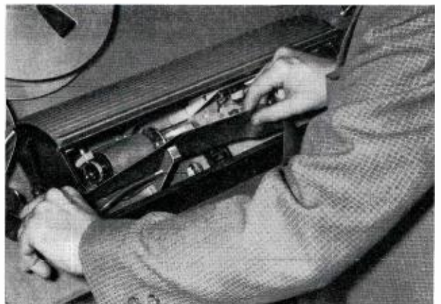
FIG. 11. A single protective cover shields the video headwheel assembly and the audio, erase, cue and control track heads. This slides back against the tape deck for easy threading . . . from a natural and comfortable position.
