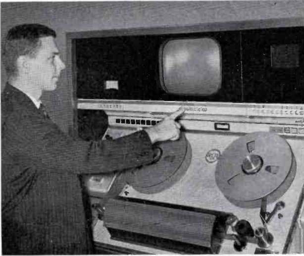
1 FIG. 3. The monitoring deck of the TR-22 includes high quality 14-inch picture monitor (center), TO-2 precision waveform monitor (right) and audio monitor (left) including speaker and VU meter.
