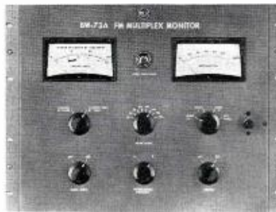
FIG. 16. The Type BW-73A Multiplex Monitor. A new instrument, designed for accurate monitoring of FM transmitters handling stereo and/or SCA programming.
