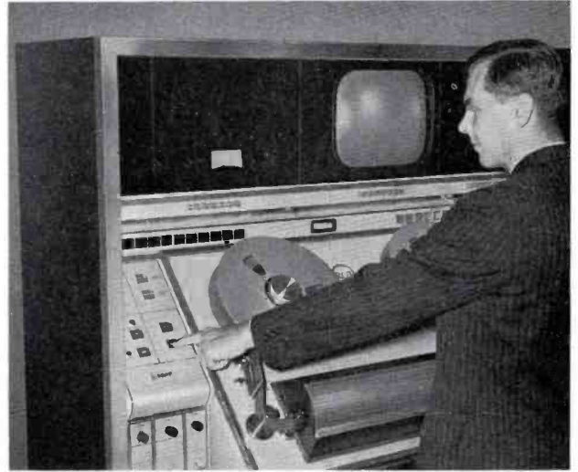
2 FIG. 4. The tape deck slopes at a 45-degree angle giving the operator maximum convenience, comfort and accessibility for routine control and operating functions.
