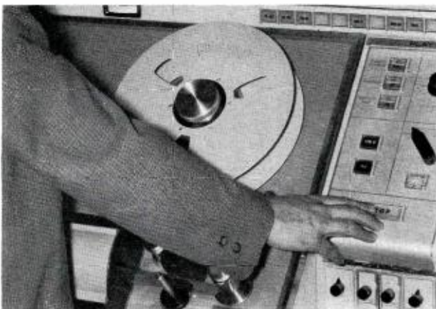
FIG. 10. Frequently used controls: play, standby, stop, etc. are located at the natural extension of the operator's arm. Less frequently used controls are beyond the operator's reach so that they cannot be disturbed during normal operation.
