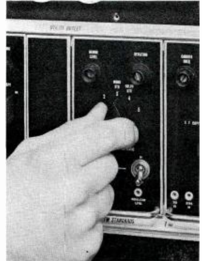
FIG. 12. A five-position switch on the front of the FM standards module selects proper pre-emphasis for monochrome or color recording or for any special pre-emphasis desired.
