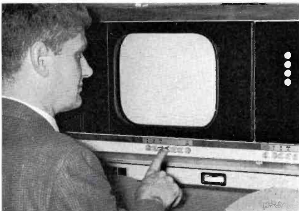
FIG. 8. A high quality 14-inch picture monitor and newly-designed waveform monitor are located at the operator's eye level. Pushbuttons at the base of monitoring facility expedite check-out, keep the operator informed of what he is looking at.
