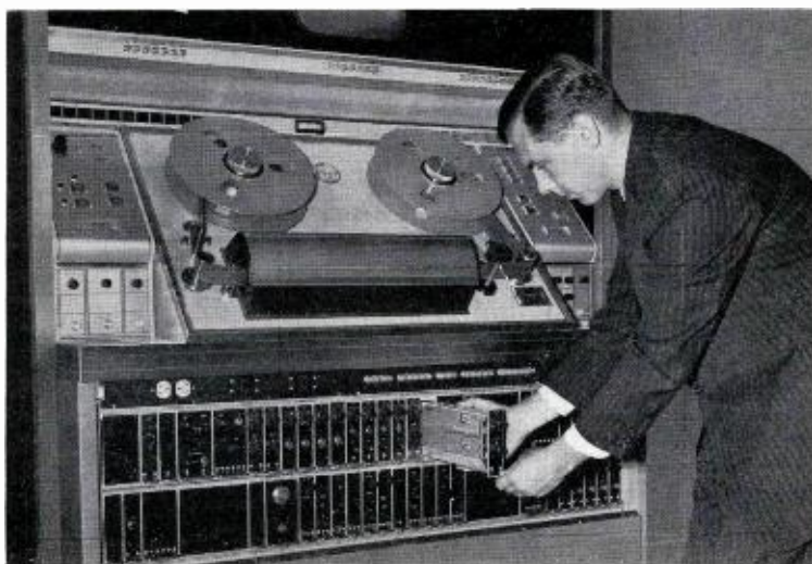
3 FIG. 6. The module bank or electronics area houses 44 modules which contain circuitry for video and FM processing and for all the servos required by the machine.
