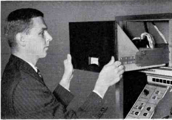
FIG. 18. Audio shelf slides out and tips down to expose audio amplifier, speakers and VU meter.
