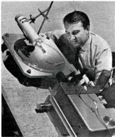
At RCA Laboratories, experimental laser is focused to produce a continuous beam of infrared radiation.
