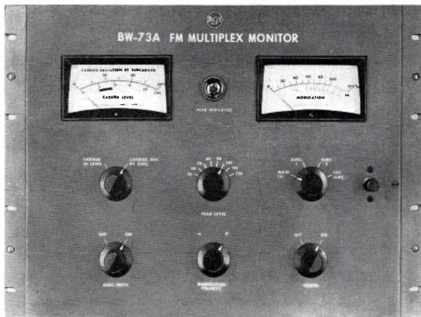
FIG. 1. Type BW-73A FM Multiplex Monitor, a convenient instrument for monitoring and measuring multiplexed-transmitter performance.
