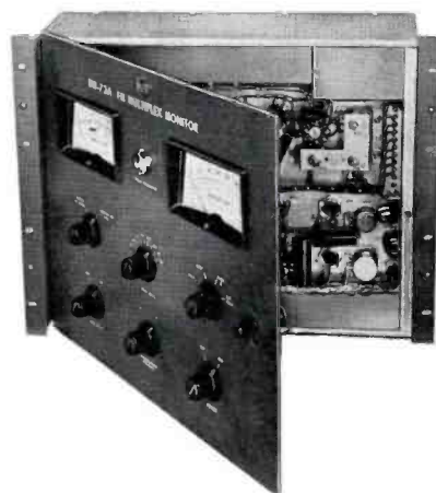
FIG. 3. Swing-aside front panel provides access to the chassis underside. This feature allows examination of circuitry while instrument remains in rack.
