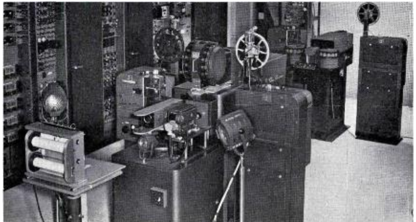
FIG. 10. Color film grouping includes all equipment necessary to originate color films, slides and opaques. A TP-15 multiplexer accommodates TK-26 color film camera, two TP-6 16-mm film projectors, TP-7 dual-drum 2 by 2 slide projector and opaque attachment.
