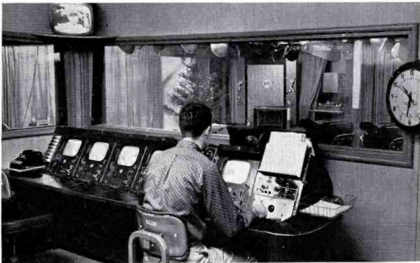
FIG. 14. Video Control. Five TM-6 Master Monitors are mounted in the console. The screen in the upper left displays the air signal. Video Supervisor John Raymond prepares for a switch.
