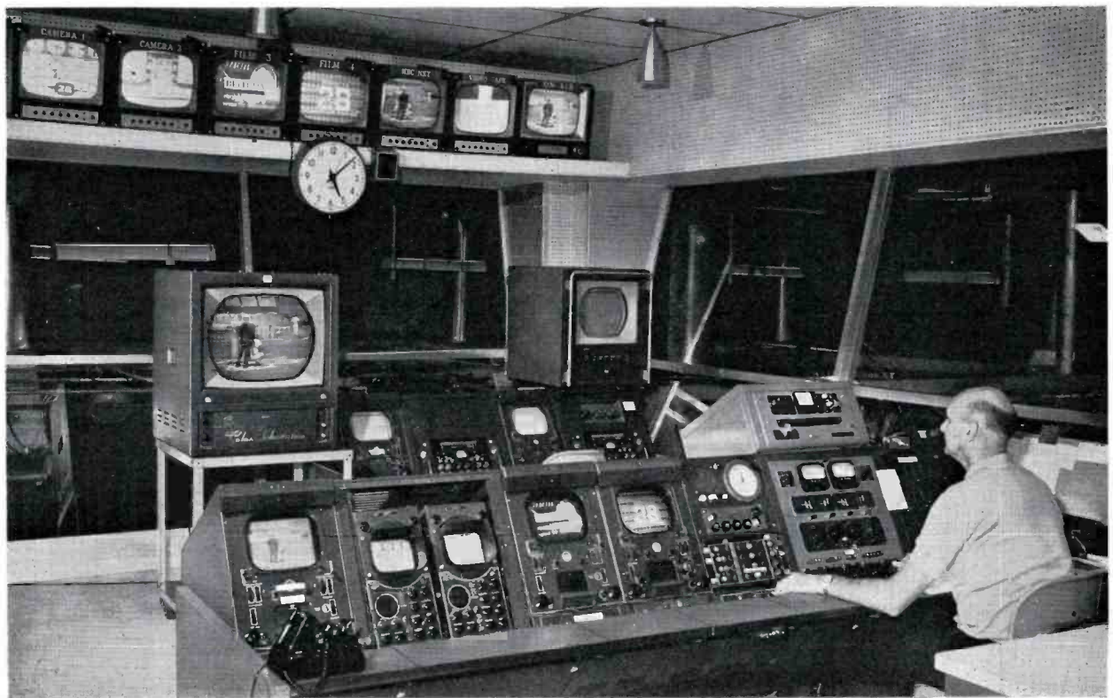
▲ FIG. 12. Two new TR-22 transistorized tv tape recorders, recently installed in the control area. These two compact units are self-contained tv tape recording facilities—require no external racks.
