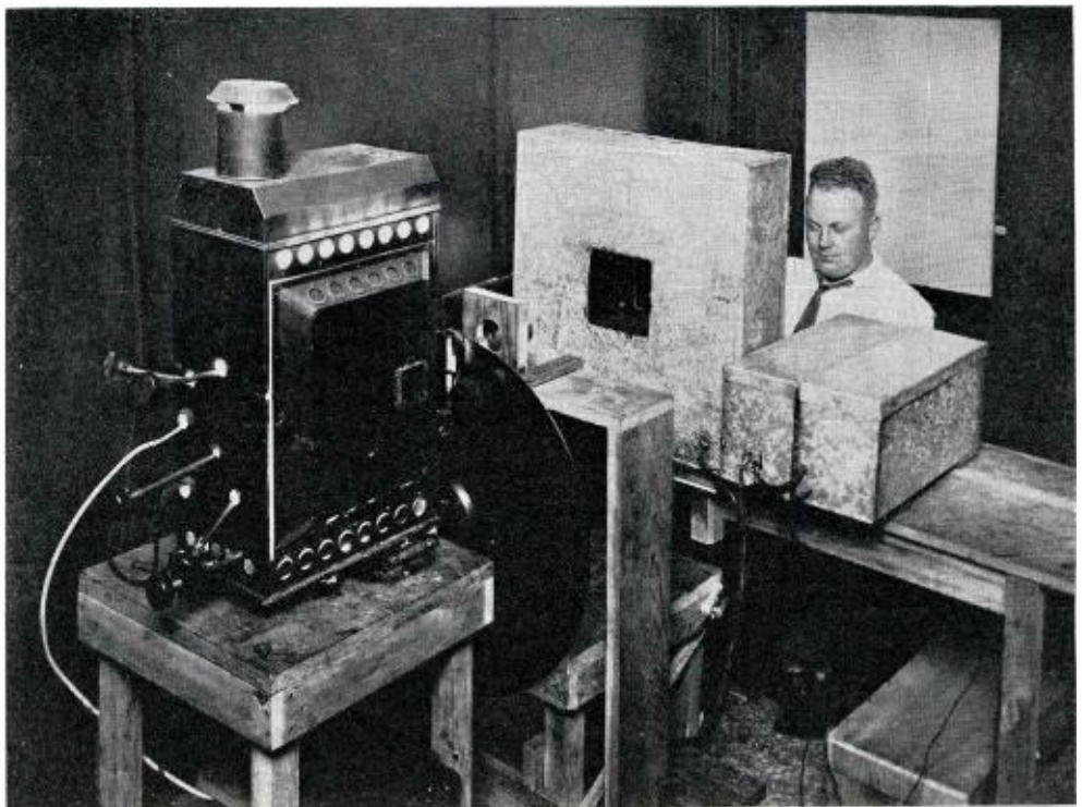
Photograph made on October 21, 1927, shows Merrill Trainer in front of early television scanning equipment. Arc lamp at left furnished high-intensity light which spirally arranged holes in Nipkow disc caused to scan performer's face. Photo cells on far side of the square doughnut (facing performer) picked up light reflected from performer's face and converted this to video signal.
