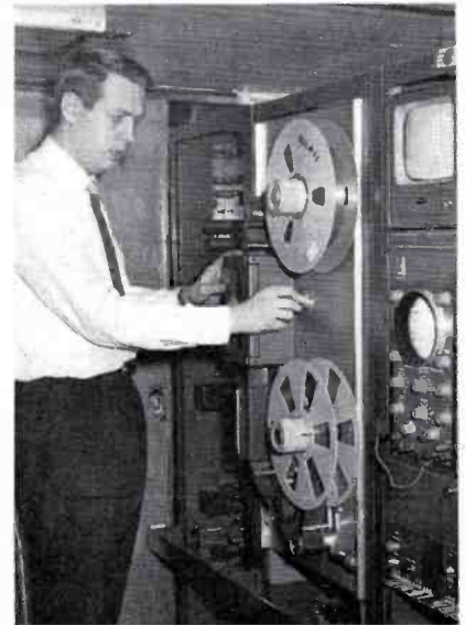
FIG. 20. Engineer Tom Brask, remote supervisor at TR-11 TV tape recorder in mobile unit. Station engineers installed the TR-11 in short racks to fit the truck.
