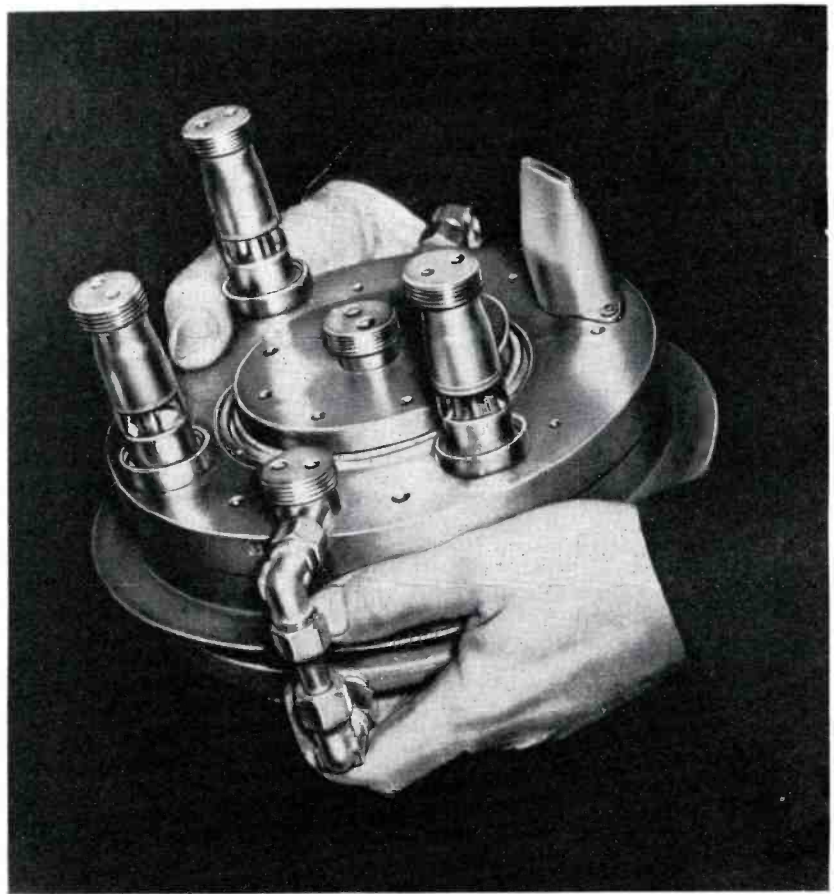
FIG. 4. The UHF Tetrode (6448 or 6806). Considering its power capabilities, this tube is small in size and extremely rugged. Installed in this transmitter, the tube becomes part of a concentric cavity with only two tuning controls.
