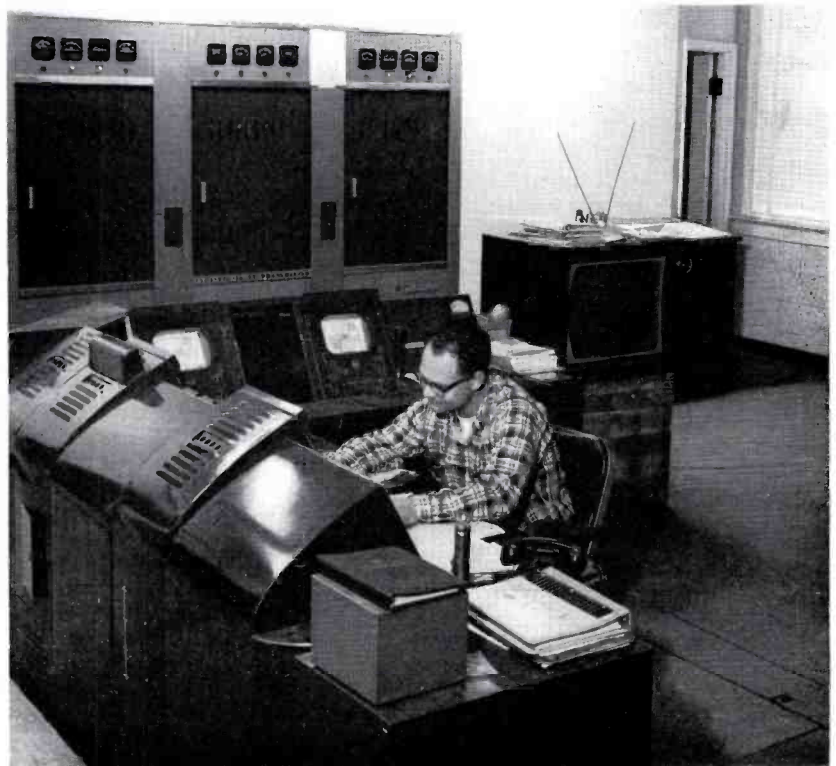
FIG. 16. UHF Television Transmitter, type TTU-1B. Transmitter supervisor, Harold Wagner is at operating console.
