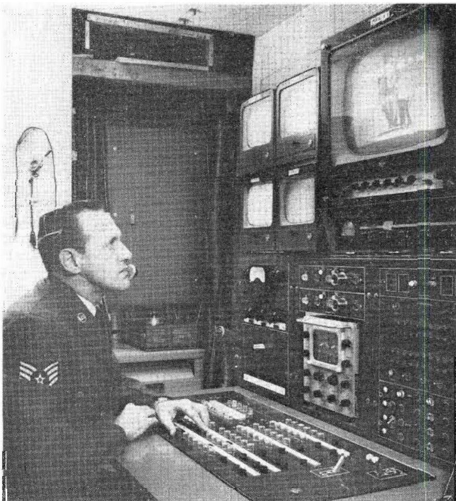
FIG. 11. TV switching system Type TS-40 selects program source requested in any of the conference rooms or offices. System permits special effects to be inserted.
