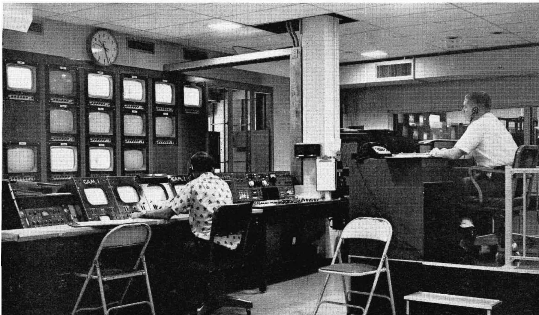
FIG. 10. Master control with camera control monitor (left), master control board (center), and technical director's position (right).
