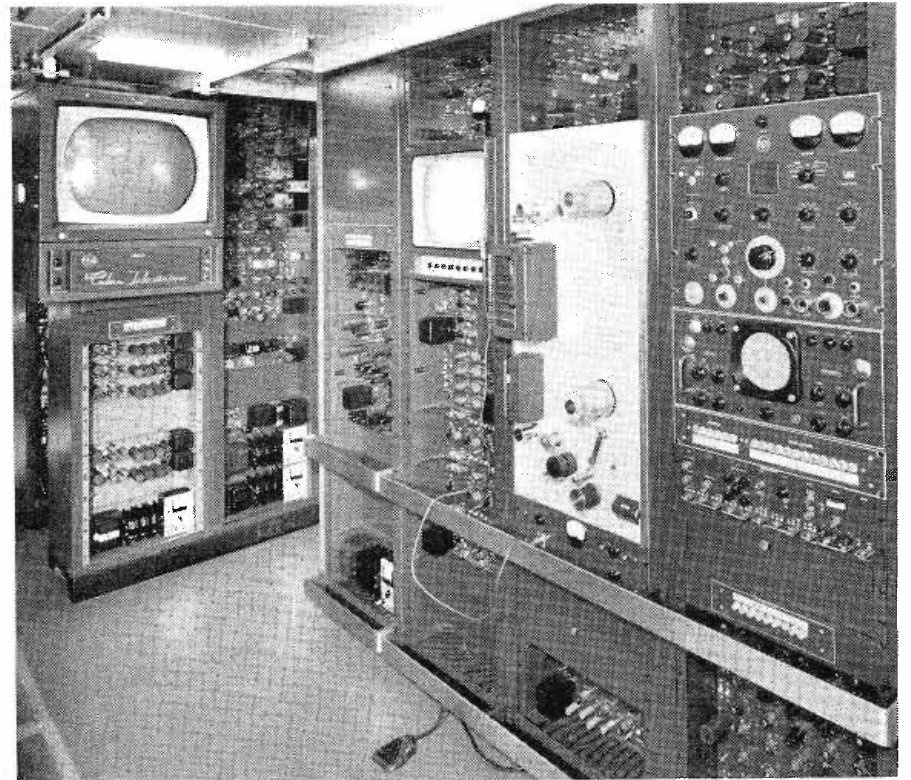
FIG. 32. TV tape area in S.S.D. color mobile van.
