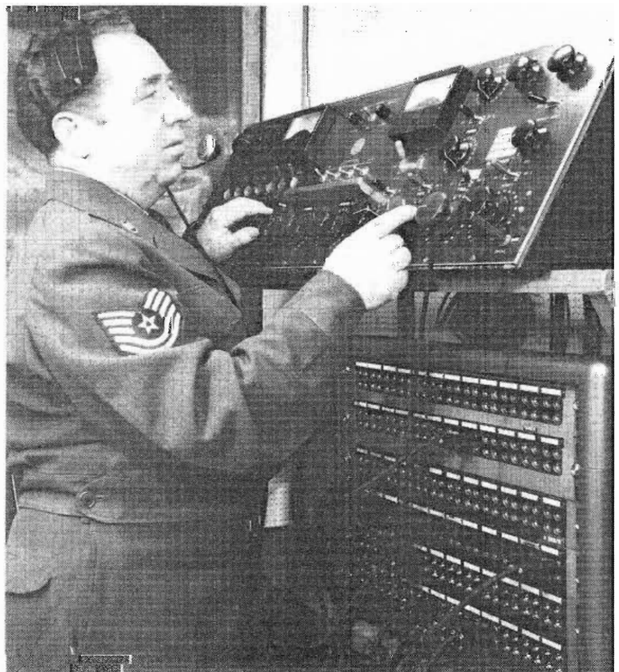
FIG. 12. Control room equipment includes dual channel audio console Type BC-7, permitting simultaneous use of two sound channels.
