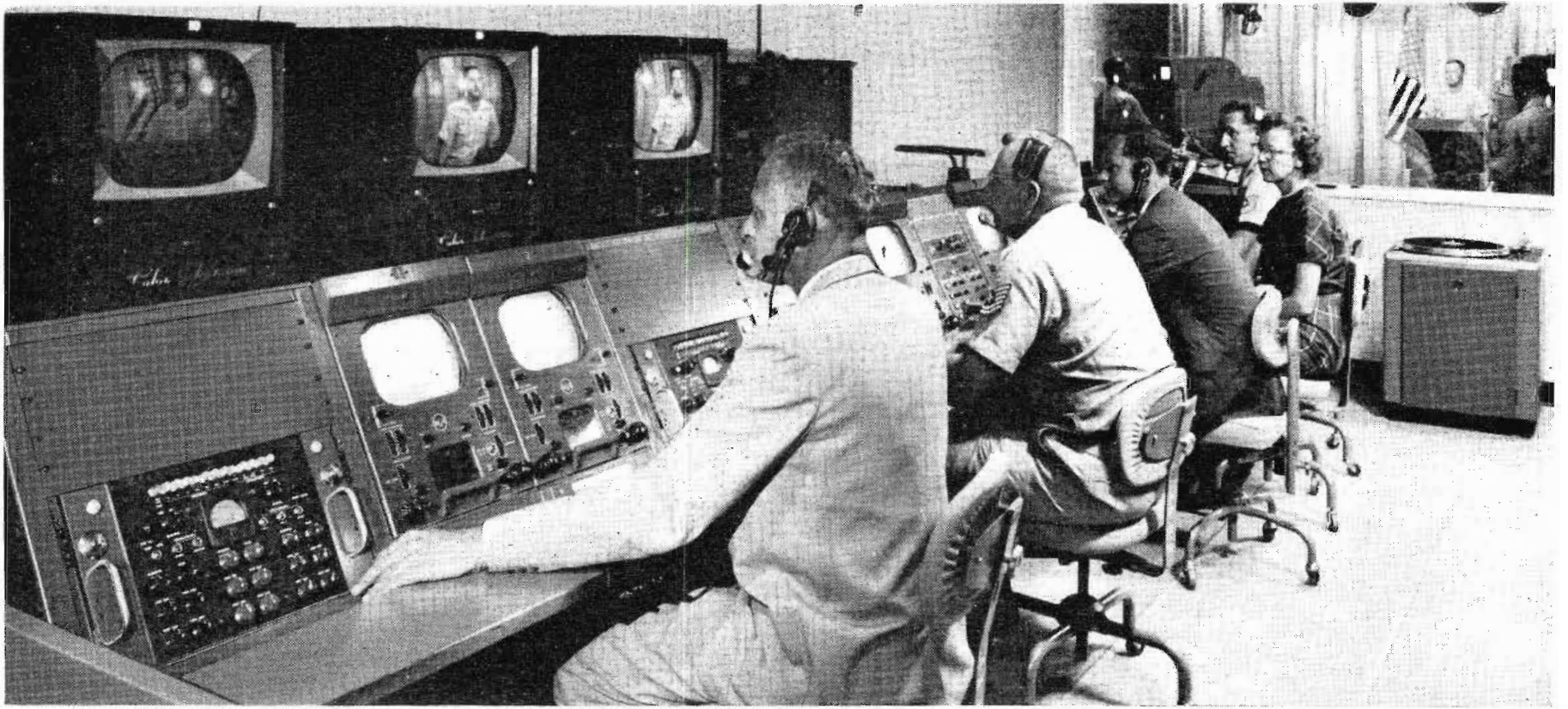
▲ FIG. 21. Studio Control Room at Patrick. Cameras are switched here and films are integrated in TV Tape presentations. Note, at far right, window looking into TV studio.
