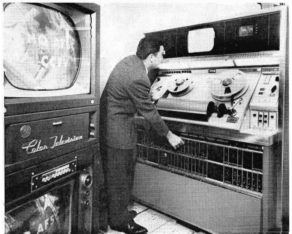
FIG. 16. Equipment complement at Andrews includes transistorized TV Tape Recorder, Type TR-22, for producing color briefings.
