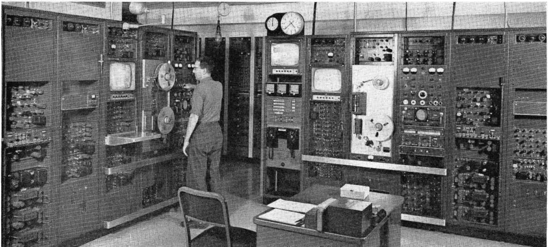
▲ FIG. 18. TV tape area includes two fully-modified TRT series TV Tape Recorders.
