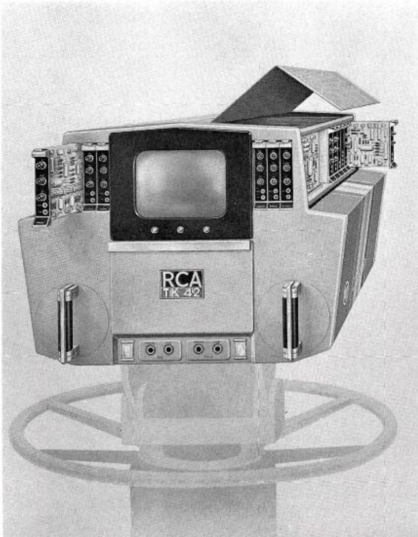
FIG. 2. Rear view of the TK-42 Color Camera. One group of plug-in transistor modules flanks the viewfinder. Another group is located along the side. "D" handles shown at the back control zoom and focus of the lens.
