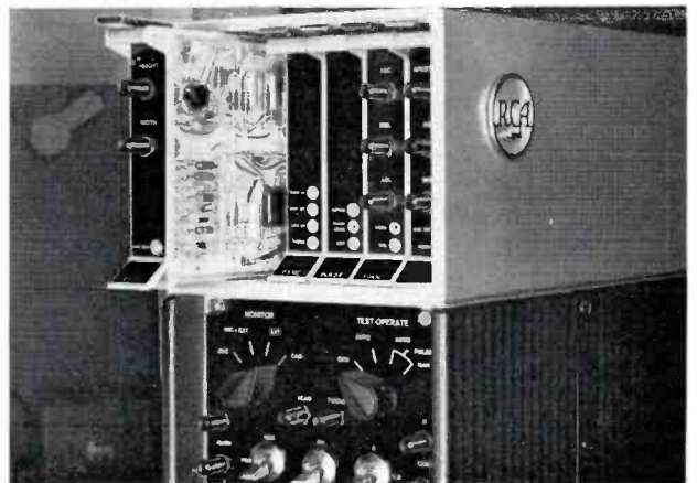
FIG. 8. Camera circuits are also plug-in modules. Adjustments require no attention after setup. A monitor feed is available at the camera. No high voltages are present in camera cable.
