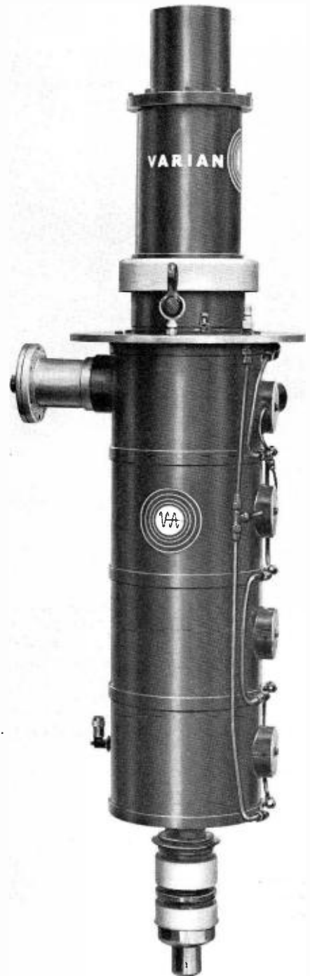
FIG. 4. New integral-cavity vapor-cooled klystron used in new look 30 KW UHF Transmitter. Because of smaller cooling system required it reduces overall power consumption by nearly one-fourth. Factory-tuned cavities and all-metal construction eliminate many troubles of earlier type klystrons.
