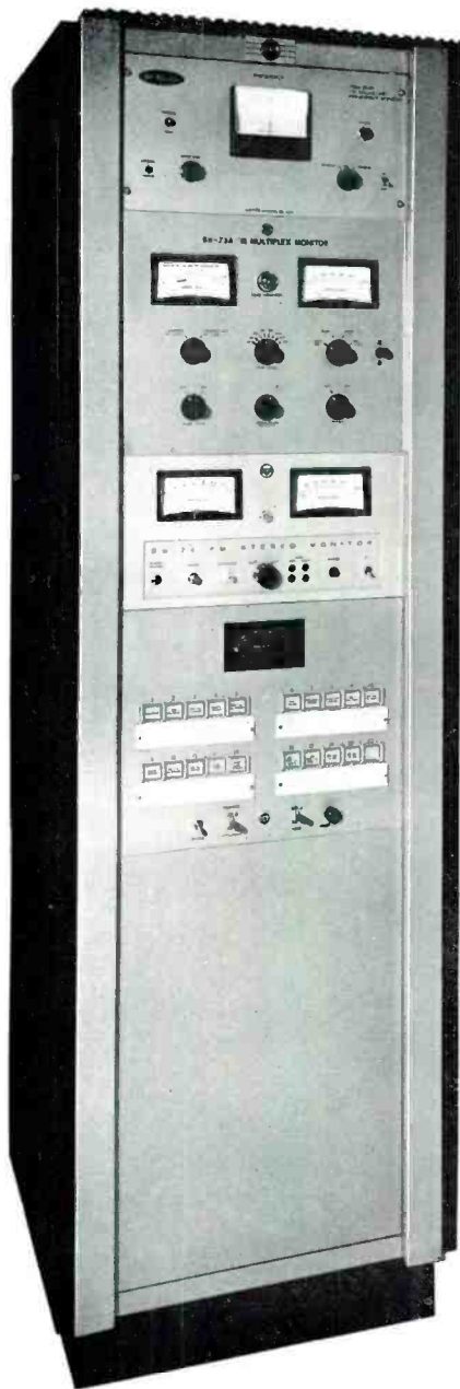
FIG. 13. Type BTR-20C Remote Control unit is normally located in input and monitoring rack, shown below. Other units, top to bottom, are TBM-3000 carrier frequency monitor, BW-73A multiplex modulation percentage monitor, and BW-74 adapter for use with multiplex monitor to check transmitter stereo performance.
