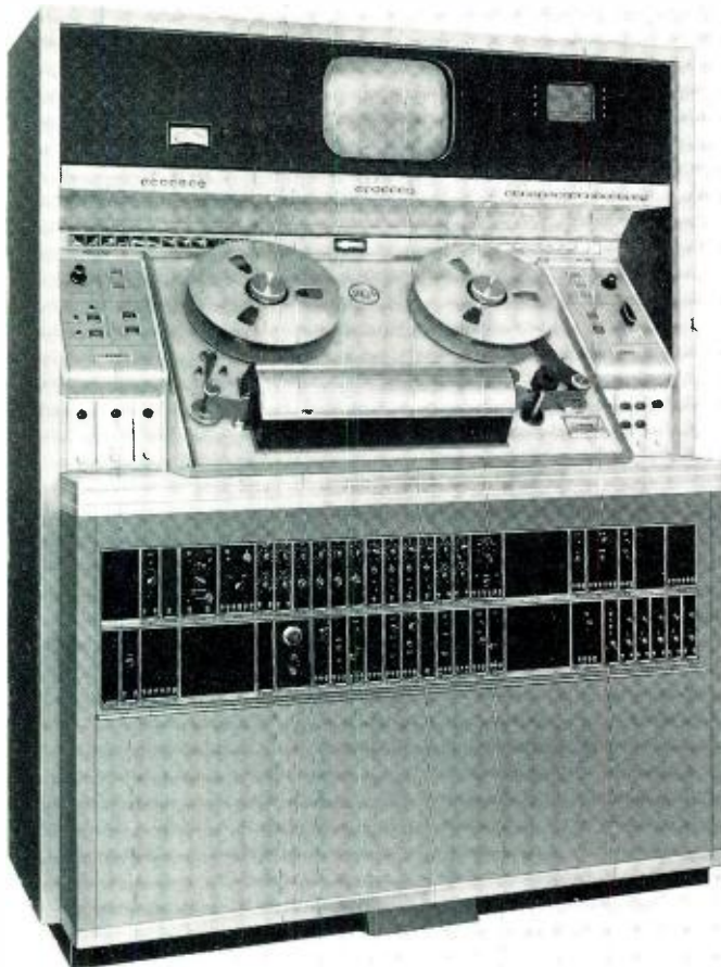
Modular layout of the deluxe TR-22. Many of these same modules are used in the TR-5, TR-4 and TR-3.
