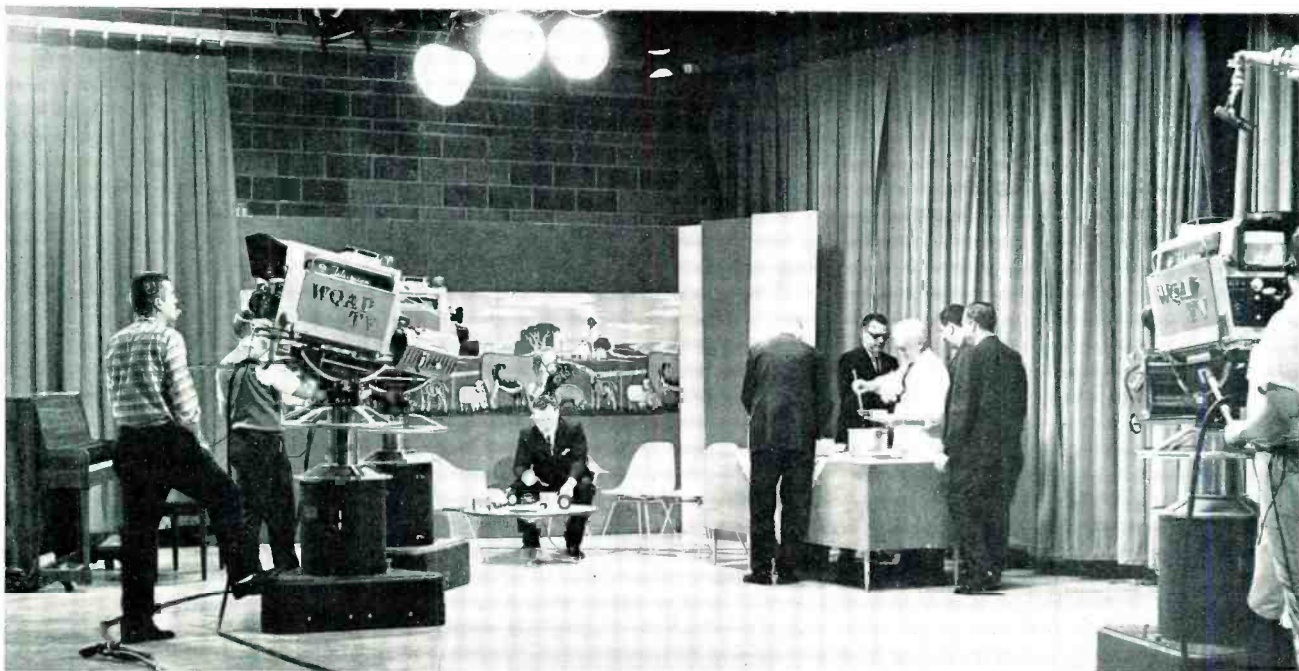
FIG. 5. Three TK-60 Cameras are used in daily production of "Channel 8 Farm Report" in Studio A.
