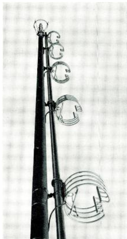
FIG. 2. A four-section BFA- B antenna as it appears when pole-mounted. Pole-mounting provides excellent horizontal-pattern circularity.
