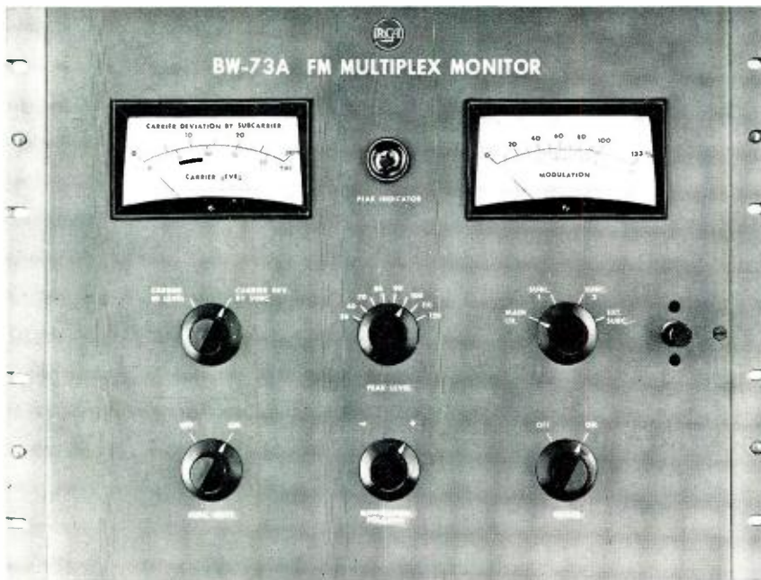
FIG. 4. The BW-73A is both a quantitative and qualitative modulation monitor for demodulating and separating main-channel and SCA audio.
