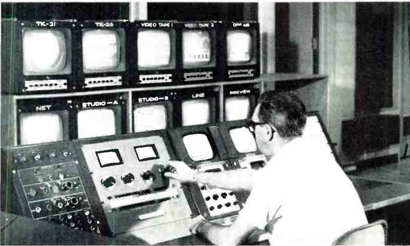
FIG. 24. Master Control with Bill Benjamin. Shown is an RCA TS-40 switcher which is an audio follow pre-set type switcher, custom built for this installation. There are remote panels for both TV tape machines. The Master Control operator has the ability to do all station breaks from this position.
