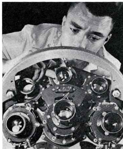
Close-up view of RCA camera system aboard Ranger.
