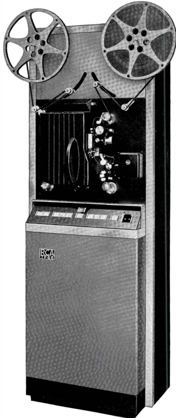
New 16mm Television Film Projector, Type TP-66
