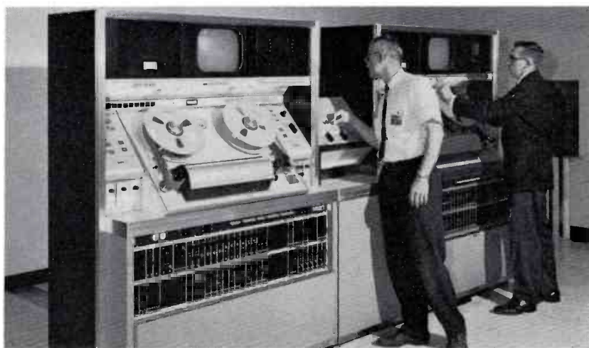
FIG. 28. Special TV tape delegate control was designed and built for WOC. Note that housing blends with RCA tape recorders.
