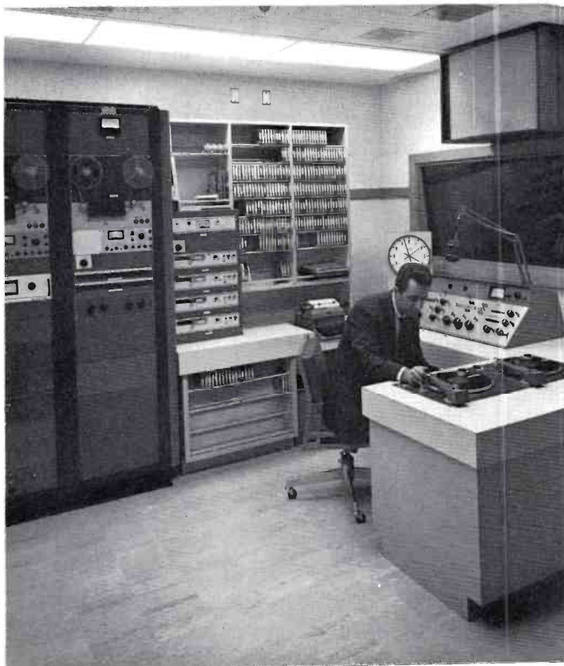
FIG. 35. WOC custom built combo console in radio studio No. 1. RCA transistorized audio tape machines and control console are employed. ▼
