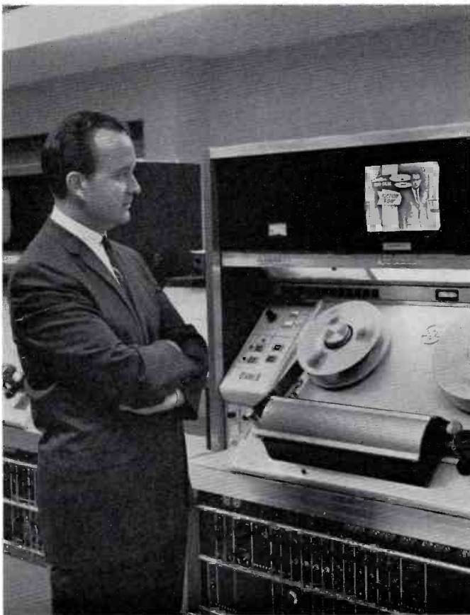
FIG. 43. Two minutes after taping, commercials are reviewed on one of the two RCA Deluxe TR-22 tape installations in the WOC-TV control room.
