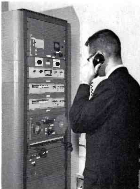
FIG. 19. Spot news recording center, which permits recording off telephones, 2-way radio, or from News Booth control. Equipment includes RT-7 Cartridge Tape machines and NBC Hot-Line alert receiver.
