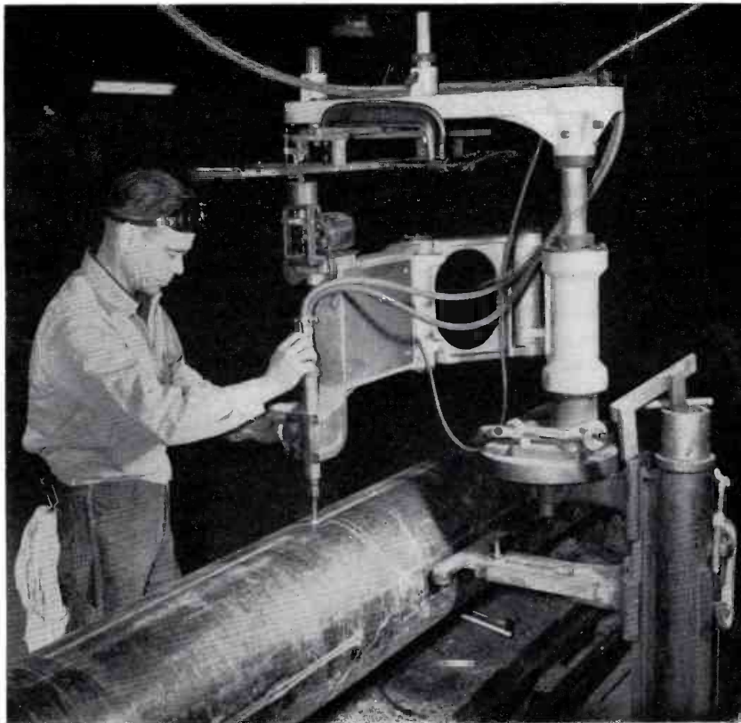
FIG. 4. Cutting the radiating slots in the structural-steel pole. Oxy-acetylene cutting torches, under precision control, burn away unneeded steel to form the dozens of radiating slots in each UHF-Pylon antenna.
