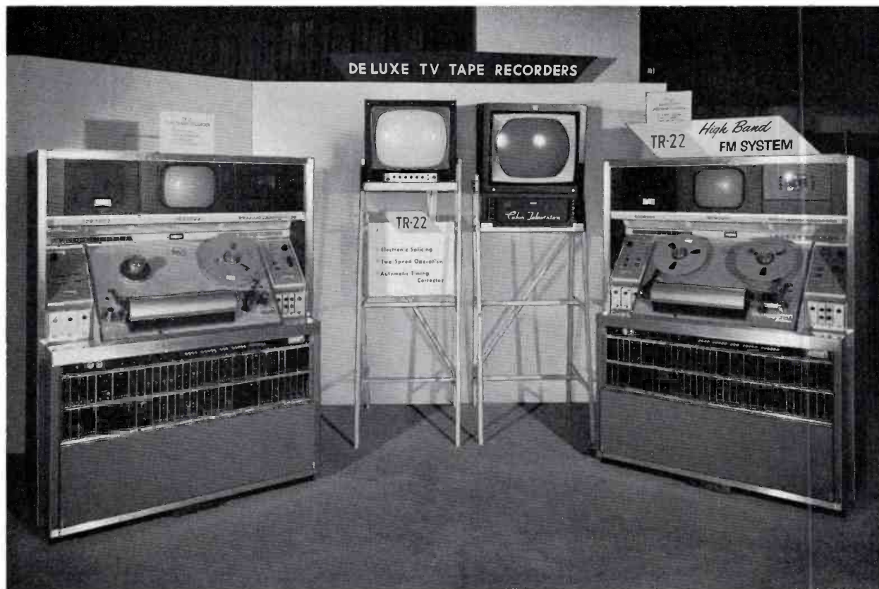
FIG. 1. Deluxe RCA recorder, TR-22, equipped for high-band operation, is shown at right in this 1964 NAB Convention photo. More than 20 RCA recorders, high-band equipped, have been delivered to international customers.
