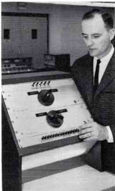
FIG. 25. Chief engineer David Hauser at custom-built delegate control in projection room. Top switches operate intercom. Upper large switch delegates film projectors and slide projector on TP-11 island to "A", "B", or Master Control. Lower large switch delegates projectors and slide projector on TP-15 (color) island to studio controls. Bottom row of push buttons is WOC house monitoring system, to punch up any of 15 video sources with matching audio.
