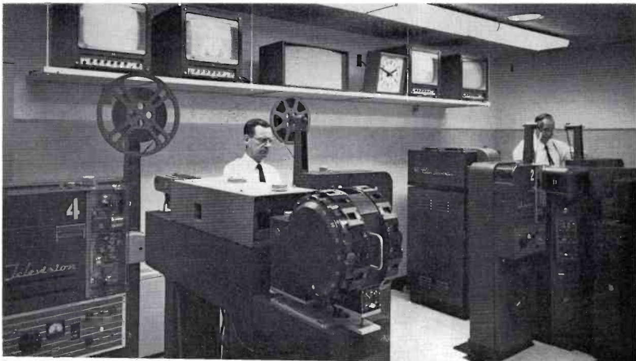
FIG. 33. Two islands of film equipment at WOC. Each is equipped with two film projectors and a slide projector. Island at left handles black and white. Island at right handles color as well as black and white.
