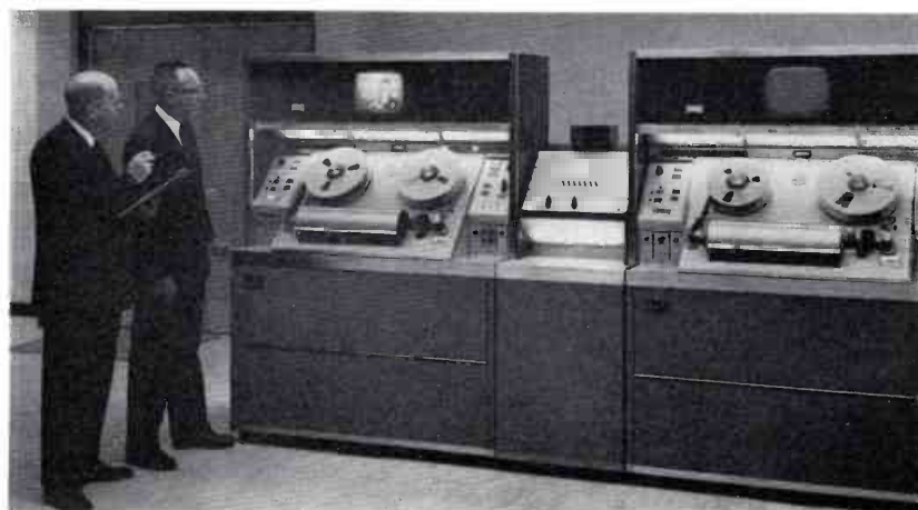
FIG. 17. Control for Studio "A" (shown) is identical with Studio "B". Both feature TS-40 custom-built switchers with special effects. Note transistorized audio control at right.
