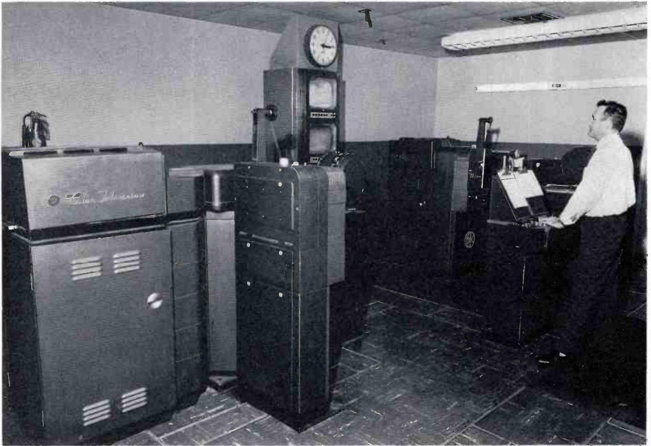
FIG. 19. Film Projection Room. Equipments are operated by the projectionist-switcher at an RCA custom-built control pedestal. They may also be remotely controlled from Control "A" or Master Control. One monitor is for "off the air" viewing, the other is switched from the control pedestal for previewing.
