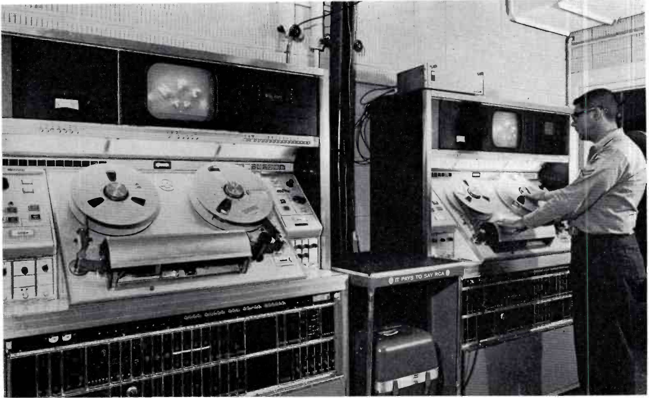
FIG. 11. Use of two television tape recorders permits simultaneous rehearsals and programming, and provides backup in recording.
