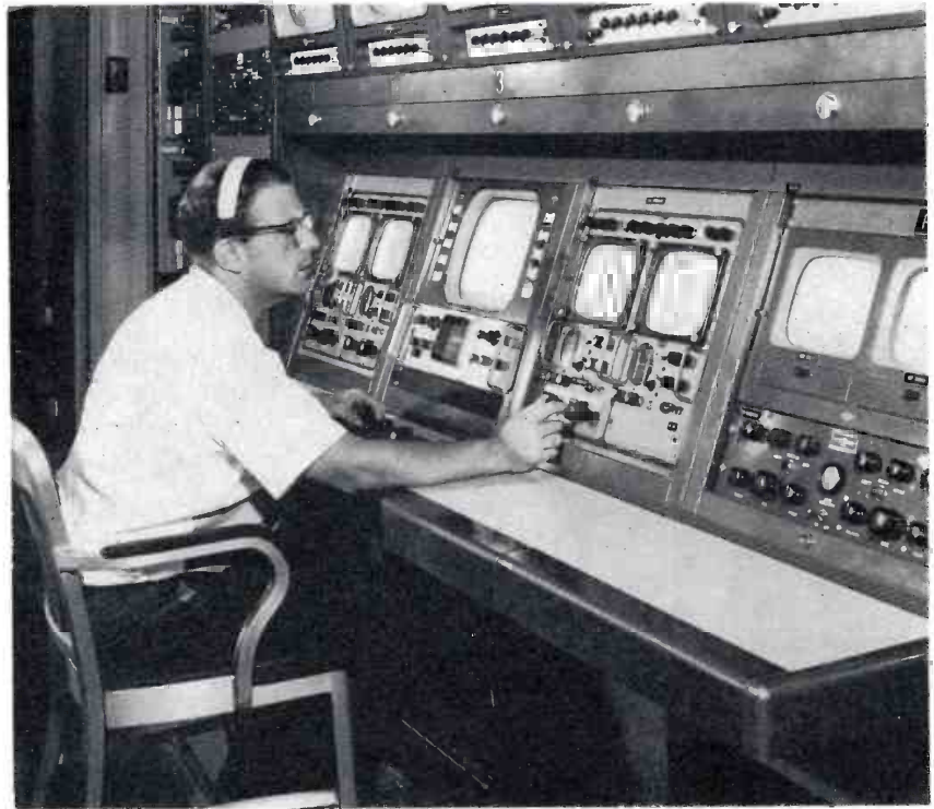
FIG. 9. Video control desk contains switcher for selecting cameras, film chain and tape, and remote controls for film and tape.
