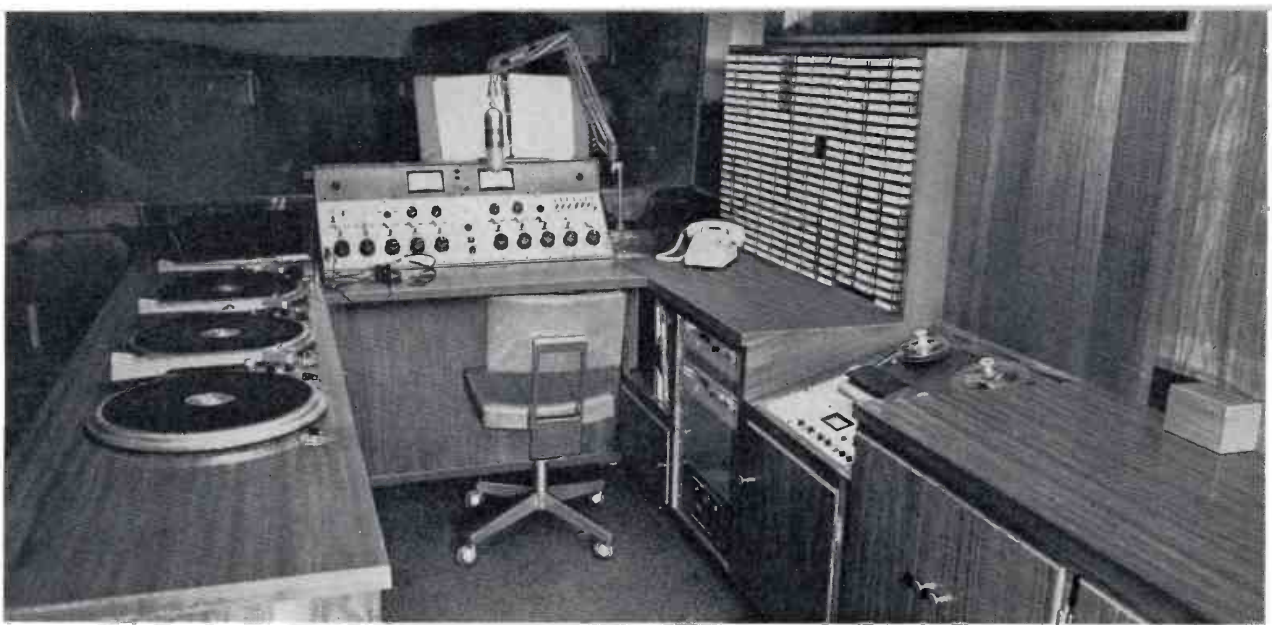
FIG. 4. Master Control is equipped with three turntables, a reel-to-reel tape deck, two cartridge-tape machines and, of course, the control console. Note cartridge-storage bins above cartridge-tape machines.
