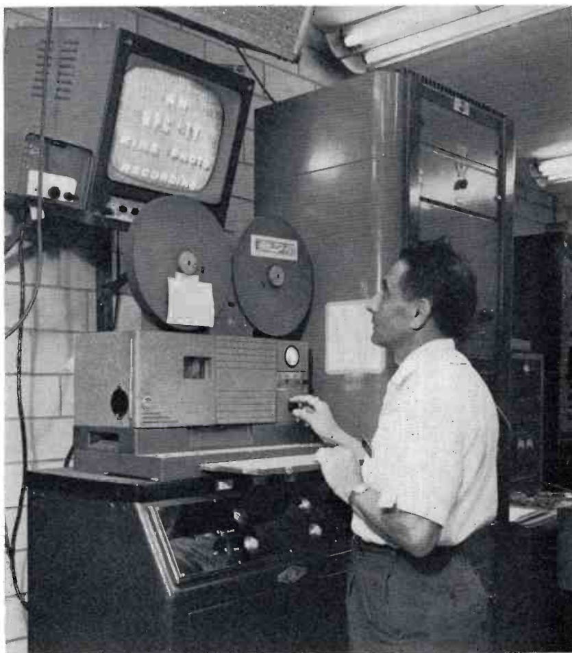
FIG. 18. RCA optical sound recorder used at NPC to record sound on film by using the double system.
