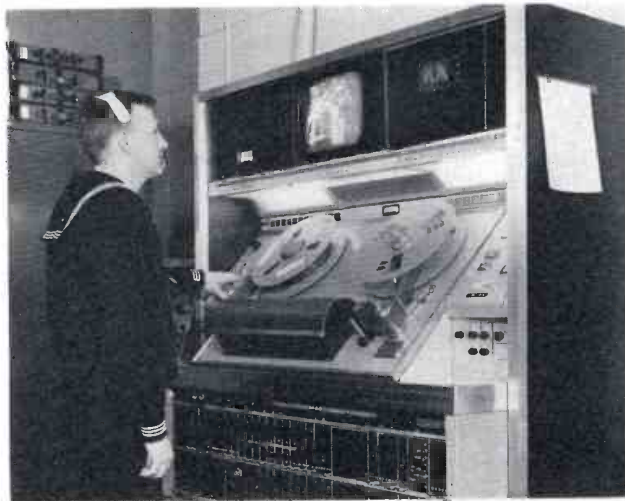
FIG. 4. Television tape machine used for recording TV studio pickups. Also used for playback of TV tape recordings to feed the Kine-Recorder.
