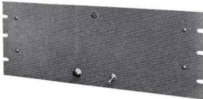
FIG. 5. The transmitter unit of the BTRA-5A Tone-Alarm System. This unit utilizes one of the remote-control telephone pairs to communicate with its studio counterpart.
