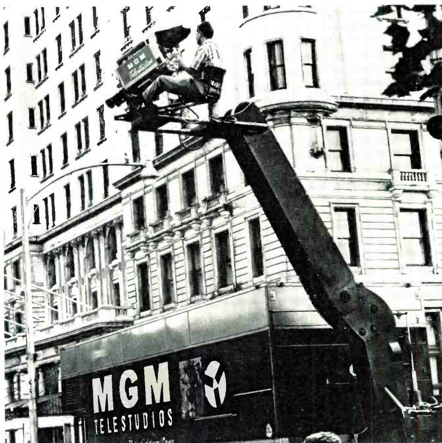
TK-60 camera mounted on 22-foot boom gives MGM Telestudios new mobile tape unit wide versatility, while below nine-month-old Leo shows you what a hard day at the viewfinder does for a lion.
