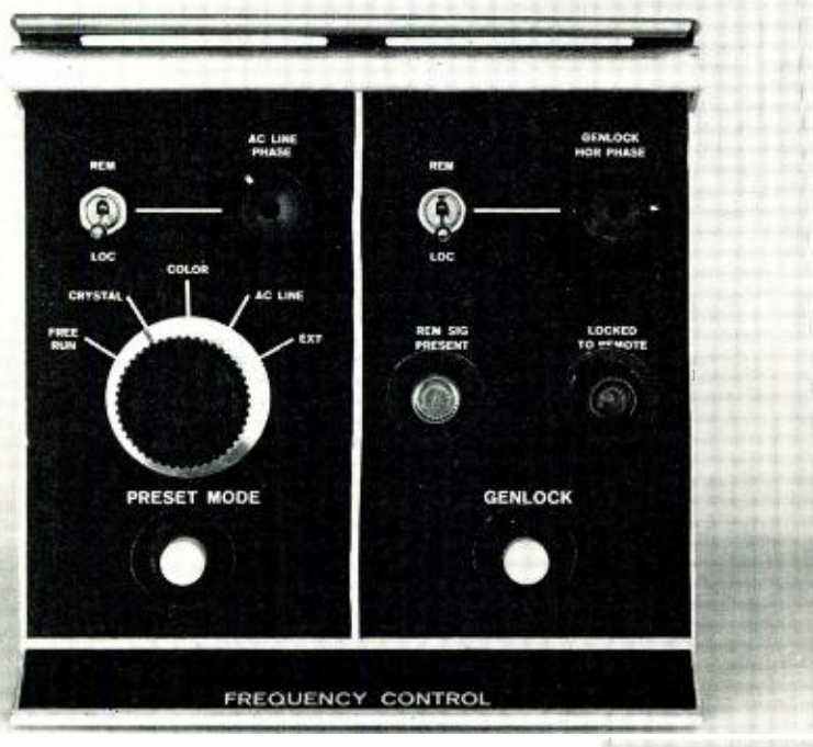
FIG. 5. Frequency Control Module Control Panel, showing six modes of control: 1. Free Run, 2. Crystal, 3. Color, 4. AC Line, 5. External, and 6. Genlock.
