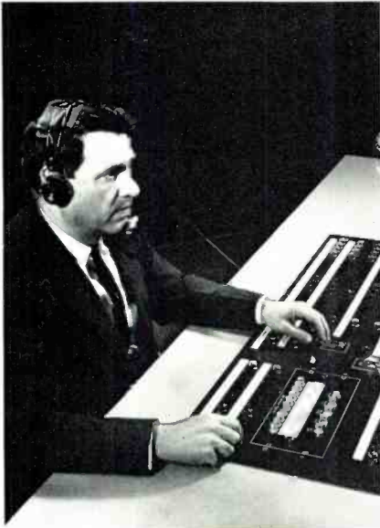
MASTER SWITCHER. This single TS-40 video switching system handles all program switching requirements. It is fully equipped for a multitude of electronic special effects.
