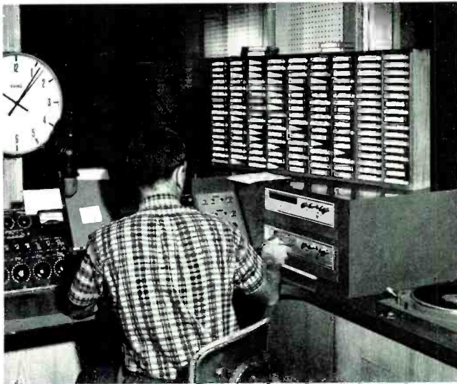
PRIME USE OF CARTRIDGE TAPE is demonstrated by its location here in the radio control room. Note that playback equipment and cartridge storage get position of prominence at the right of the operator-announcer. This AM control room overlooks tv studio B which is equipped to handle orchestral, choral and audience participation-type radio programs.
