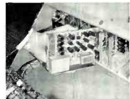
Plug-in flexibility... preamplifiers for low-level sources... isolation/balancing units for high level sources.
