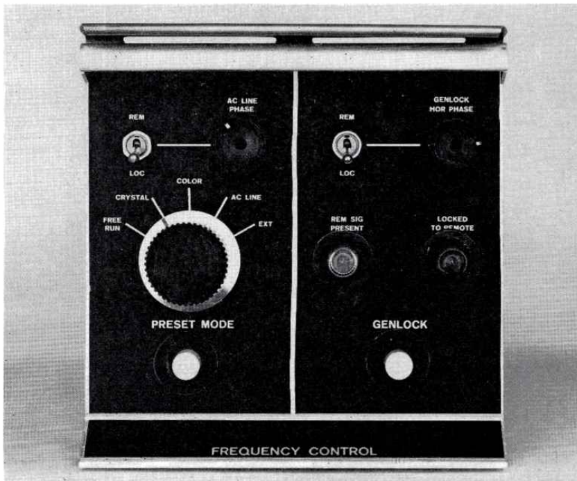
FIG. 5. Frequency Control Module Control Panel, showing six modes of control: 1. Free Run, 2. Crystal, 3. Color, 4. AC Line, 5. External, and 6. Genlock.
