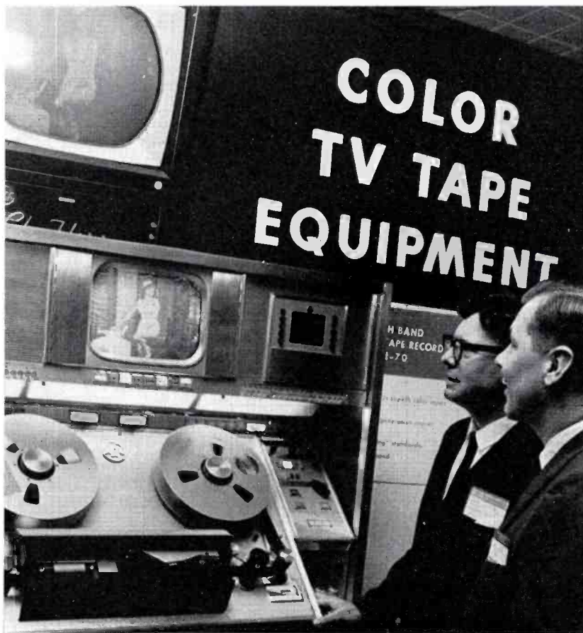
High-level color TV tape performance attained with high-band equipment was exemplified by the TR-70, shown for the first time.
