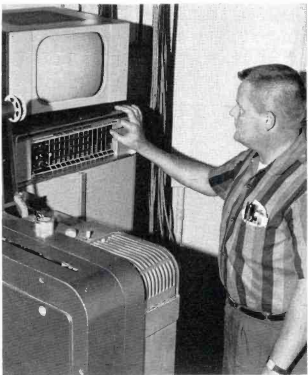
FIG. 4. One of two TK-27 color film chains complementing WLBW-TV's new RCA matched Color TV equipment.
