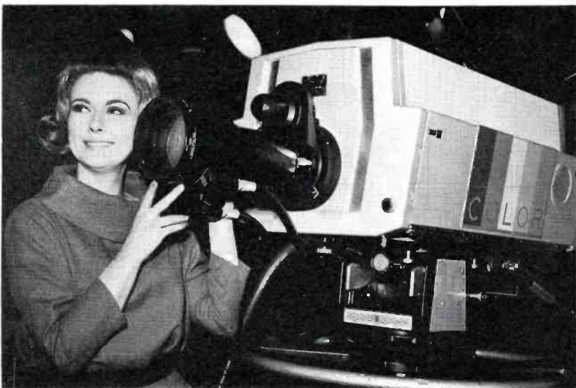
External zoom lens distinguishes the TK-43, newest four-tube color camera in RCA line.
