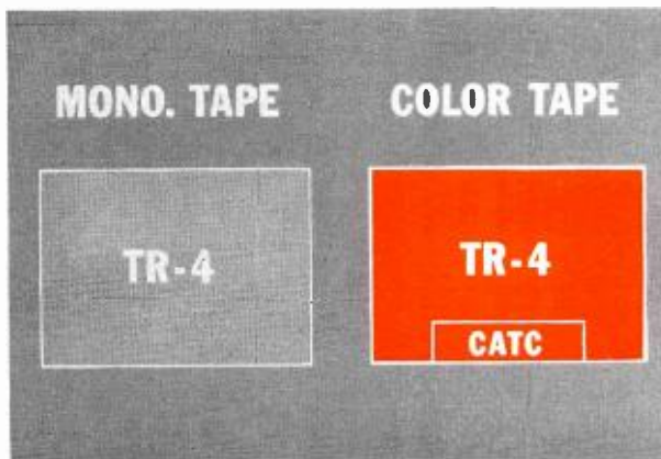
FIG. 22. Modifying tape equipment for color.
