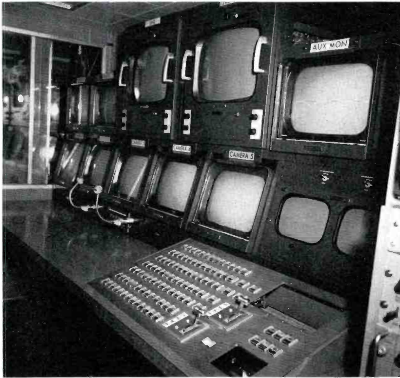
FIG. 6. The video control section features two color, ten black and white monitors, and the TS-40 switching equipment. To the right is the technical producer's position.
