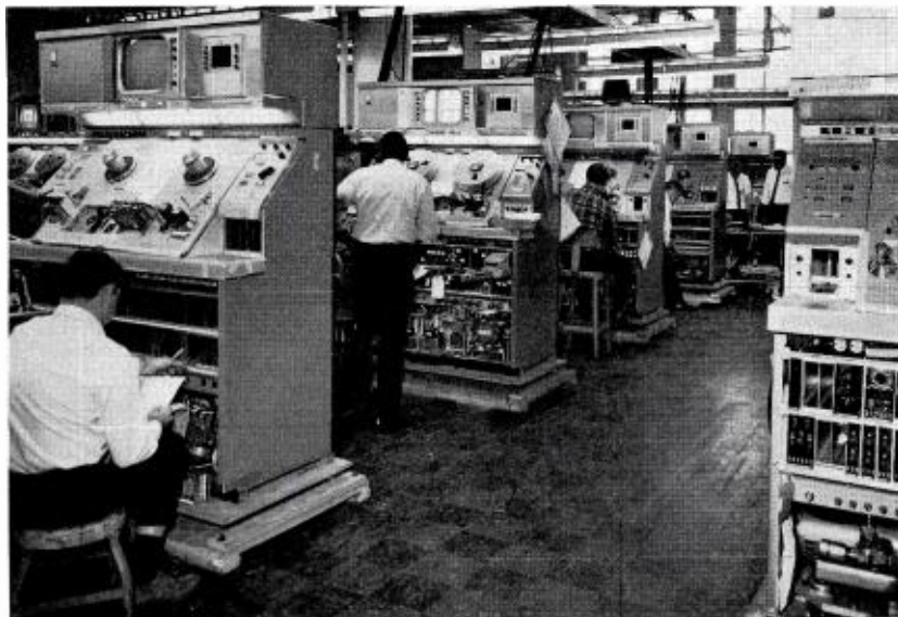
In busy test area, TR-70s get rigorous 240-hour check before delivery to broadcasters.
