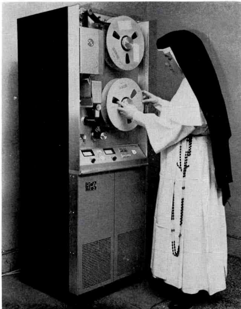
FIG. 7. Archdiocese of New York System employs RCA TR-3 TV Tape Player for presenting programs that are recorded on video tape.
