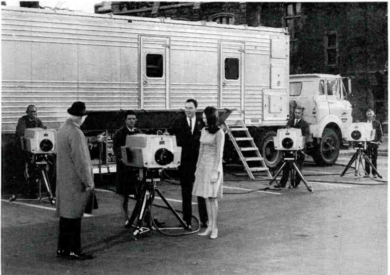
FIG. 2. One of the RCA Victor equipped vans, with four TK-42 cameras, and complete production facilities, at Westmount Park in Montreal.
