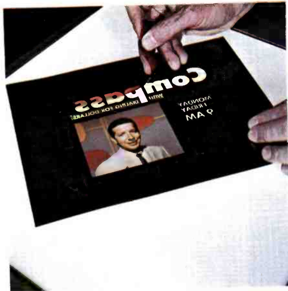
FIG. 8. Placing the Cinemoid material on the reverse side of the negative.
