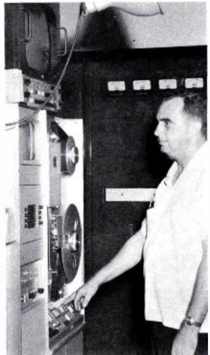
FIG. 7. KHVH-TV Chief Engineer Dan Hunter checking over RCA TR-4 color VTR machine.
