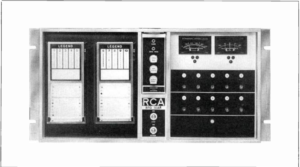
FIG. 24. RCA Type BTG Automatic Logging Equipment. Six systems are available providing local or remote logging of up to 20 functions.
