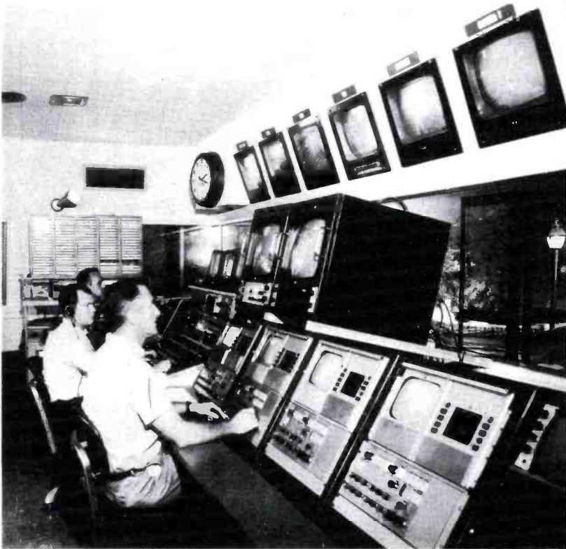
FIG. 2. Station-built master console using TS-40 Transistorized Switcher and "New Look" live and film camera controls.
