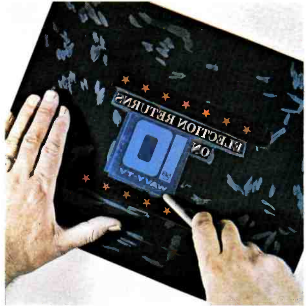
FIG. 3. Example of how color is stripped on the reverse side of the negative.
