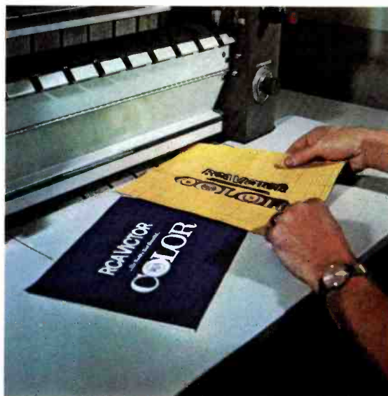
FIG. 15. Tecnifax color sheet being run through the Ozalid.
