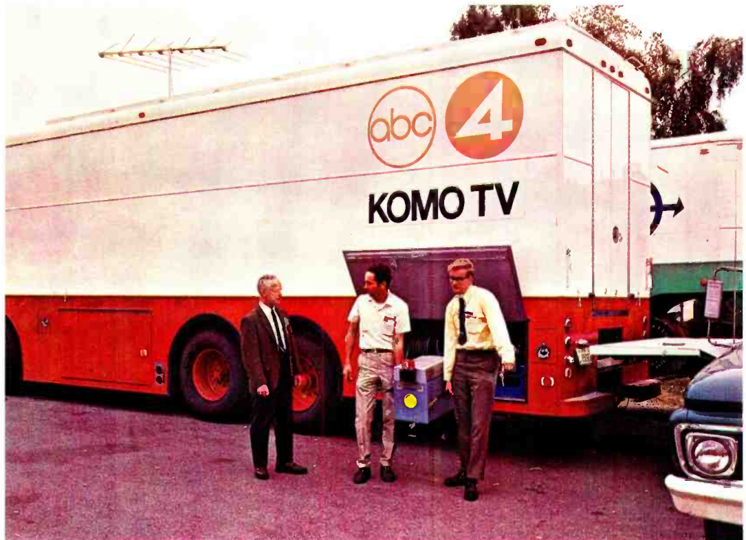
Left to right, Ralph Mifflin, Wally Schutter, and John Carlbom carrying one of the RCA TK-44A cameras by means of convenient fold-out handles located on either side. The truck skirt compartment in the background houses two power driven camera cable reels as does the compartment directly forward of the truck rear wheels. A similar compartment on the opposite side contains shock mounts for six TK-44A cameras.
