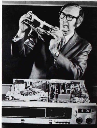
The precision tape transport component of a new magnetic tape home TV player-recorder which RCA plans to market to consumers by late 1973.
