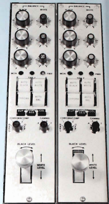
5. Pair of remote control panels for TK-28.
