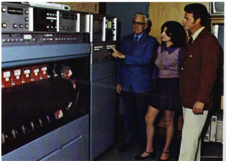
"Cart" machine at WPTV enables station to schedule additional tape syndicated shows while retaining reel-to-reel capability for commercial production.
