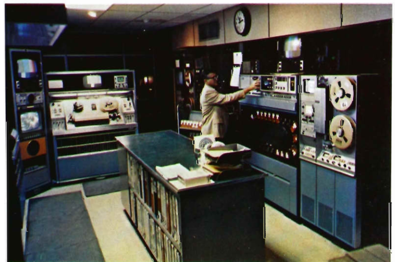
In the WISN-TV tape room, the "Cart" handles the bulk of on-air tape plays, freeing reel-to-reel machines for production.
