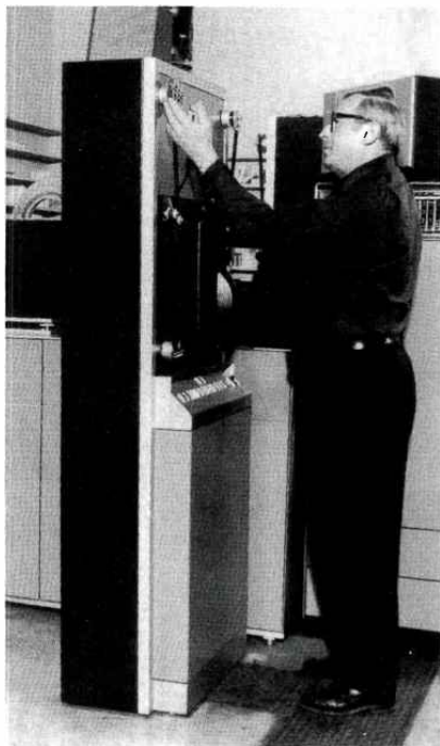
Putting together a spot involving dealer tags has been greatly simplified with the TCR-100. In the picture sequence above, the "cart" machine is set up for recording; the spot film commercial and the dealer copy slide have been loaded on the film island. The film spot is dubbed to the cart, then the dealer ID slide, along with appropriate audio. Recording a spot takes only 2 or 3 minutes at WTVC.
