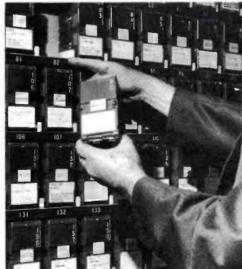
An advantage of large size engraved number is easy identification of all "carts" in machine. Number is clearly visible even when cartridge is in the "play" mode.
