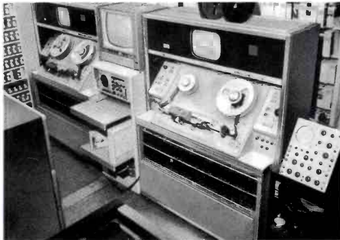
With the TCR-100 handling the break traffic, KCEN is able to get more effective utilization of its studio, tape and film equipment. The "cart machine" provides extra flexibility and capacity to take advantage of more production and commercial opportunities.
