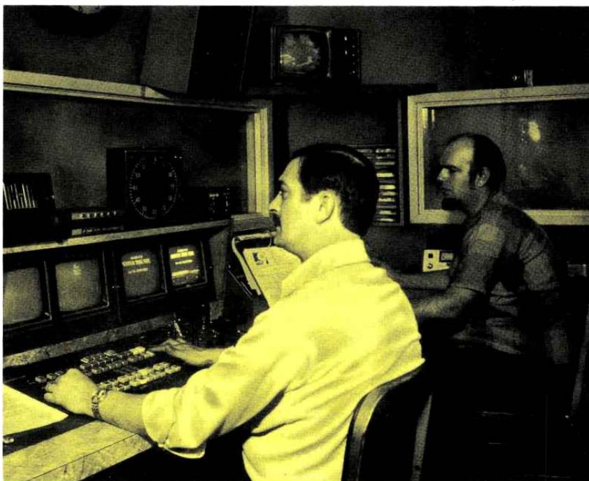
Putting together a spot involving dealer tags has been greatly simplified with the TCR-100. In the picture sequence above, the "cart" machine is set up for recording; the spot film commercial and the dealer copy slide have been loaded on the film island. The film spot is dubbed to the cart, then the dealer ID slide, along with appropriate audio. Recording a spot takes only 2 or 3 minutes at WTVC.
