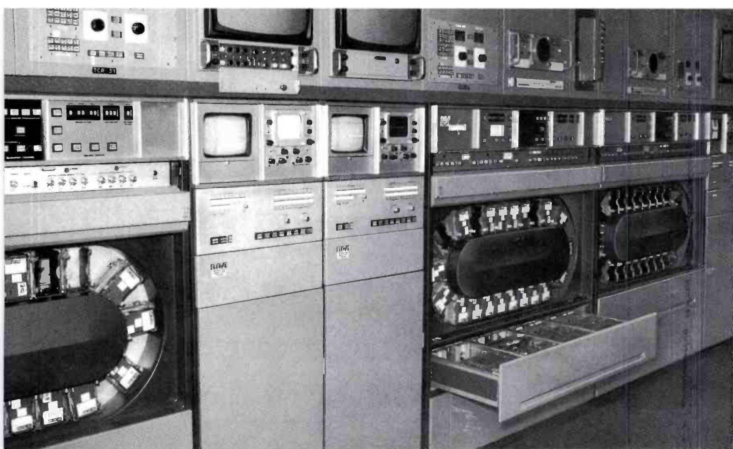
Three of the four "cart" machines on duty at NBC, New York. 96% of NBC network and WNBC local tape commercials are played on these machines. The TCR-100's are handling more than 400 plays per day.
