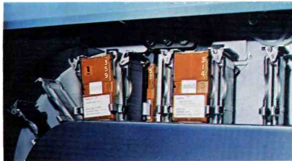
An advantage of large size engraved number is easy identification of all "carts" in machine. Number is clearly visible even when cartridge is in the "play" mode.
