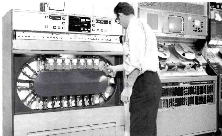
A popular and economical option is the TCR-100 "slaved" to the TR-60 reel-to-reel recorder. The "master" TR-60 time-shares its electronics with the TCR-100. The TR-60 can record while the TCR-100 is playing back and vice versa.
