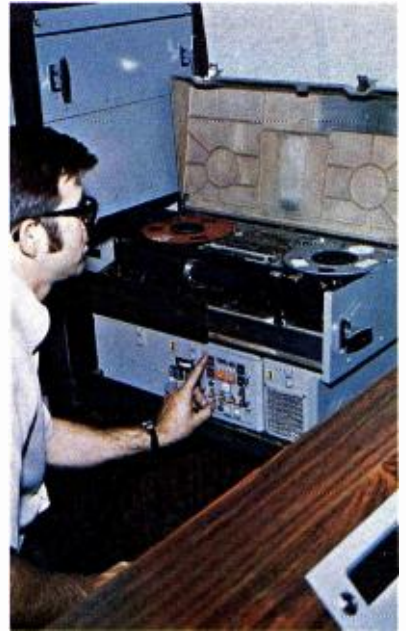
TPR-10 quad VTR's are drawer-mounted in van in front of video switching position.
