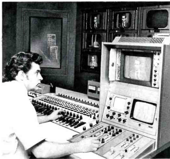
Director, left, calls on special effects of TS-51 System 14 Video Switcher. Four bus unit has two bus panels assigned to mix and effects and two for preset/preview and program. Engineer, right, operates joystick control for #2 studio camera while also keeping a hand on the audio fader controls. The BC-100, with 18 mike inputs and 2 channels out, is an audio-follow-video system that works especially well in quick-turnaround news shows and in cuts between local and remotes on network productions.
