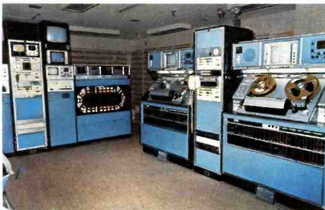
Two TCR-100A cartridge tape machines provide the flexibility needed for production and for on-air playback of "cart" commercials.
