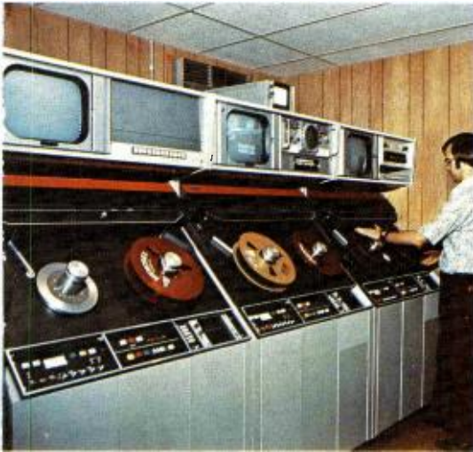
Three TR-600's handle a heavy video tape load, including recording, editing and dubbing.
