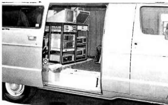
Main compartment of the van includes rack-mounted camera controls and VTR's.
