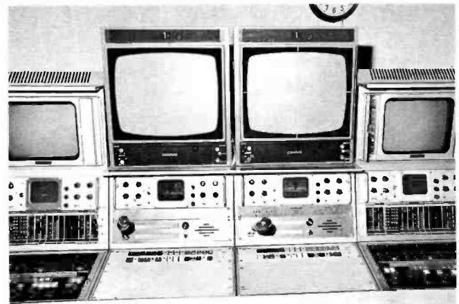
Video Control is set up with two Technical Preview positions with Master-Match monitors. This permits the use of both studios for independent, simultaneous productions.
