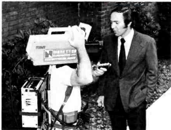
One-man News Team. WBRE-TV has a long-standing record of adopting and adapting innovative broadcast products. The Wilkes-Barre station was among the first to install the TCR-100 video cartridge tape recorder and the TCP-1624 cartridge film system. The TK-76 was a natural addition, but TV-28 added a different touch: teaming the TK-76 with a back-packed cassette recorder to permit news coverage by one man if necessary.
