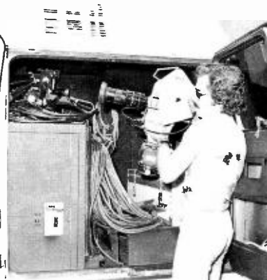
Rear compartment of van is crammed full, storing the TKP-45 camera head, 600 feet of camera cable and a miscellany of other accessory equipment.
