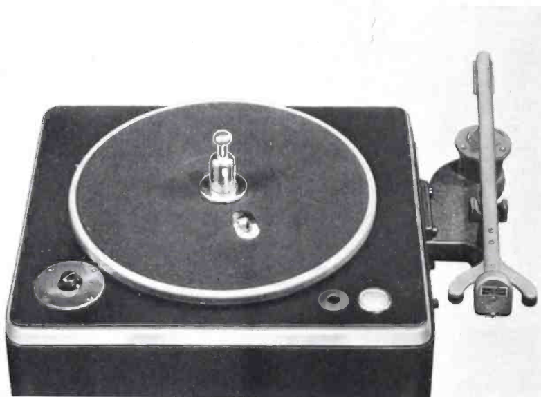
TOP VIEW OF THE NEW RCA VICTOR TYPE 70-A CONSOLE, SHOWING THE TURNTABLE, SUSPENSION ARM, PICKUP, AND SELECTOR SWITCHES. THE SPEED SHIFT BUTTON IS LOCATED ON THE TURNTABLE DISC ITSELF. THE VERTICAL PICKUP TYPE 71-A IS NOT SHOWN
