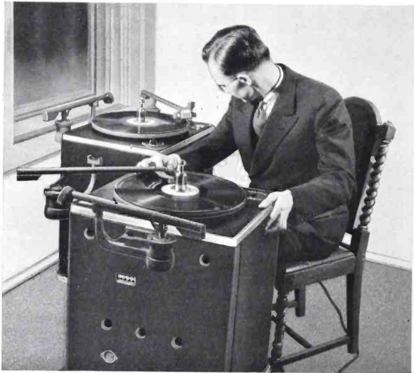
THE NEW RCA VICTOR "DELUXE" TRANSCRIPTION TURNTABLE EQUIPMENT IS COMPACT AND IS DESIGNED WITH A VIEW TOWARD OPERATING CONVENIENCE. WITH TWO OF THESE UNITS, AN UNINTERRUPTED PROGRAM MAY BE RUN FROM ELECTRICAL TRANSCRIPTIONS EITHER AT 33-1/3 R.P.M. OR 78 R.P.M. SPEEDS, AND WITH EITHER VERTICAL OR LATERAL TYPE RECORDINGS
