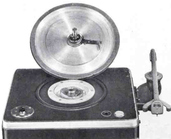
THIS VIEW SHOWS THE TURNTABLE DISC TURNED OVER TO DISCLOSE THE INGENIOUS BALL-BEARING SPEED REDUCTION MECHANISM. THE PAWL ON THE BOTTOM OF THE DISC ENGAGES THE SLOT IN THE CLUTCH RING WHEN 33- \frac{1}{3} R.P.M. OPERATION IS DESIRED
