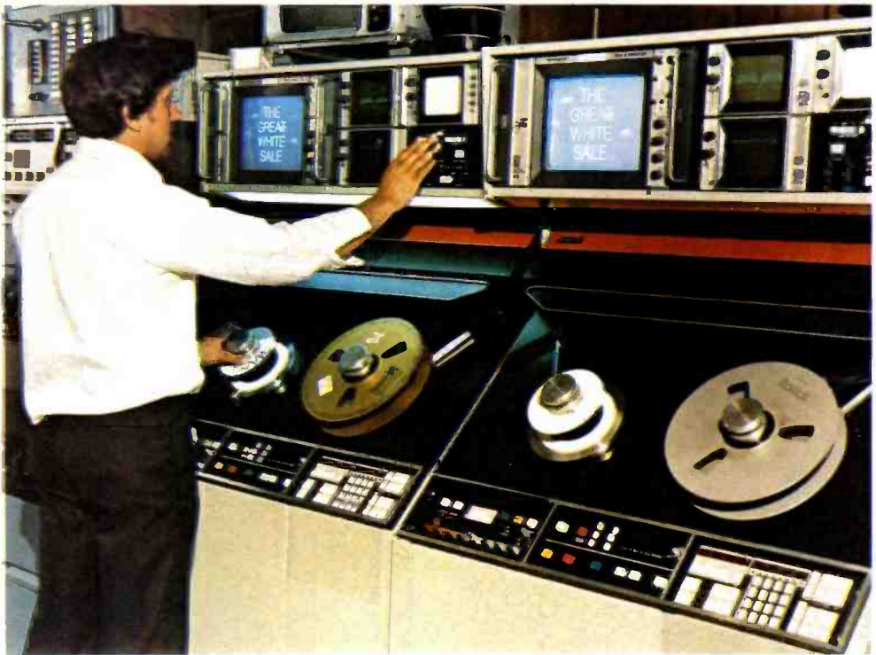
Two TR-600A quad tape machines with AE-600 Time Code Editing Systems are used for program playback, production and editing.
