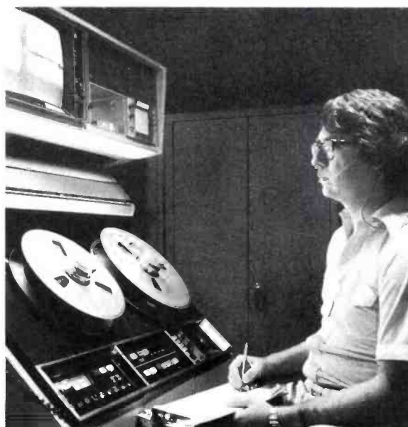
Used in high-band mode at 2X speed, a TR-600 rolls with a pre-recorded movie.
