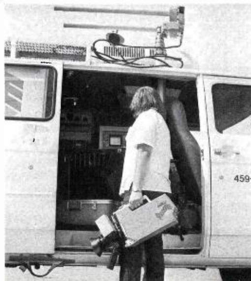
ENG unit, TK-76, and cameraman unload for a local, live pick-up. The telescoping Nurd antenna allows quick signal alignment.
