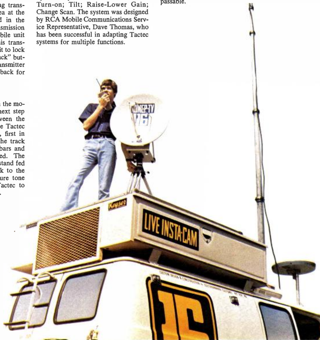
Unit #1 with mini-link relay. Stu Wilson uses RCA Tactec portable radio to expedite microwave alignment.
