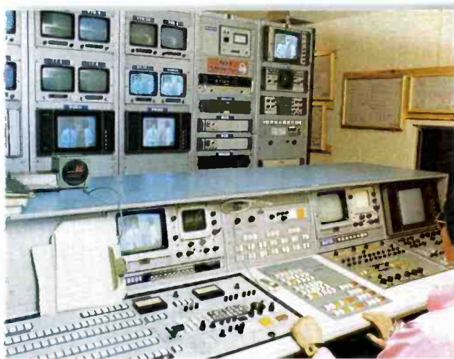
Master Control can also be used for Production when needed. Complete functional diagrams for technical system are framed on wall at right for ready reference.
