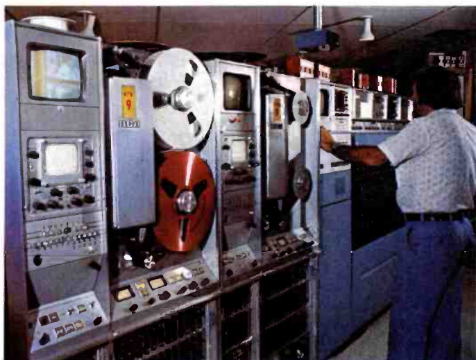
TCR-100 and tape machines were moved from the old facility. Everything but news and special films is dubbed to "cart" for playback. TCR is used for production as well as for airing commercials.
