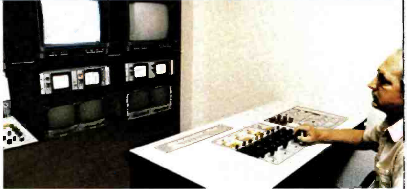
Hal Smeder employs one of the TK-47 RCUS to fine tune a camera.
