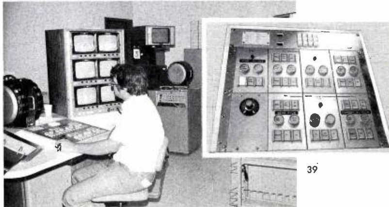
KMTV-designed remote telecine machine panel (inset) and bank of monitors aid in production and on-air operations.
