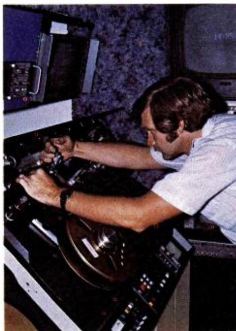
Jim Taylor makes a headwheel adjustment on a TR-600 VTR.
