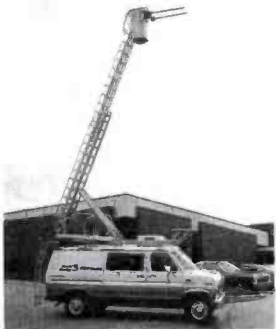
The KMTV ENG complement includes a microwave-equipped van for extended distance direct transmission to the studio.
