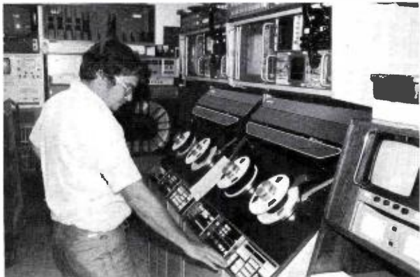
Tape production is handled by TR-600A VTR's equipped with AE-600 Time Code Editing Systems.
