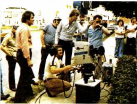
TK-760 rides comfortably on short mount, with a viewing receiver as a base.
