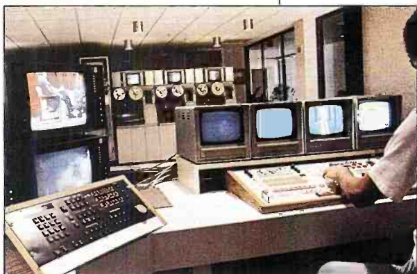
One-inch Post Production Suite with AE-800 Time Code Editing system and video switcher, looks directly into Master Control, with TR-800 VTRs in background.
