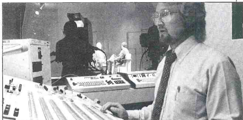
The Director Control Room, with machine controls, Production Switcher and graphics facilities, provides a direct view into Studio A.
