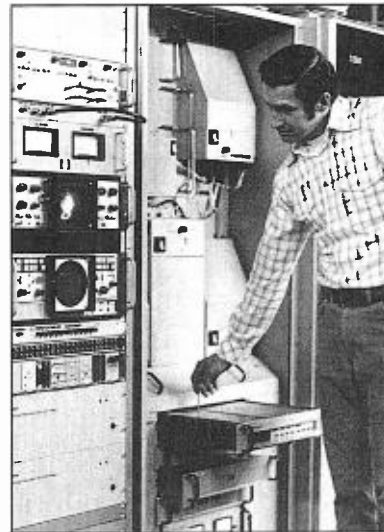
Engineer Alroy Kessler makes an adjustment, using video test rack conveniently located between the two TTG-50H Transmitters.
