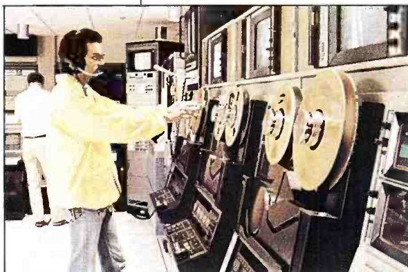
Multi-format tape facility includes TR-800 one-inch VTRs, quad machines and videocassette units.
