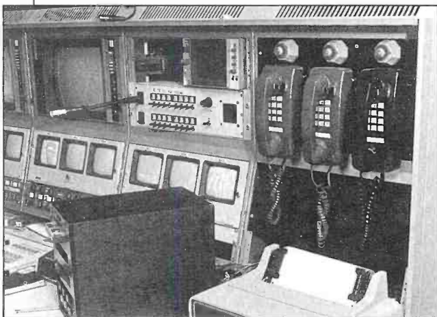
Hard copy printout used with Multi-cassette playback system provides positive identification of each commercial, its duration and time of airing.
