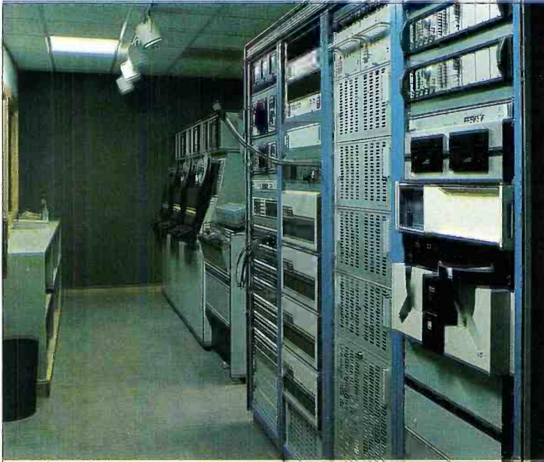
Three TR-800s share space outside the EPIC I Editing Suite with extensive video and audio distribution and terminal facilities.
