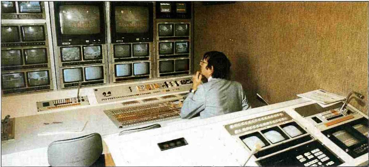
Production control in the QVLV truck features a Grass Valley 300-3A video switcher with five isolated banks and a Chyron IV graphics system.
