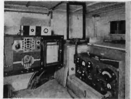
FIG. 12. The TMV-75-B-equipped station wagon of Edwards and Martin, Consultants. The equipment is arranged as in Fig. 9c—that is, the recorder is driven from a receiver-amplifier combination, the field intensity meter being used for calibrating purposes only. This provides flexibility and allows the meter to be used for measurements outside of the car.
