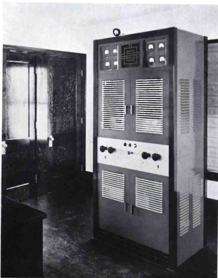
The new RCA ET-4250 Transmitter which steps up power for WRAK.
