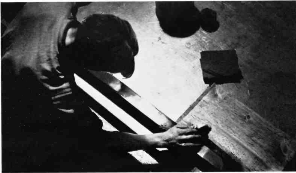
41. Finishing side strips. Careful attention to details, hand rubbing of panels and style strips and improved lacquers assure a pleasing appearance of the equipment.
