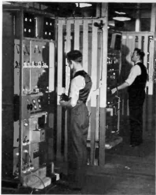
27. Individual test booths with separate measuring equipment permit several transmitters to be tested at once.
