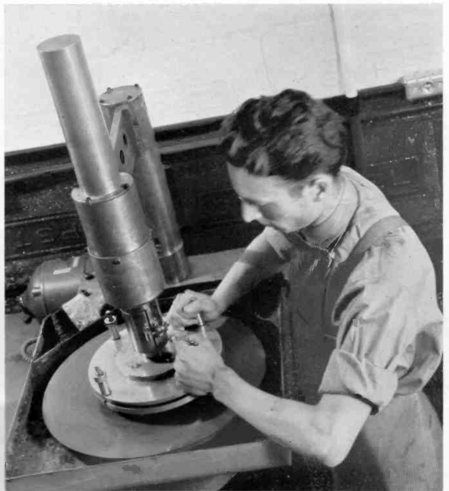
34. Grinding of blanks is carried out on special machines by trained workers.
