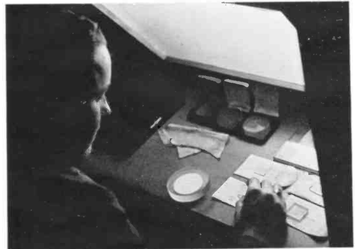
38. Interference patterns made by light falling on the lapped crystal as it rests against an optical "flat" assure flat plates.
