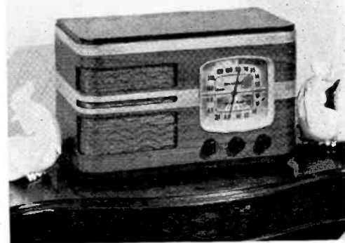
▲ Model 85T1... a smartly fashioned little chest model that will give you entertainment from all over the world. New type dial simplifies tuning and enhances appearance. Cabinet reveals new and modern uses of fine, rare woods. A 2-band, 5-tube superheterodyne of fine volume and tone. Dynamic speaker, automatic volume control.
