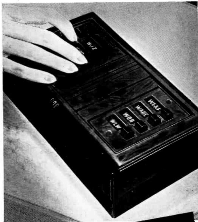
▲ Model 85T1... a smartly fashioned little chest model that will give you entertainment from all over the world. New type dial simplifies tuning and enhances appearance. Cabinet reveals new and modern uses of fine, rare woods. A 2-band, 5-tube superheterodyne of fine volume and tone. Dynamic speaker, automatic volume control.
