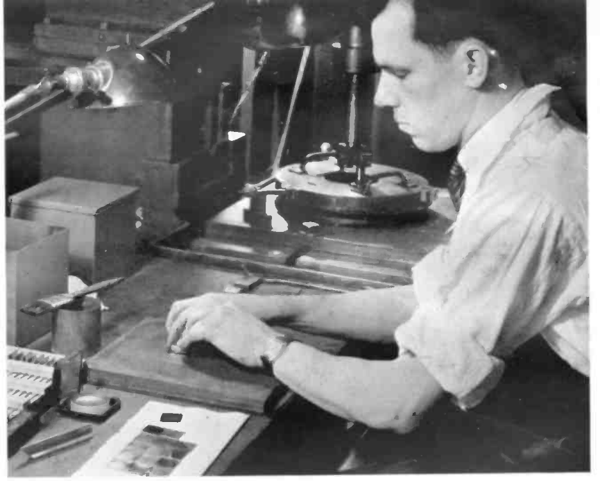
36. Holders must be carefully built. Metal electrodes are carefully lapped and polished to optically flat, uniform surfaces.
