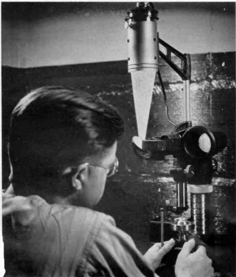
33. Thickness gauges indicating ten-thousandths of an inch aid in preparation of the quartz for final lapping.
