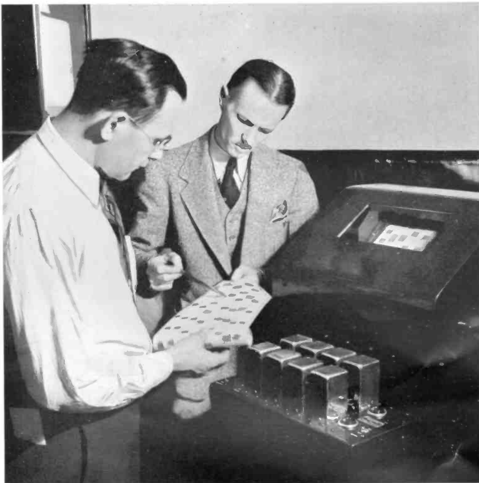
40. Testing thermostats. This machine marks on a roll of paper whenever the heat is applied to the crystal oven. Eight heater units are tested simultaneously.
