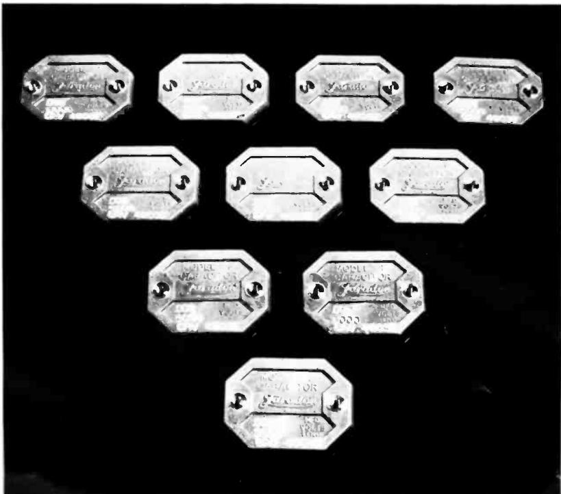
18. Other components manufactured in RCA'S plant begin to arrive in the factory awaiting assembly. Faradon condensers, built by RCA and used generally in all
