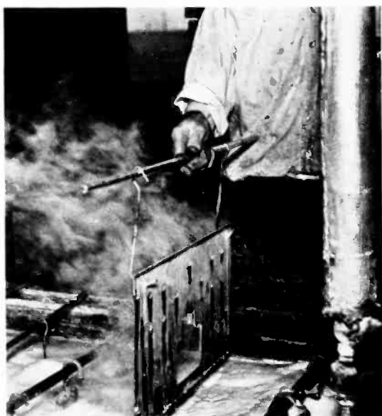
14. Rust protection is important. Frames, metal panels, shields, all are rust-proofed before applying final finish. Here in the copper plating shop, components are receiving a protective coating.
