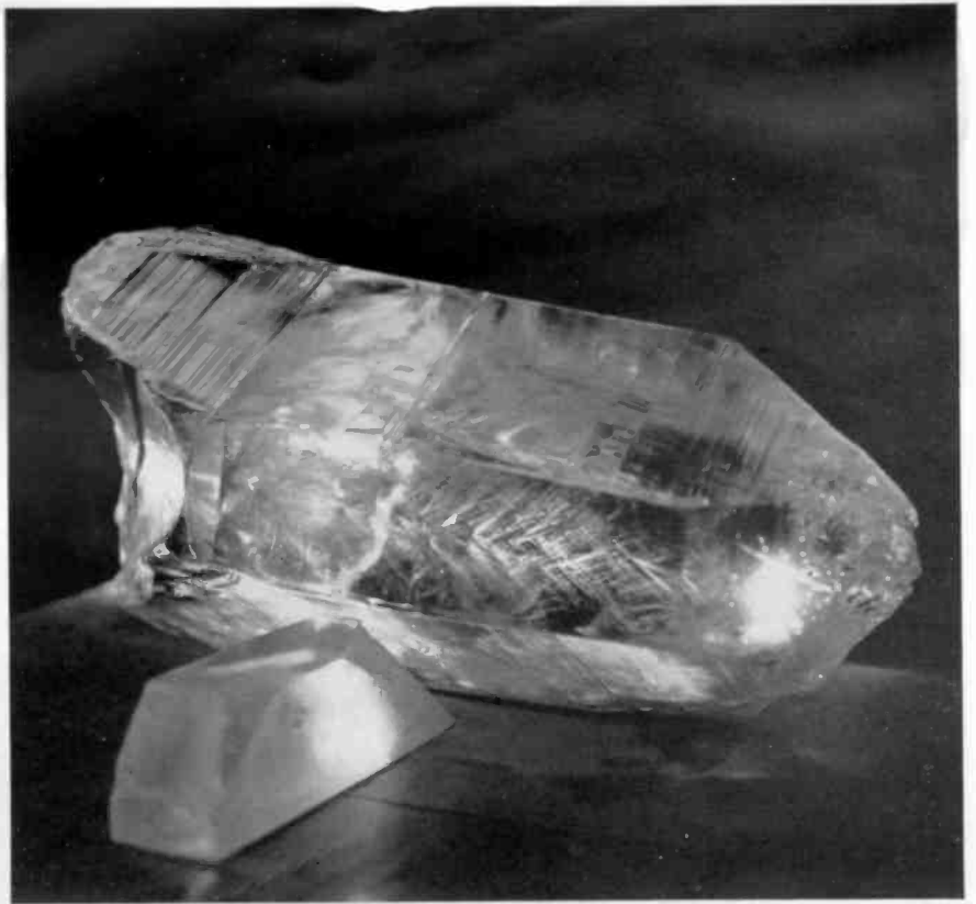
32. The mother crystal shown exhibits "needling," which makes it unsuitable to meet RCA's specifications.
