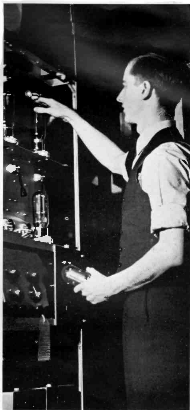
29. Transmitters are tested with actual tubes from stock, not selected tubes. Final measurements are made using the tubes sold with the transmitter.
