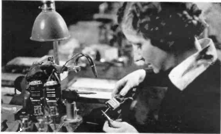
Inserting a heater cathode in the element assembly of an RCA 837. Great care is exerted in applying the active material to the cathode surface to retain exactness of the coated area and thickness.
