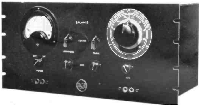
69-A Audio distortion meter measures both hum and distortion over 50 to 7500 cycle range.
