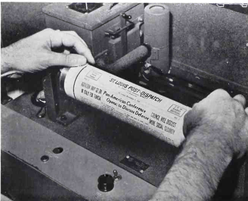
BELOW: Adjusting a page from the St. Louis Post-Dispatch in the scanning unit.
