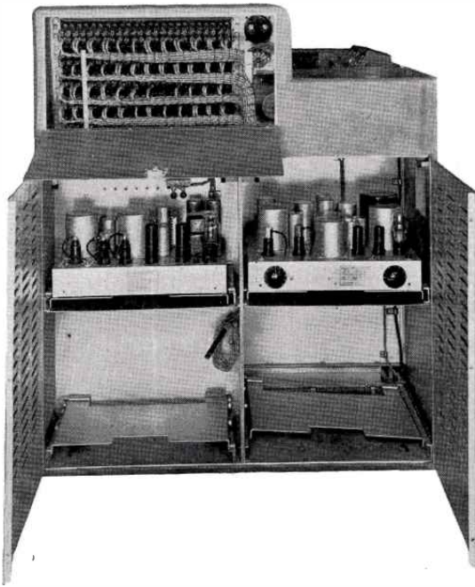
FIG. 4. Monitoring and program amplifiers are mounted on sliding shelves in the right side of the console.
