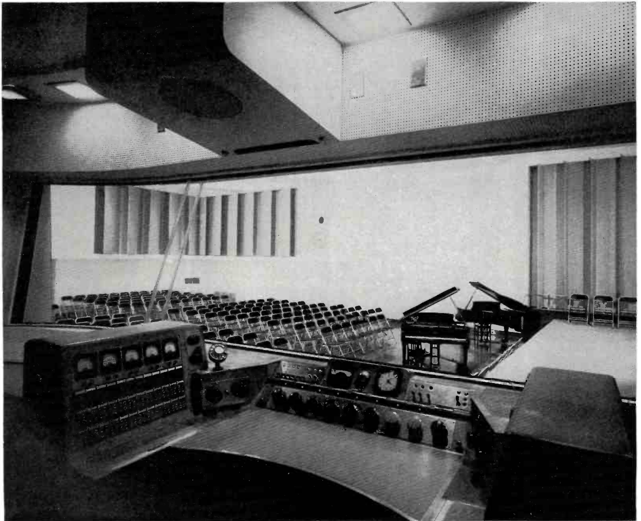
FIG. 3. The 2-A Console in one of the booths at CBS, New York. Note how the low front gives the operator an unobstructed view of the entire studio.
