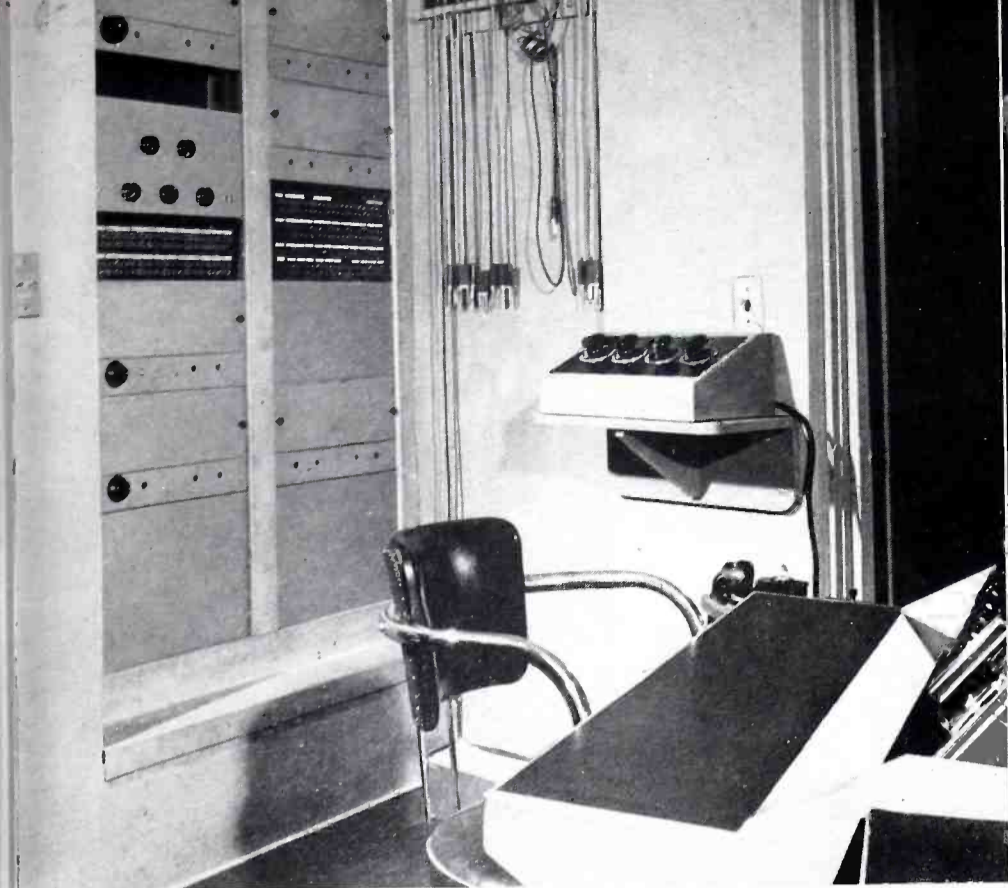
FIG. 7. Audio equipment racks. On the wall shelf is a portable mixer box.
