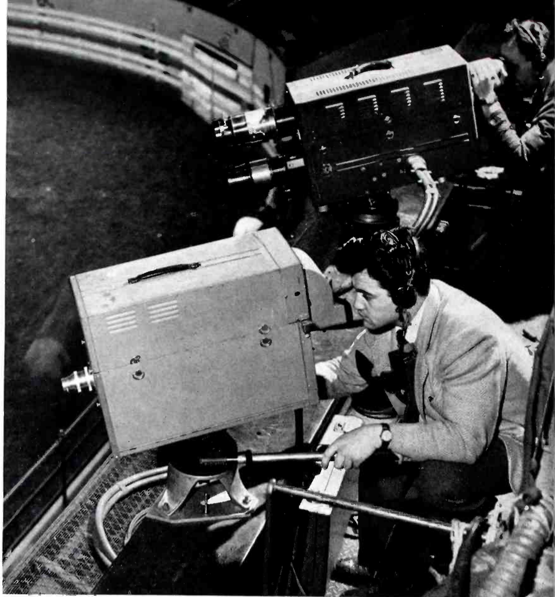
The New High-Sensitivity Camera (foreground) in use at Madison Square Garden. Scenes which could not be picked up with the older field camera (rear) are now seen with perfect clarity.
