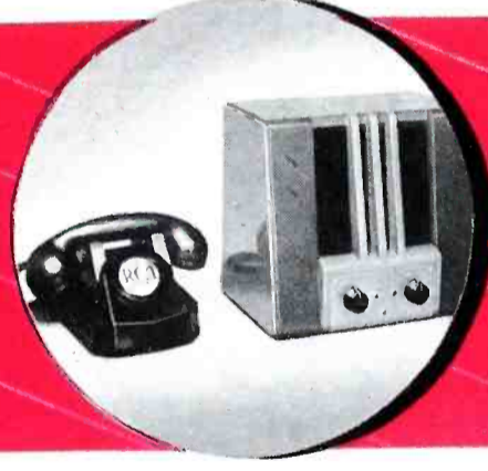
9. Station Handset and Control Unit: Furnished with the FM Station Transmitters shown here. The control unit contains a loudspeaker, plus controls for adjustment of "volume" and "squelch." Also, "transmit," "receive," and "stand-by" signal lights.
