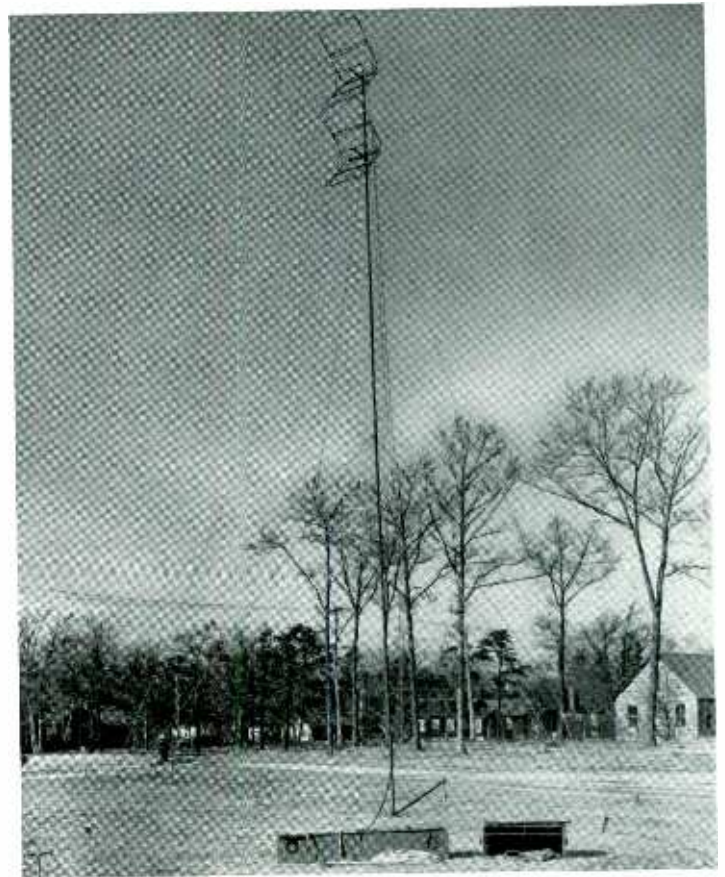
(Above)—Portable antenna system used with the AN/TRC-8 transmitting-receiving equipment designed and built for the Army by RCA.
