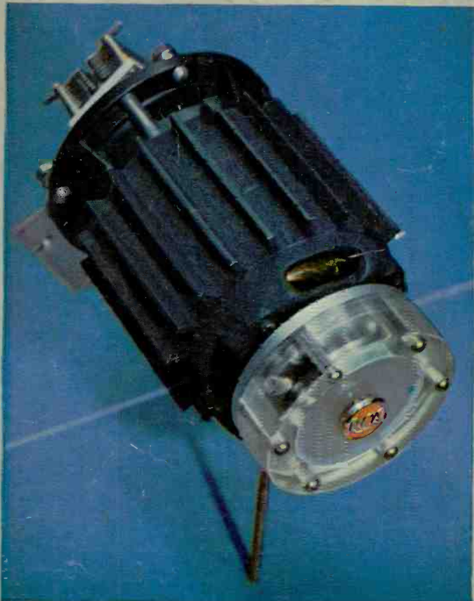
Two-phase induction motor with frequency-compensating condenser mounted directly on shaft. The Lucite cylinder contains the oil-dampening element.
