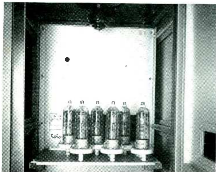
RCA-8008 Rectifier tubes are used in 3 KW and higher powered transmitters.
