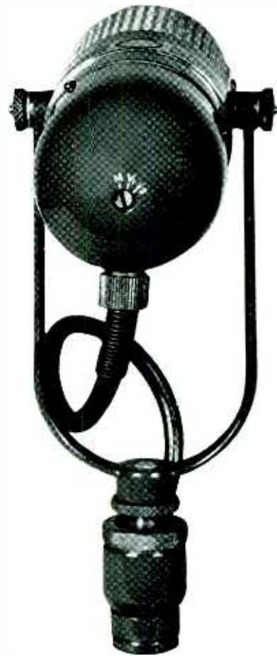
FIG. 8. Bottom view showing voice-music selector switch.
