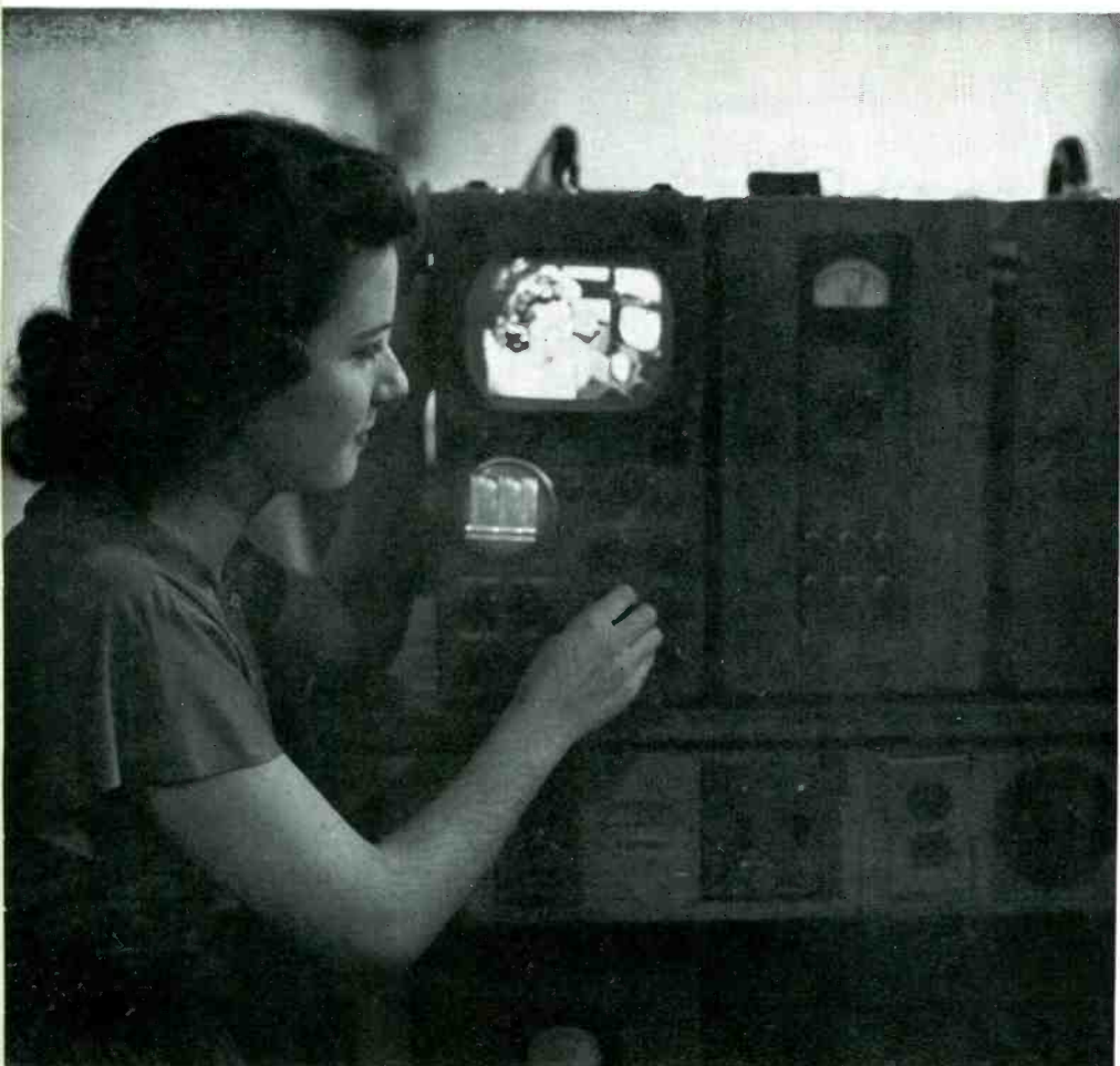
(Left)—In this illustration the girl operating the monitoring unit of the new RCA Field Equipment is looking at her own image on the screen. The only illumination of this scene was light coming over a transom from another room. The light incident on the scene measured 3½ foot-candles.
