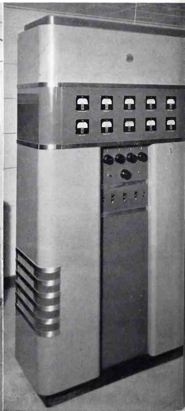
FIG. 2. (below) Llewellyn Jones, Chief Engineer, at the controls of the WSBA 1-kilowatt AM transmitter, RCA Type 1-K.
