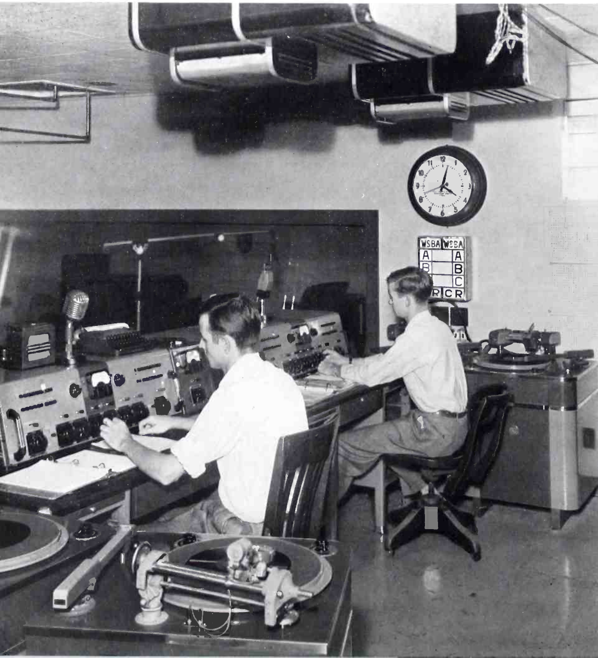
FIG. 1. (below) Complete control of studios and AM transmitter is provided by this flexible arrangement consisting of 76-B2 and 76-B4 Consolettes and 70-C2 Turntables complete with recording attachments. Messrs. Beaver and Lovett, operators, are shown at the master controls which face the AM transmitter.
