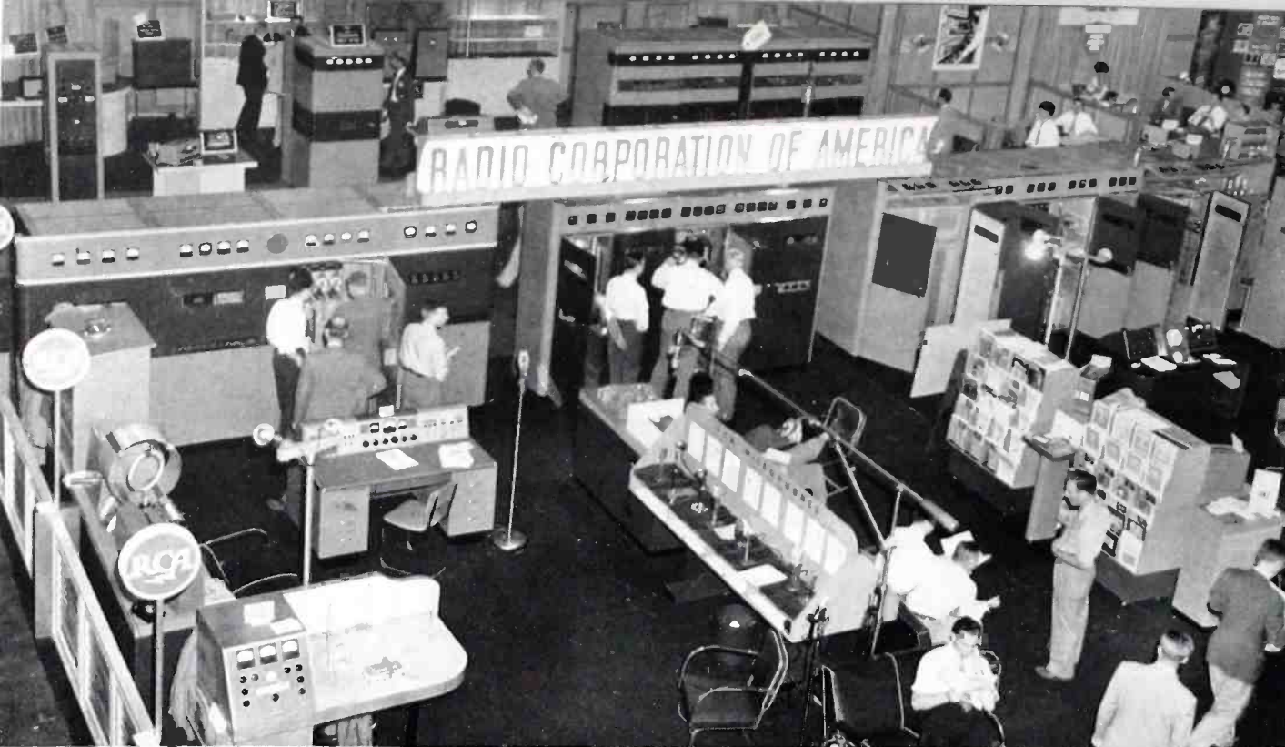
Prominent feature of the RCA booth was this line of transmitters. Left to right, the BTA-5F 5 KW AM Transmitter, the BTF-10B 10 KW FM Transmitter, and the TT-5A 5 KW TV Transmitter.
