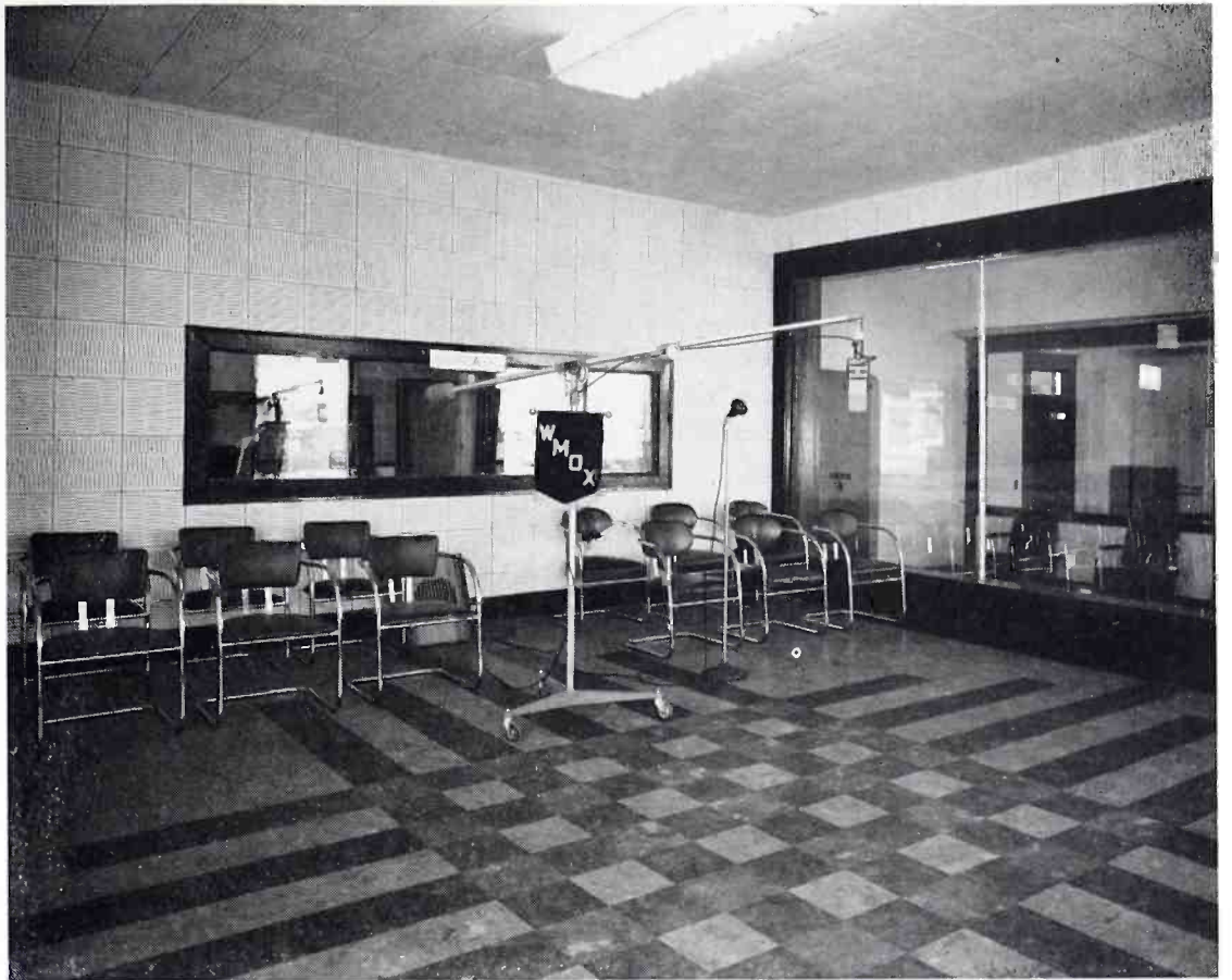
FIG. 2. (Right) A corner of WMOX's Studio A, looking toward the control room. Lobby and offices are to the right. Microphones include an 88-A and 44-BX on a boom stand. WMOX's Studio B, which is not shown, is 25 feet by 30 feet in size and has a skylight which provides an interesting daylight effect. Type 44-BX's are also used in this studio.
