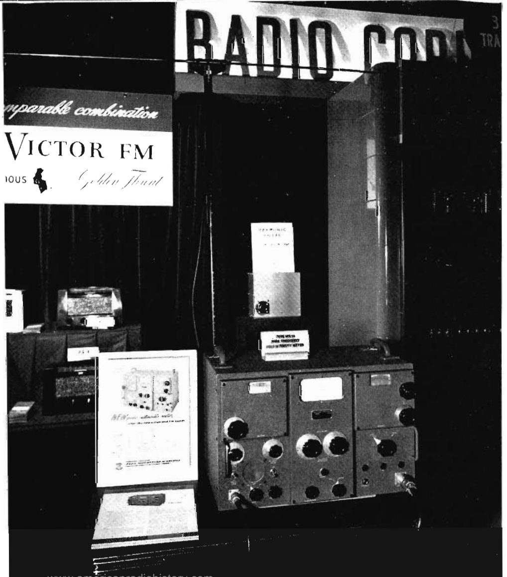
FIG. 3 (Right). The WX-1A Field Intensity Meter for FM and Television frequencies drew much favorable comment.
