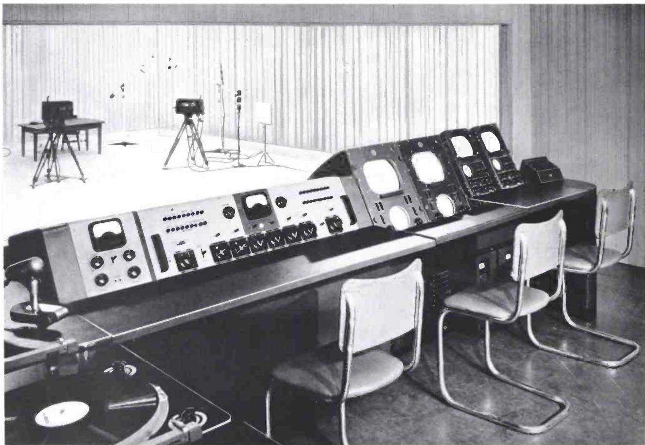
FIG. 16. (Below) Control Room for the Type B Small Station. This equipment layout utilizes the Type TS-10A Camera switching and lap-dissolving system, designed for studio control room use. Video units are identified in the block diagram, opposite page.
