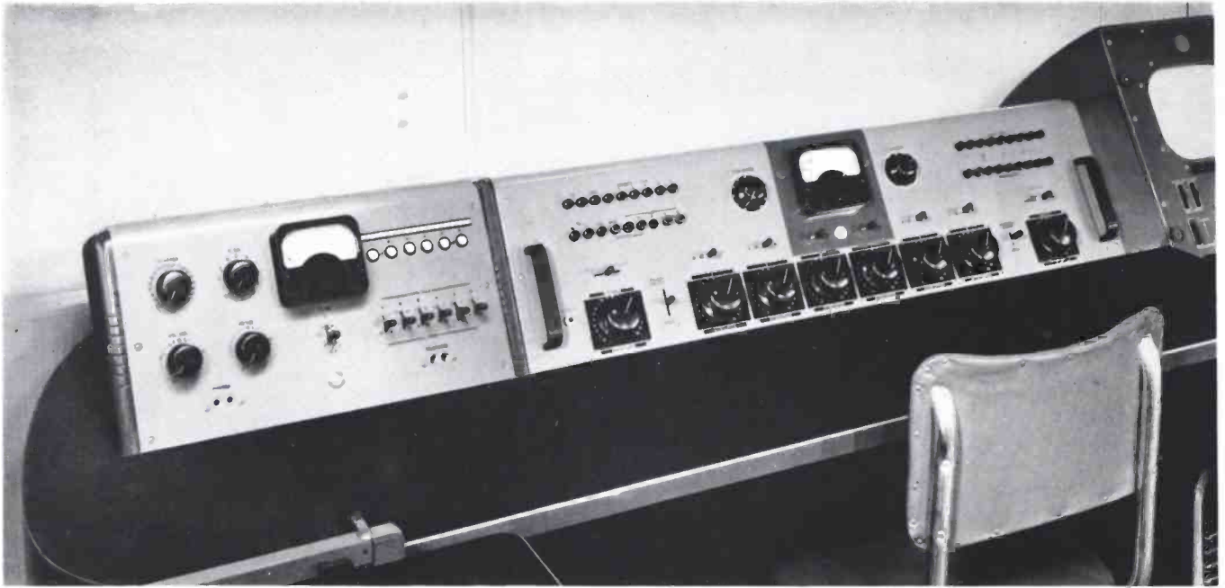
FIG. 36. The audio console above will handle the audio requirements for most television stations. Equipment shown is the Type BCS-3A Auxiliary Switching Unit (smaller unit at left) and the Type 76-TV Console. (Below) Block Diagram of the Audio Control Setup for a Television Station Employing a Single Studio, a Projection Room and Control Room.
