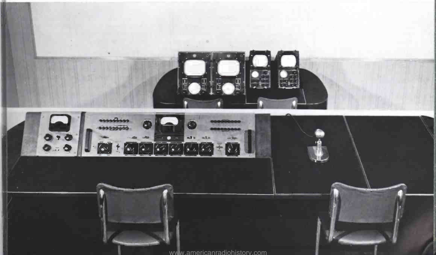
FIG. 24. To provide the director with closer supervision over video switching operations, the TS-10A Camera Switching System can be located on the platform with the audio console, as shown above. Platform setups are possible with any of the equipment layouts described. Photo below shows an arrangement for the Type B station previously described.
