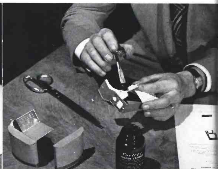
FIG. 7. Apply thin film of rubber cement to BOTH the surfaces to be cemented together. Allow the cement to dry and then press surfaces together firmly. They should form a strong joint immediately.
