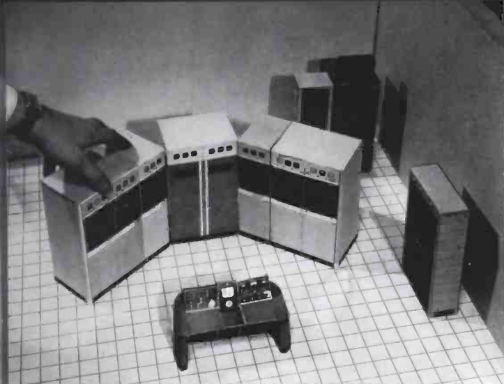
FIG. 10. The models are scaled one inch to the foot. When placed on a card ruled in one inch squares, room dimensions can be determined quickly and easily. Here, the RCA 5 KW transmitter is shown in a "U" arrangement.
