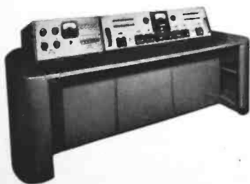
FIG. 6. Television Audio Console. This console is the control center for the audio part of the television program.
