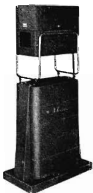
FIG. 2. Type TK-20A Film Camera. This camera converts motion pictures projected from 16mm or 35mm projectors to video signals for television transmission.
