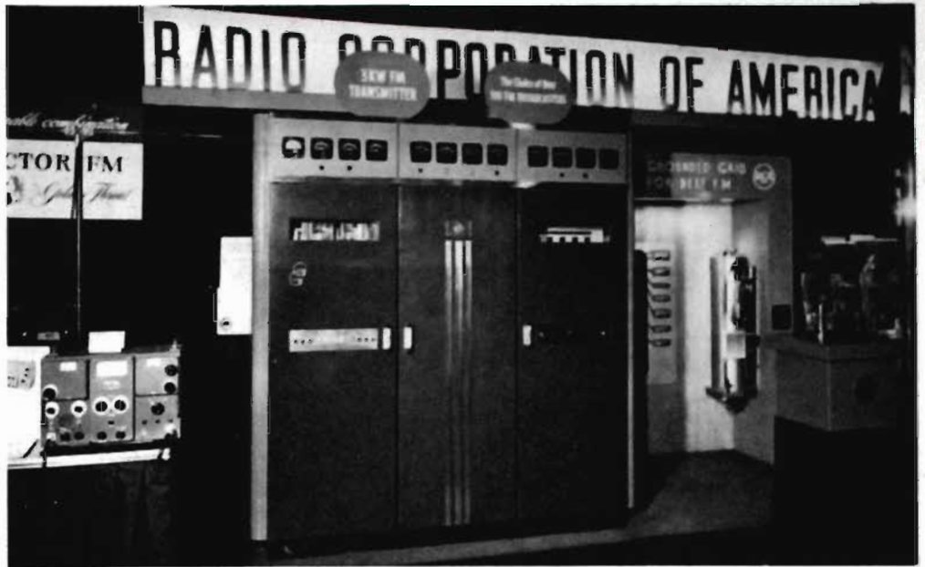
FIG. 4 (Above.) A favorite with FM broadcasters is the RCA 3KW Transmitter, shown above. Behind it, and to the right, is a working display of the well-known Grounded-Grid Tank.
