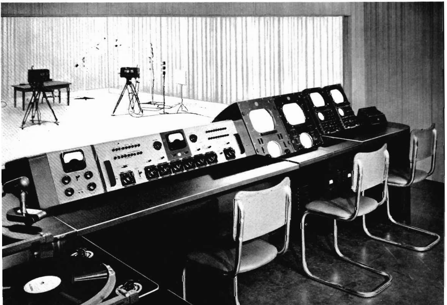
FIG. 16. (Below) Control Room for the Type B Small Station. This equipment layout utilizes the Type TS-10A Camera switching and lap-dissolving system, designed for studio control room use. Video units are identified in the block diagram, opposite page.
