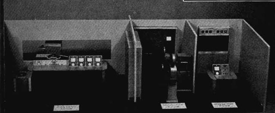
FIG. 13 (left). This model setup simulates a smaller station consisting of a combined studio and master control room, a projection room, and a transmitter room containing a model of the RCA 500-Watt TV Transmitter.
