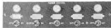
Power Remote Control, MI-26251. Operates up to 5 power supplies through 120-volt relays. Has 5 "on-off" toggle switches and 5 tally lights.
