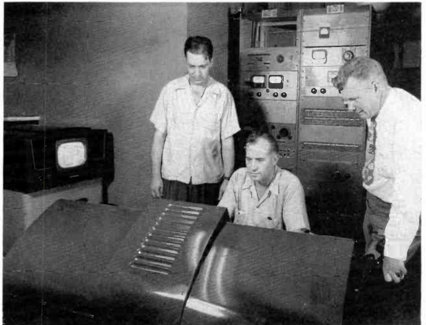
FIG. 12. Audio racks and patching system are conveniently located within reach of the operator. Messrs. Bert Coil, at left, John M. Sherman, at controls, and Paul Clark, RCA Representative, check video picture at different points in transmitter system. Converted RCA TV receiver, at left, is used to monitor microwave relay receiver.
