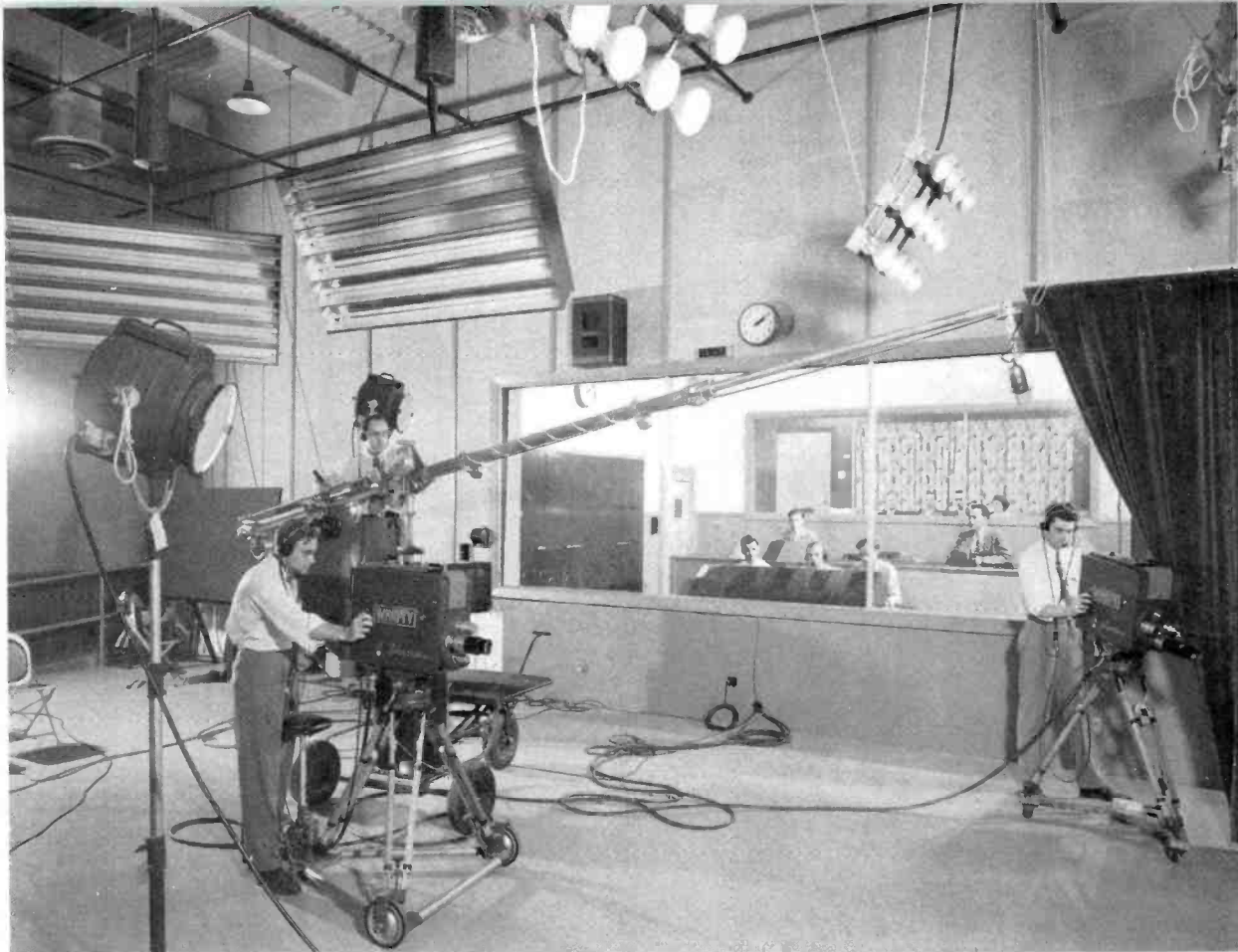
FIG. 9. This view shows the terraced arrangement of the control room and the clients' room as it looks from the studio floor. Access from studio to control room is by means of the ramp shown at extreme left of this picture.
