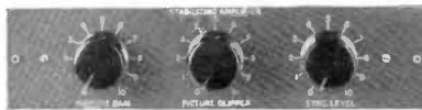
Stabilizing Amplifier Control, MI-26250. Includes three potentiometers. Controls: (1) picture gain; (2) picture clipper; (3) sync level in stabilizing amplifier.
