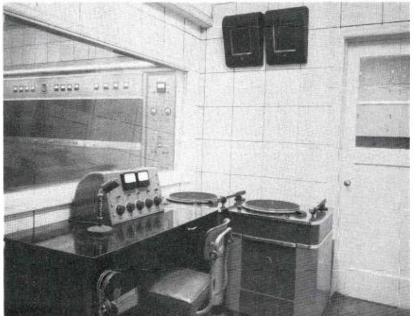
FIG. 4. Interior view of the emergency control room showing the RCA 70-C2 Turntables and station's home-made composite control console for combining or separating AM and FM programs. The 5 KW AM transmitter and one monitor rack can be seen through the window.
