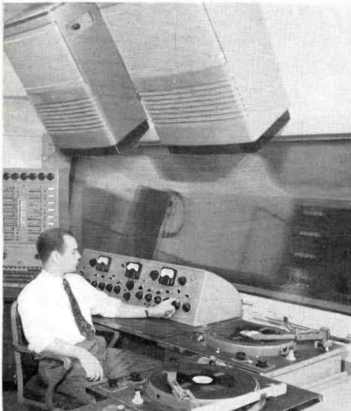
FIG. 14. Broadcast master control position is located on the third floor. Mr. Lee Neuman is shown seated at console built by WTCN. Preset program switching system, behind Newman, was also built by the station. Note bank of RCA LC-1A loudspeakers overhead for checking local and network audio quality.
