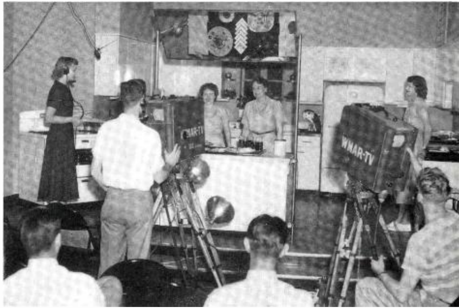
FIG. 4. Field cameras are used to telecast remote cooking demonstration. Note overhead mirror technique used in displaying dishes described.
