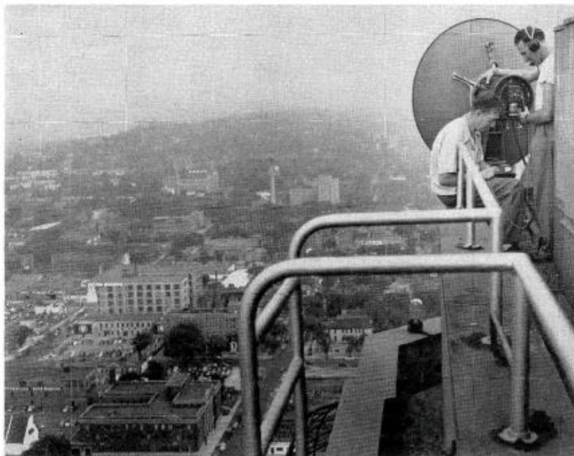
FIG. 2. View from the top of the Foshay Tower Building shows engineers adjusting one of the RCA microwave relay receiver for line-of-sight reception from the Lexington Ballpark across the river in St. Paul.
