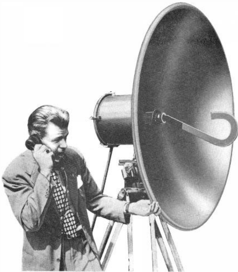
FIG. 1. RCA Microwave Relay Transmitter (TTR-1B) using four-foot parabolic reflector.
