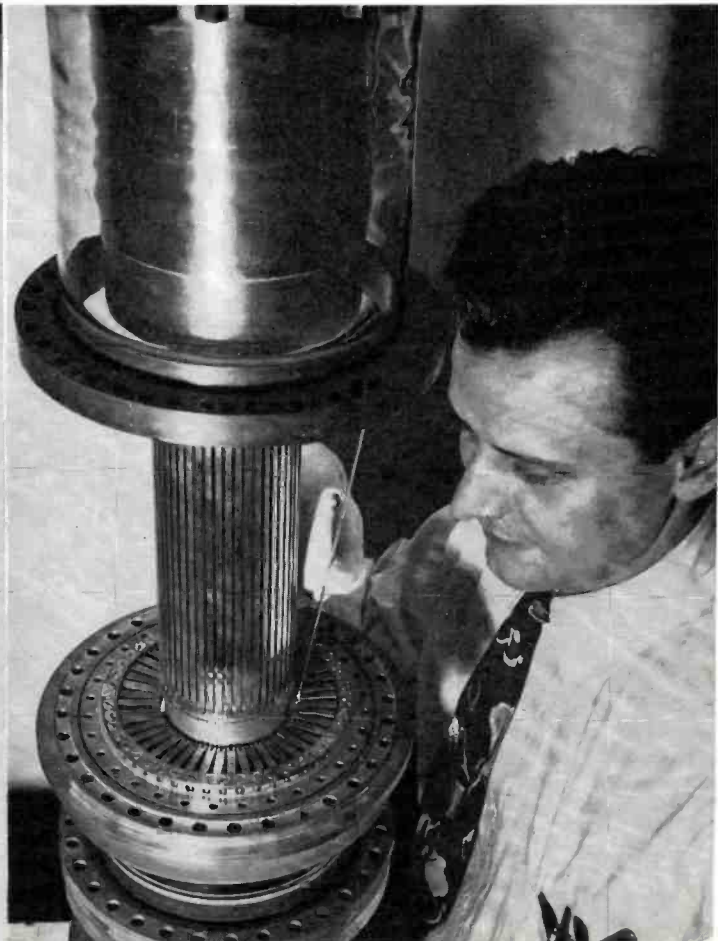
FIG. 3. The individual filament and grid elements of the unit triodes in the array are tungsten rods 8 inches long, supported at both ends by means of knife-edge V-notch arrangements. A pantographic device makes each filament strand and grid rod mechanically independent, and allows vertical movement without disturbing the precise alignments and spacings.
