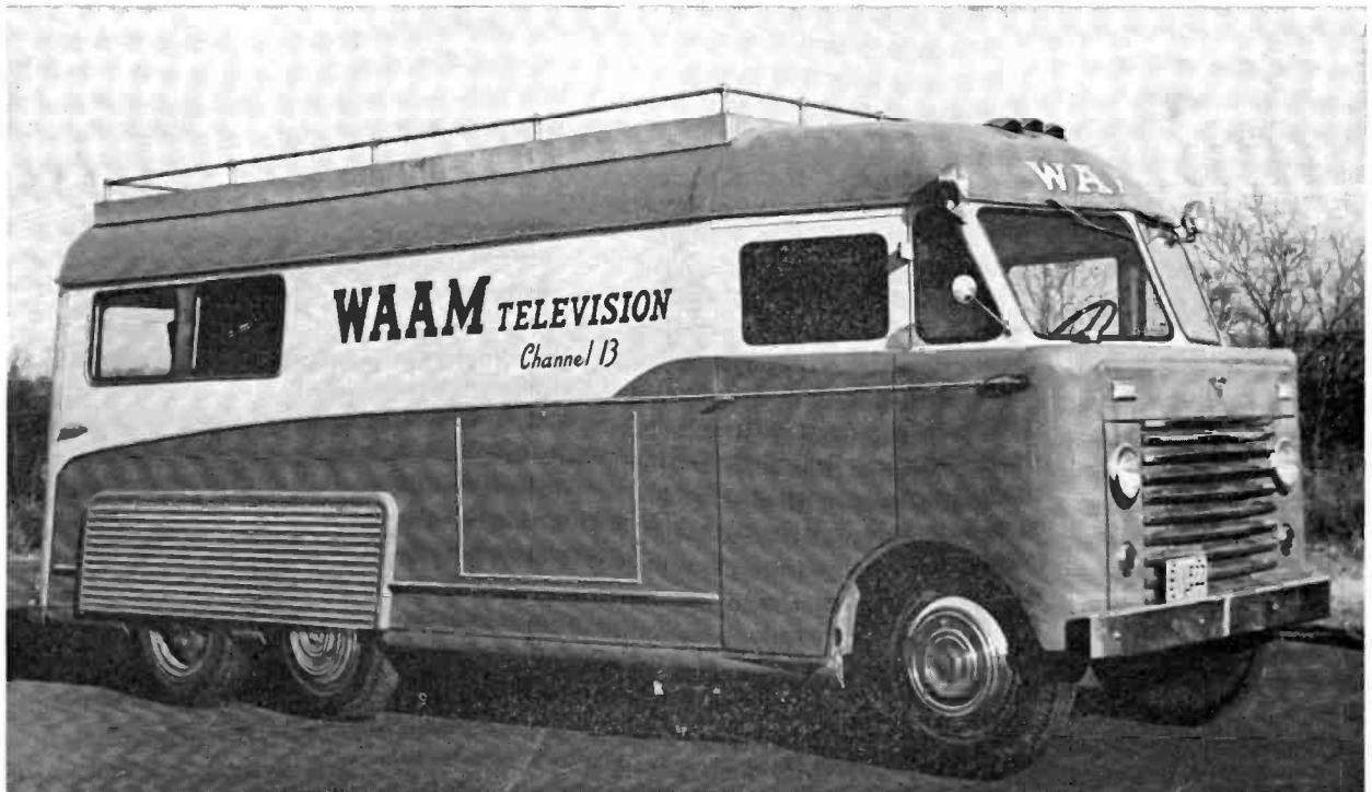
FIG. 11. RCA mobile unit of WAAM provides ample space and storage facilities for field gear used in remote pickups.
