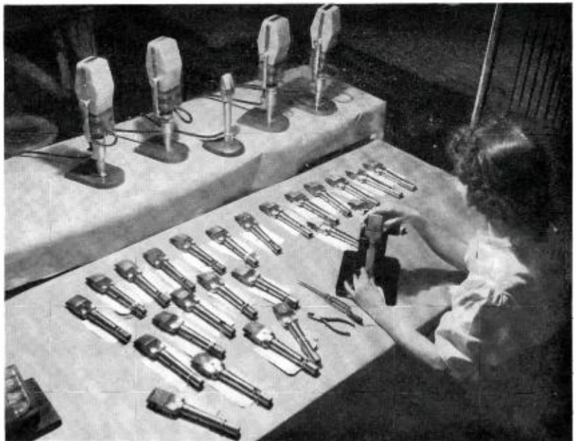
FIG. 2. The KB-2C Bantam Microphone (as shown in this production line photo) is much smaller than the popular Type 44-BX Velocity Microphone.
