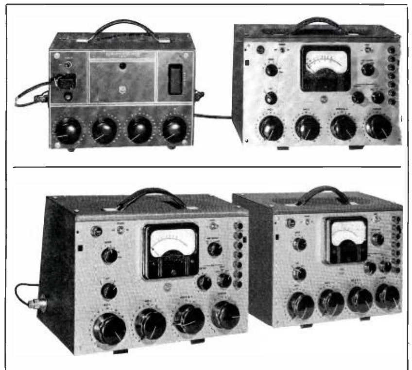
FIG. 3 (bottom). Two BN-2A's in tandem also might be utilized to provide six-channel mixing.
