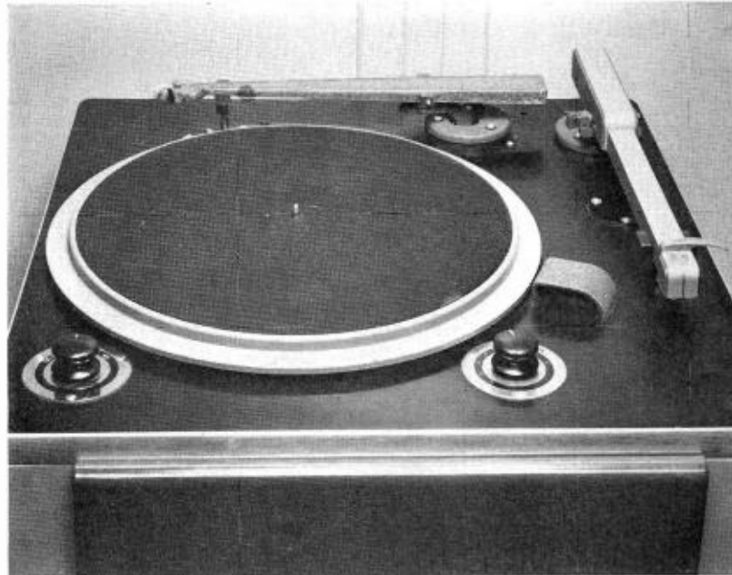
FIG. 1. Closeup of RCA 70-D Turntable with Universal Pickup (at right) and Flat Magnetic Pickup, MI-11874 (at rear) installed.
