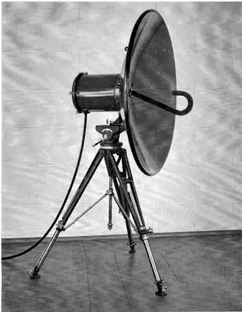
FIG. 15. The RCA Television Relay Transmitter, Type TTR-1B is shown mounted on the new TD-11A all-metal tripod. The Relay Receiver, Type TRR-1B, looks exactly like the unit shown.
