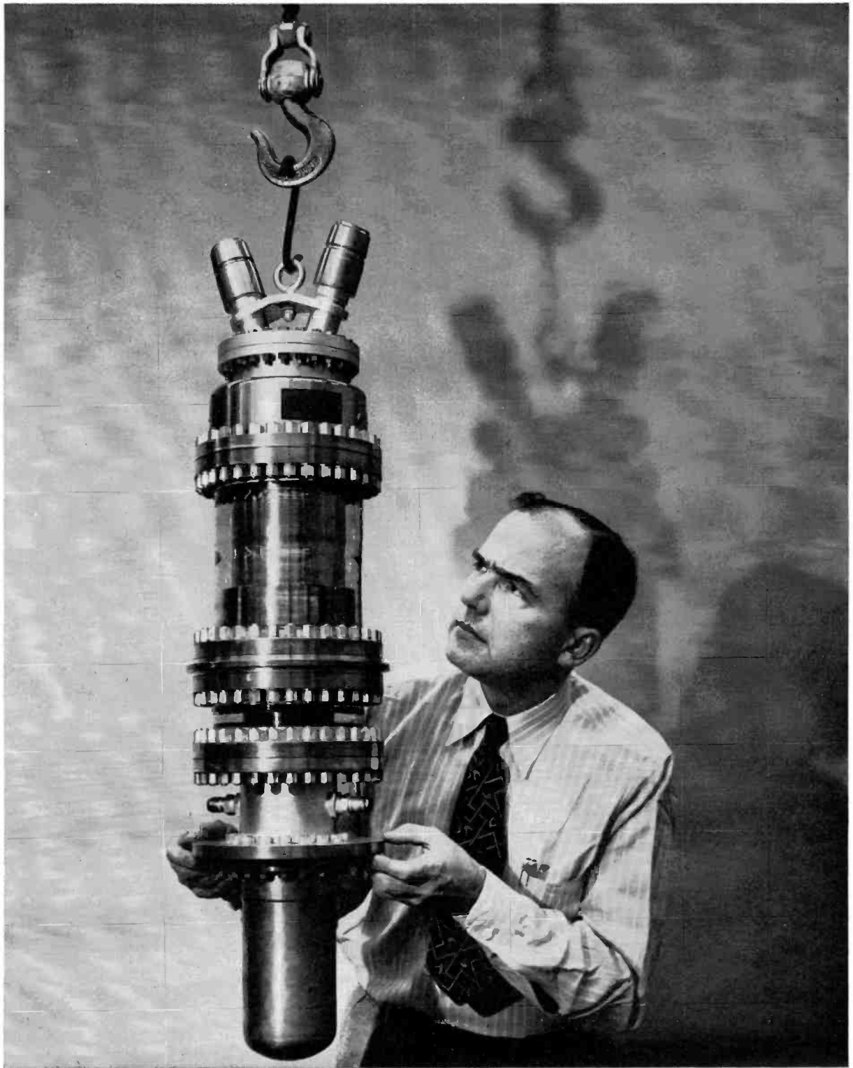
FIG. 1. RCA's new "Super-Power Beam Triode," which is capable of 500 kilowatts output and which has been tested at 1,000,000 watts input, is shown above with Dr. L. P. Garner, head of the Advance Development Lab of the RCA Lancaster, Pa. tube plant, in which the tube was developed. Despite its enormous power output, the new tube is of relatively compact design, weighing only 135 pounds and measuring only 38 \frac{3}{4} inches in length. Present applications of the new tube are in high power CW applications and International Broadcast Service.
