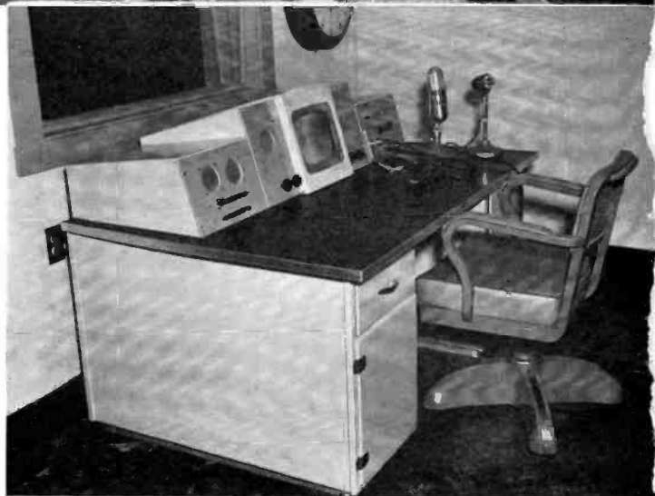
FIG. 9. Master control room above, showing equipment racks and control console. Control equipment, left to right, consists of two film camera controls, preview monitor, and combined line monitor and TS-10A Switching System. Window looks into transmitter room.
