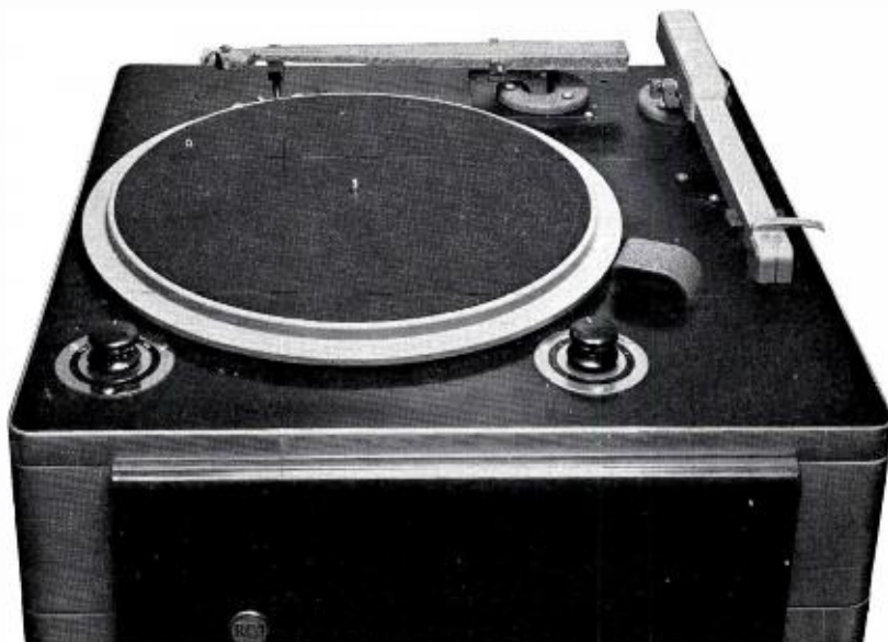
FIG. 18 (below). View of famous RCA 70-D Broadcast Turntable with Lightweight Pickup and Tone Arm at rear. At right is existing arm which may also be used at 33 1/3 and 78, when desired.
