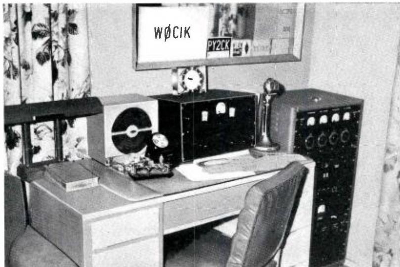
WØCIK Transmitter Room. Present transmitter runs 150 watts to pair of 24-G's.
