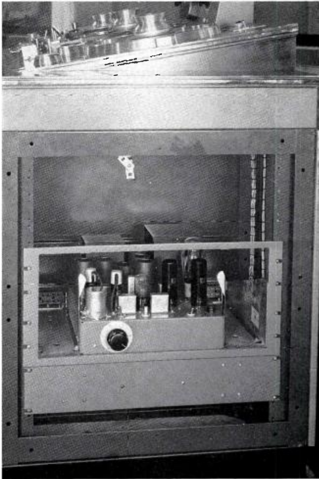
FIG. 4. End view of the Editing Machine illustrating how removable end panels make the amplifier easily accessible.
