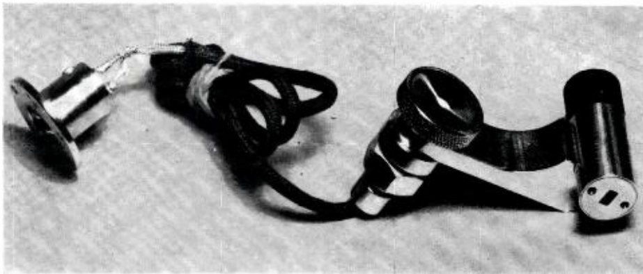
FIG. 2. Closeup view of the photocell scanning unit.
