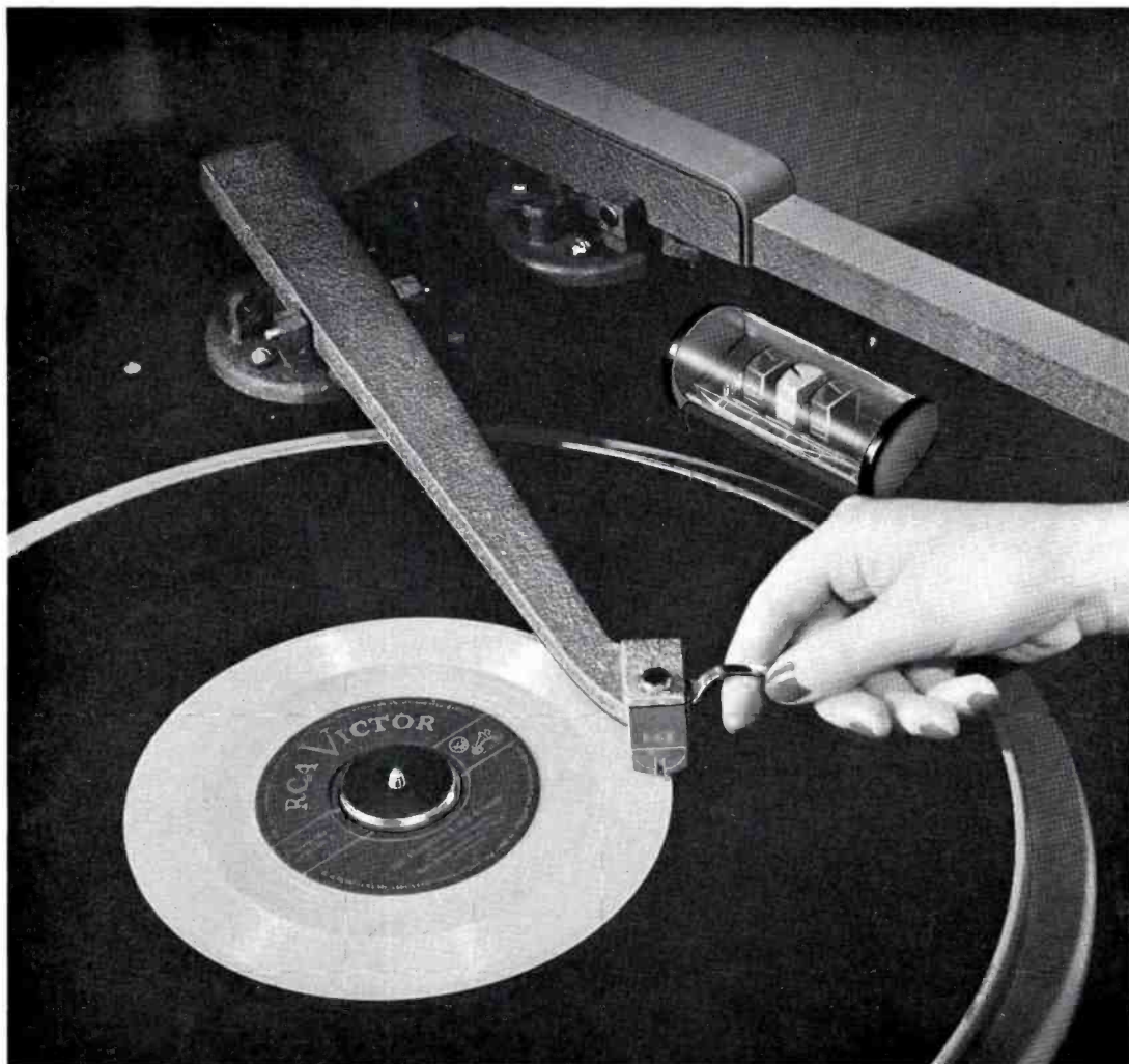
FIG. 1 (at right). The new Lightweight Pickup and Tone Arm combination plays at all speeds and may be applied to existing Broadcast turntables.
