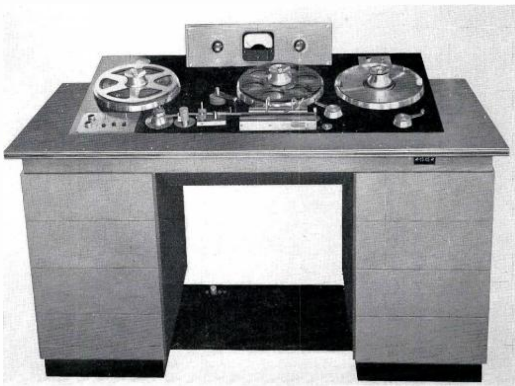
FIG. 3. Photo showing an overall front view of the Console Magnetic Tape Editing Machine. Note foot rest and sequence type foot switch located in the foot ramp.
