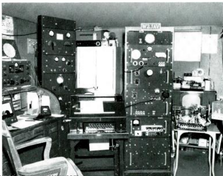
The rack in the center of the W2JAV operating room contains the original teletype gear which has been superseded by the very small unit partially visible at the extreme right. To the left of this is a teletype Model 14 tape printer, and on the left side of the rack is a Model 12 roll printer. The rack in the background is Phil's low-frequency transmitter.
